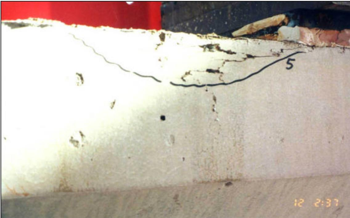
Figure 3.8 Spalling of Concrete Near the Loading Plate
