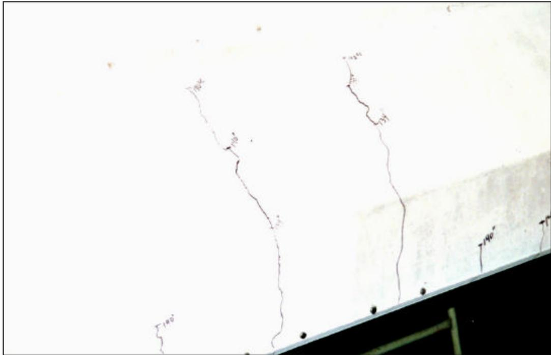
Figure 3.5 Cracks after Static Load 0-C
