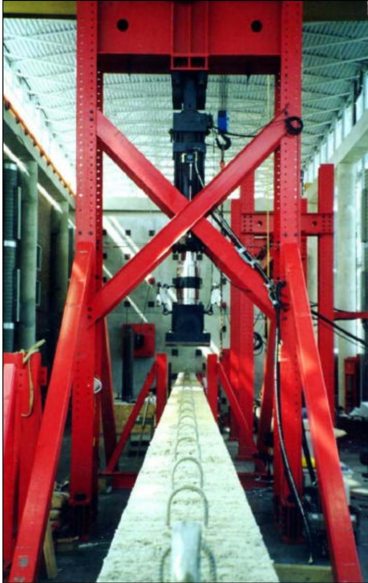
Figure 3.3 Load Frame for Girder Testing
