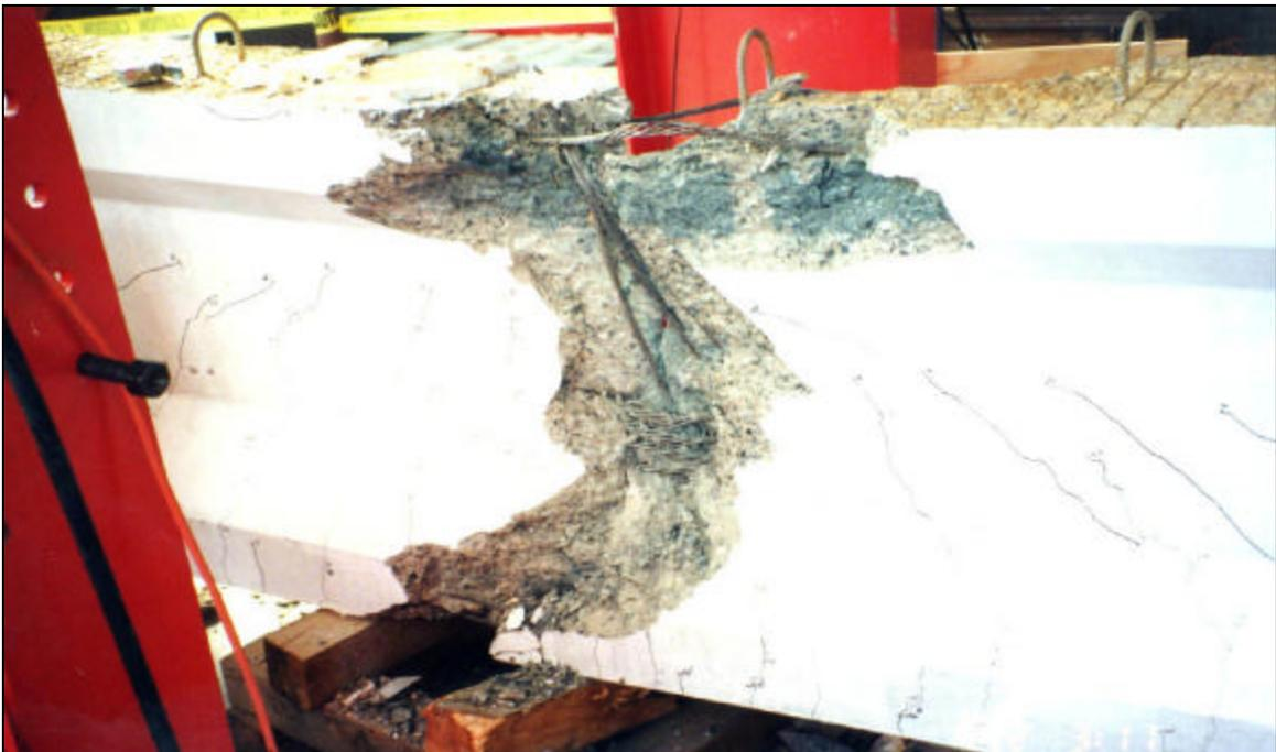
Figure 3.11 AASHTO Type III Girder after Failure
