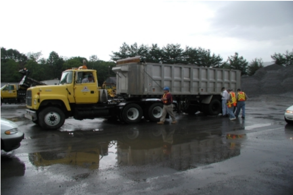
Figure 3.1 Truck used during live load test.
