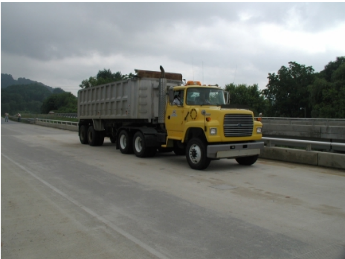
Figure 3.6 Truck on bridge during live load test.
