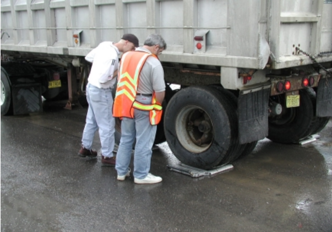
Figure 3.2 Determining wheel loads with scales.
