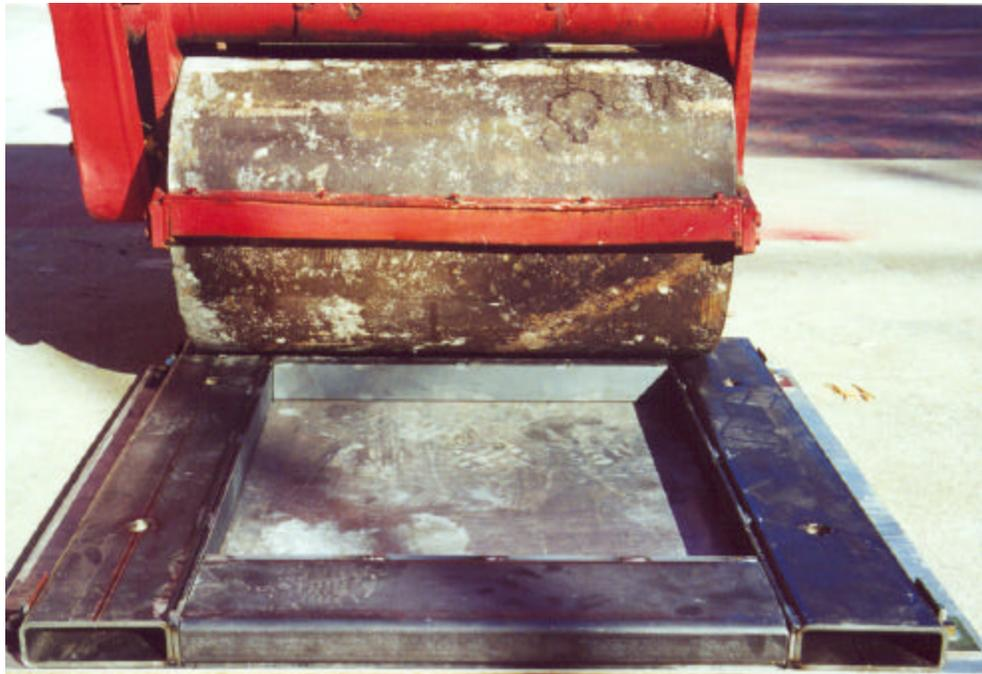
**Figure 6-2 Mold with roller**
