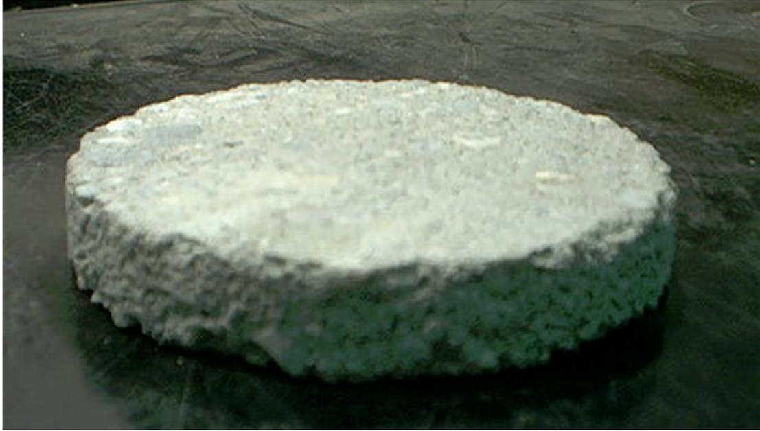
**Figure 6-5 Photo of a 1-inch thick CTB ‘disk’**
