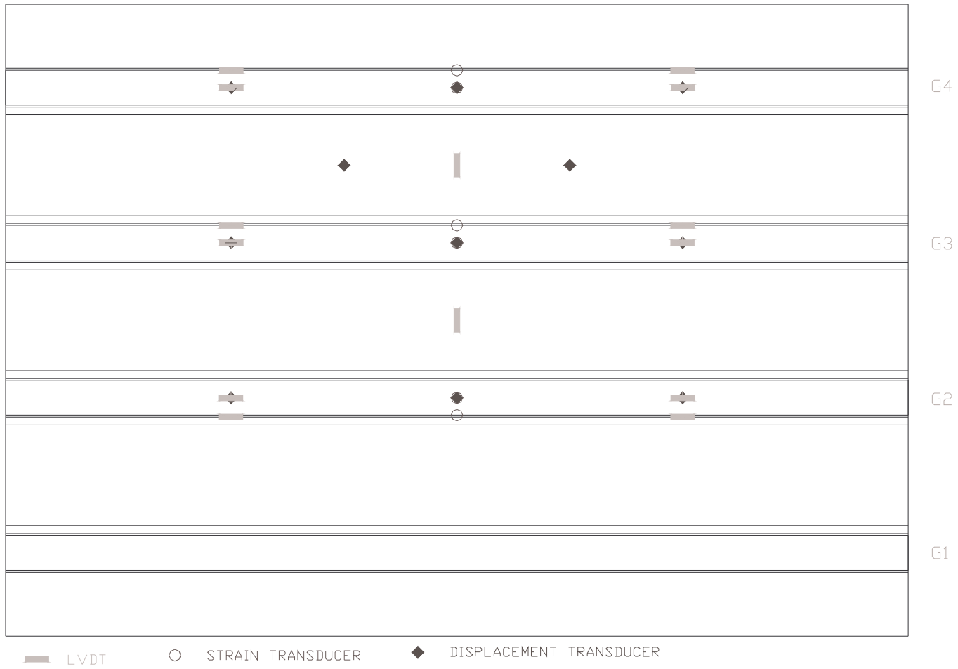
Figure C.17 Instrumentation on Span 1
