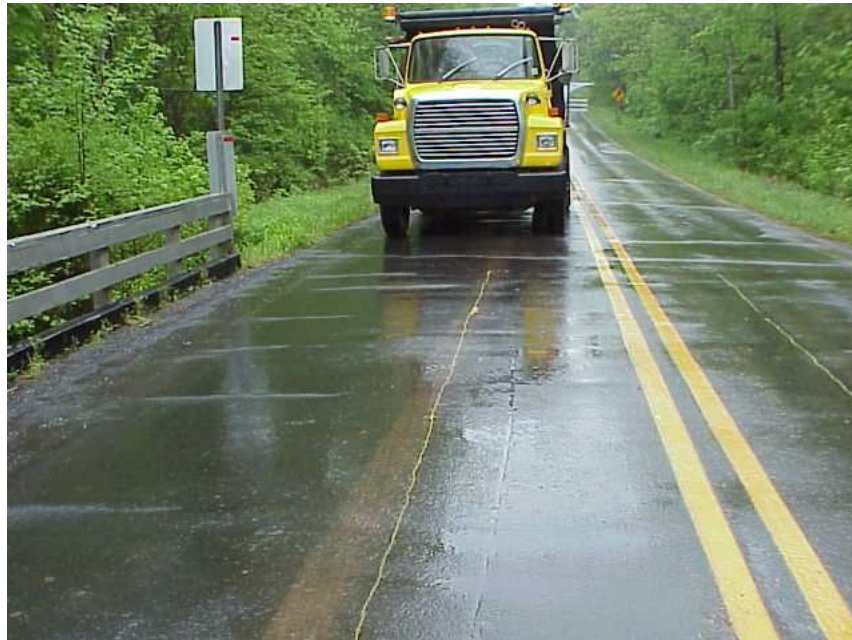
Figure C.10 Tandem truck loading bridge 89-0219
