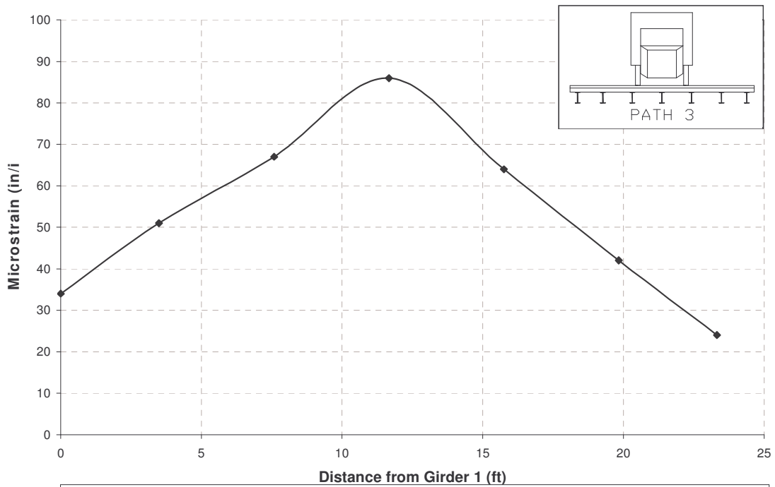
Figure 5.23 Strain distribution at mid-span – static path 3
