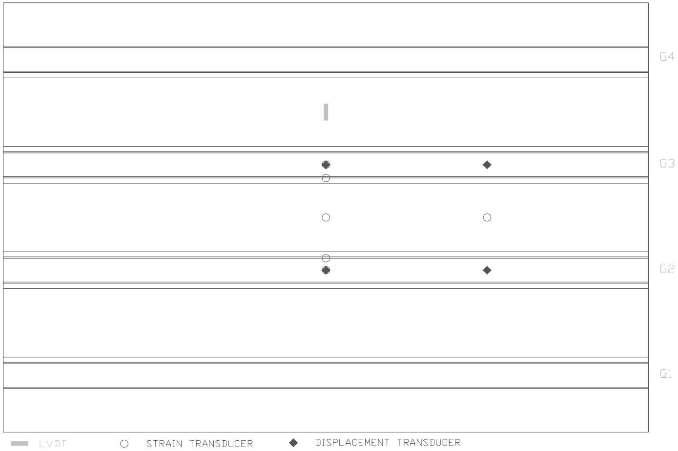
Figure C.18 Instrumentation on Span 2
