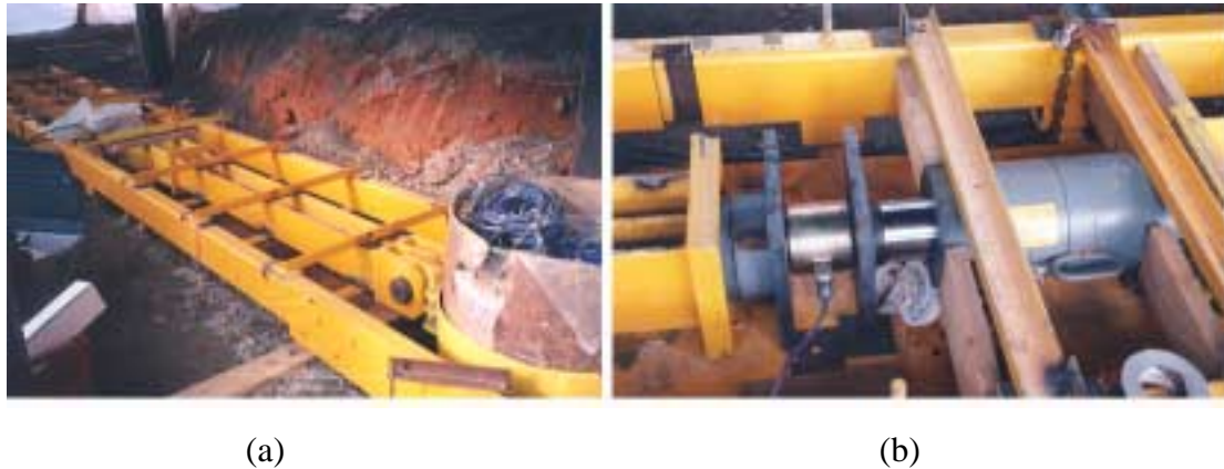
Figure 34. (a) Loading Frame, (b) Installed Loading Jack and Load Cell
