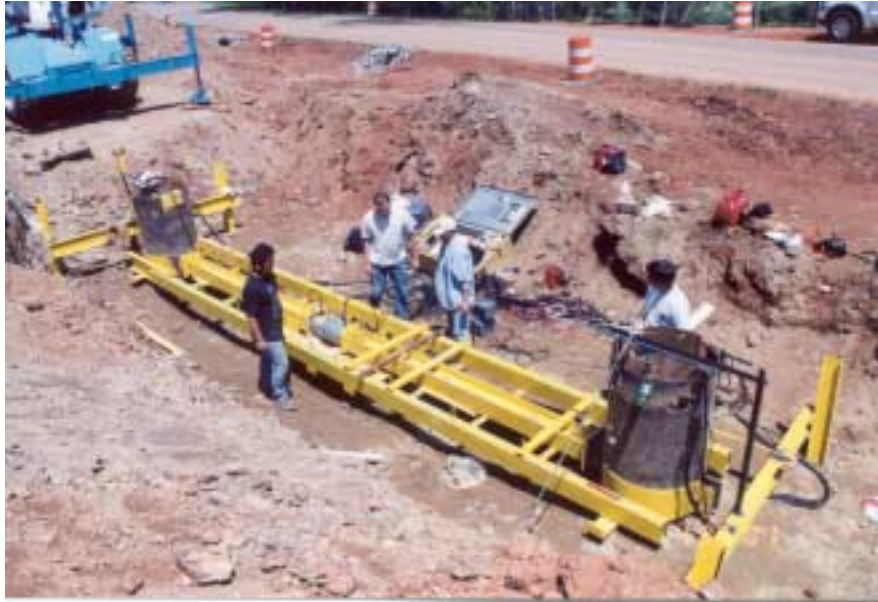
Figure 43. Load Test Frame and Instrumentation Set-up Profile
