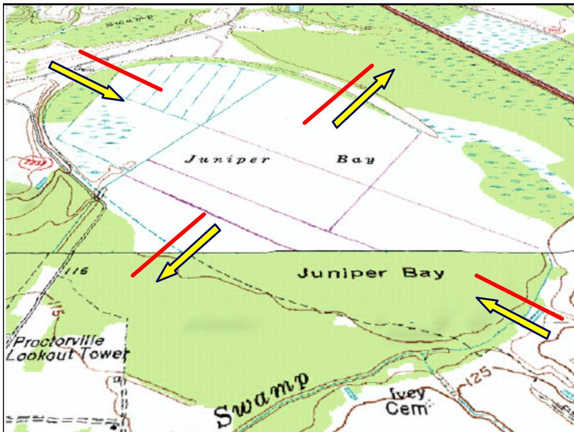
Figure 3.1 Perspective view of Juniper Bay topography. Arrows indicate the expected directions of subsurface flux.
