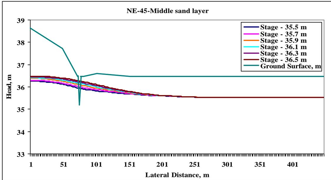
Figure 5.10 Spatial distribution of heads in middle sand layer at the NE transect for different ditch control levels on 15 February 2004.
