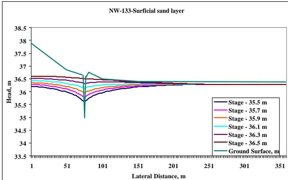
Figure 5.2 Spatial distribution of heads in surficial sand layer at the NW transect for different ditch control levels on 13 May 2004.
