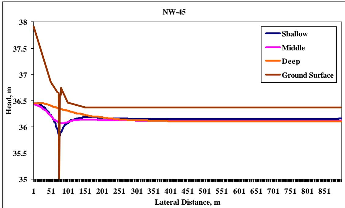
Figure 4.15 Heads in the three conducting layers at the NW transect on 15 February 2004.
