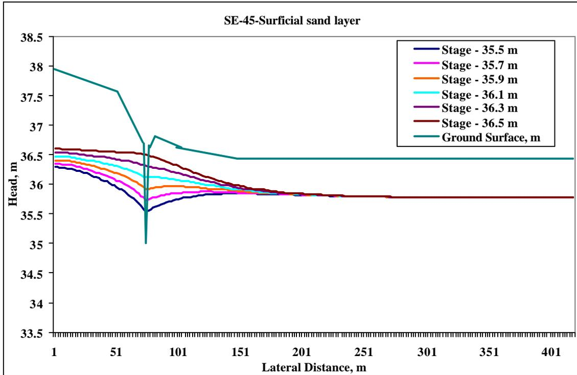
Figure 5.15 Spatial distribution of heads in surficial sand layer at the SE transect for different ditch control levels on 15 February 2004.
