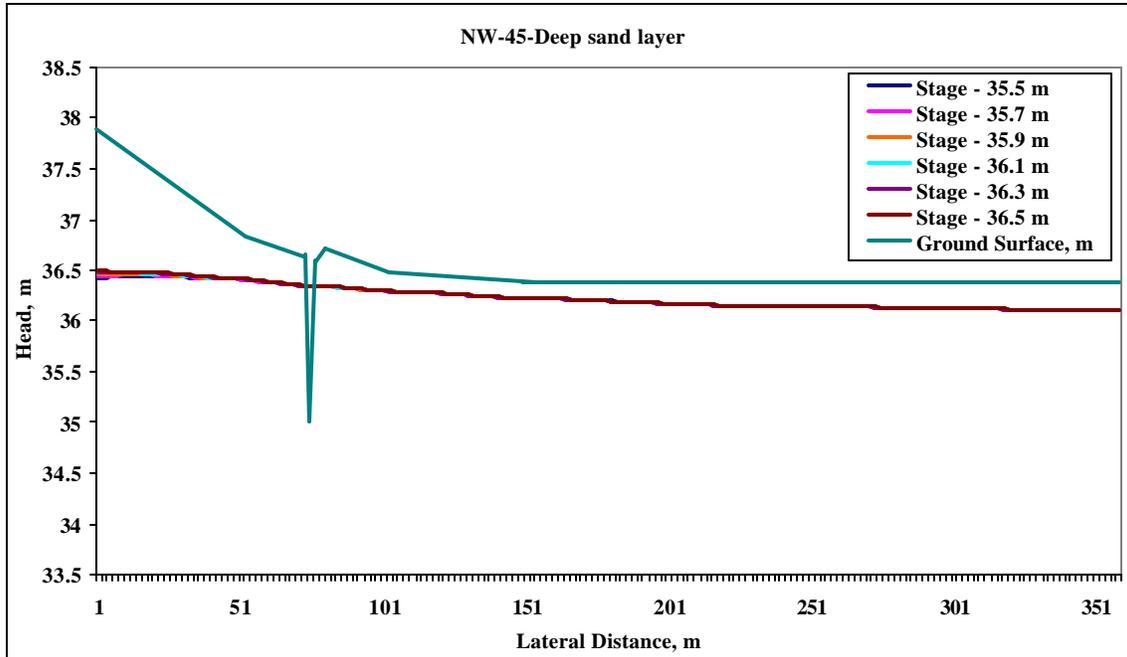
Figure 5.5 Spatial distribution of heads in deep sand layer at the NW transect for different ditch control levels on 15 February 2004.
