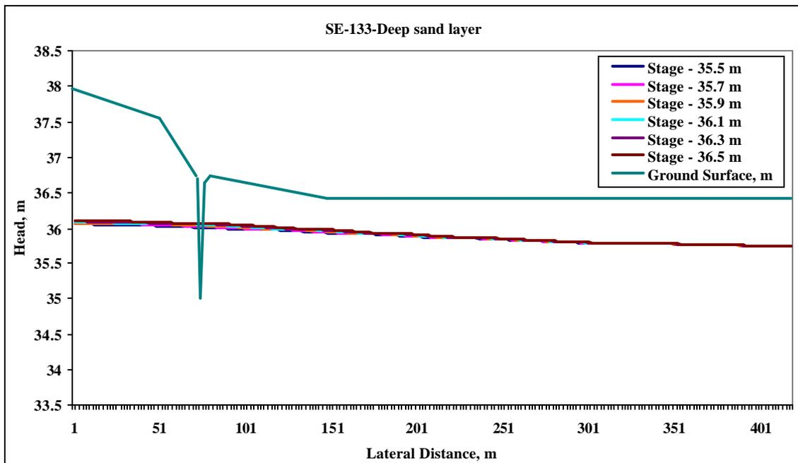
Figure 5.20 Spatial distribution of heads in deep sand layer at the SE transect for different ditch control levels on 13 May 2004.
