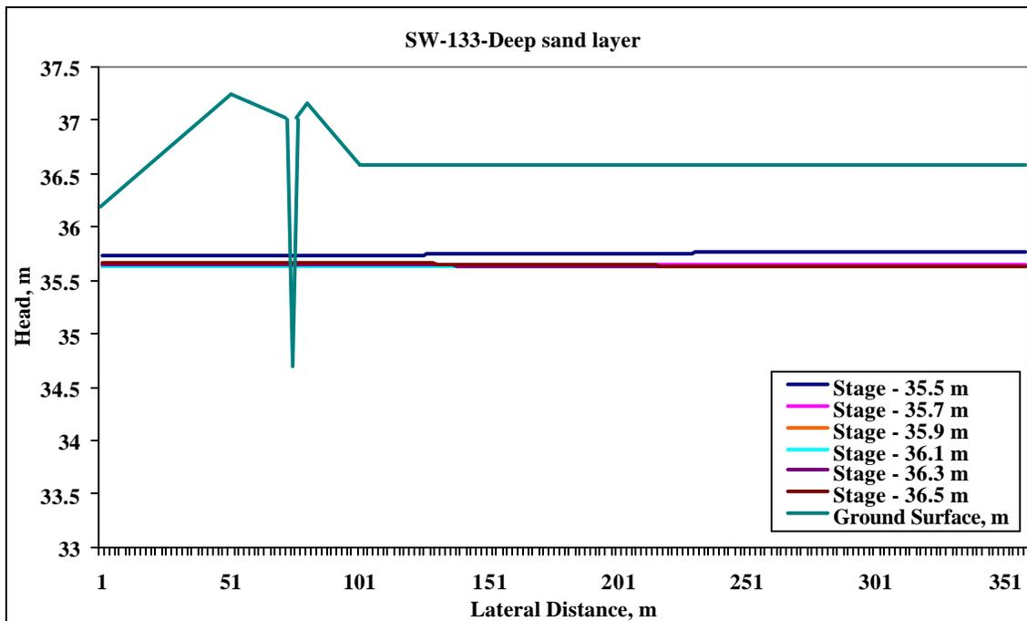
Figure 5.27 Spatial distribution of heads in deep sand layer at the SW transect for different ditch control levels on 13 May 2004.
