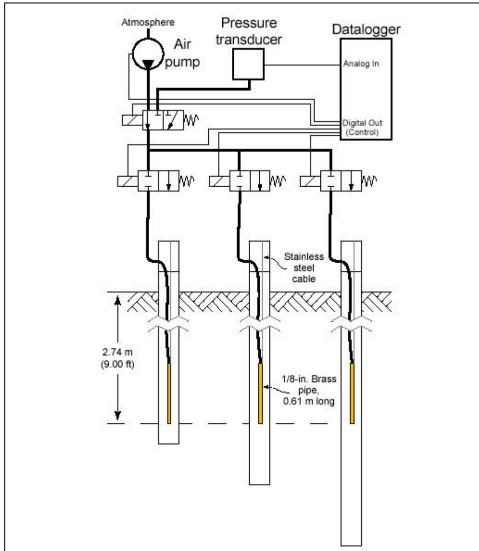
Figure 3.11 Schematic diagram of a monitoring unit assembly
