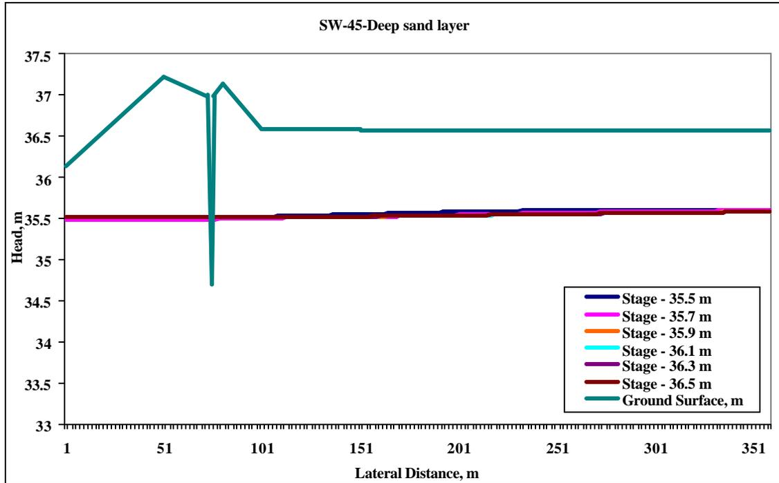
Figure 5.26 Spatial distribution of heads in deep sand layer at the SW transect for different ditch control levels on 15 February 2004.
