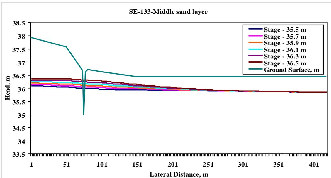
Figure 5.18 Spatial distribution of heads in middle sand layer at the SE transect for different ditch control levels on 13 May 2004.
