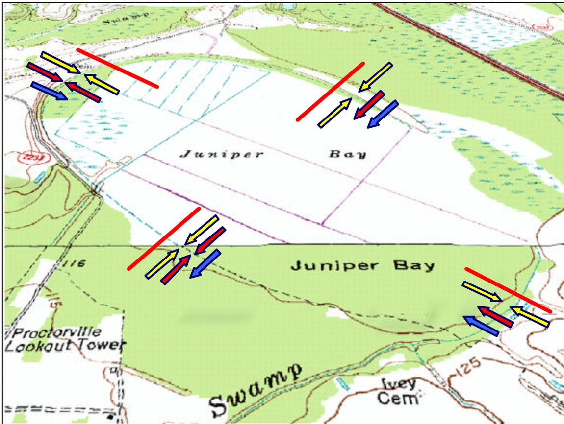
Figure 4.38 Summary of flow directions in significant sand layers. Light (yellow) arrows are for the surficial sand layers, medium (red) arrows are for the middle sand layers, and dark (blue) arrows are for the deep sand layers.
