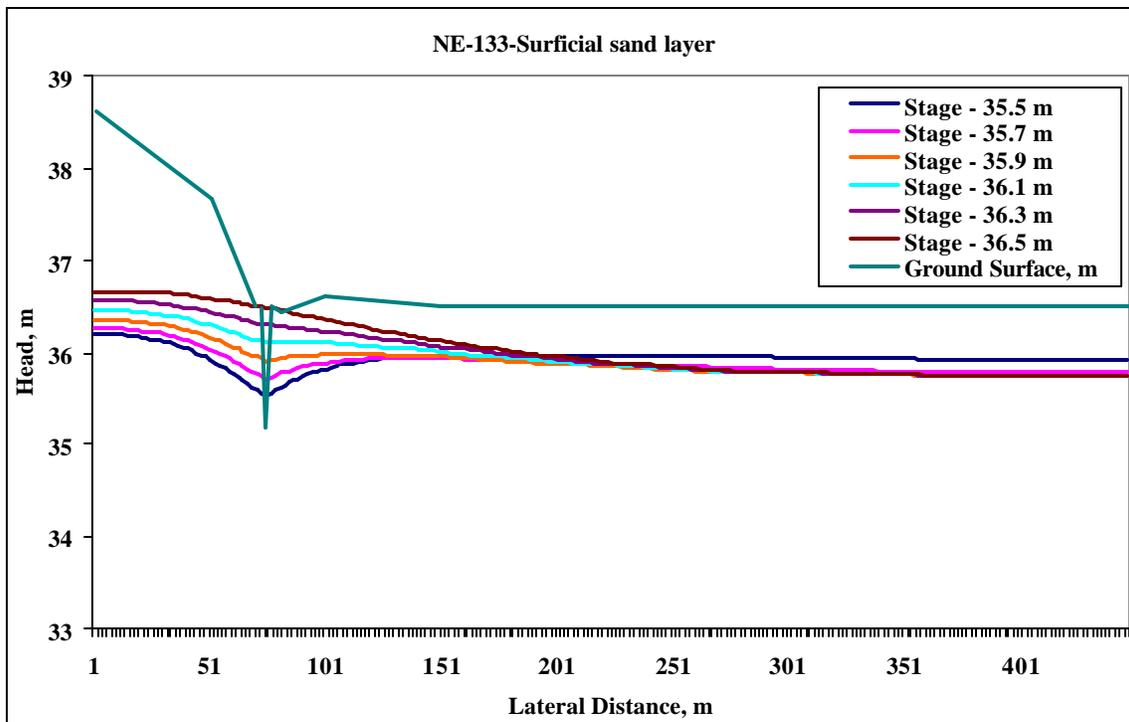
Figure 5.9 Spatial distribution of heads in surficial sand layer at the NE transect for different ditch control levels on 13 May 2004.
