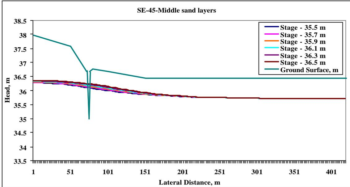
Figure 5.17 Spatial distribution of heads in middle sand layer at the SE transect for different ditch control levels on 15 February 2004.
