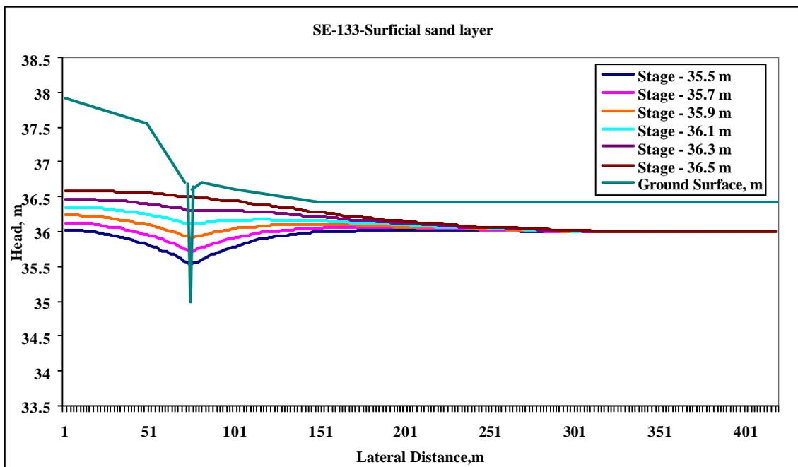
Figure 5.16 Spatial distribution of heads in surficial sand layer at the SE transect for different ditch control levels on 13 May 2004.
