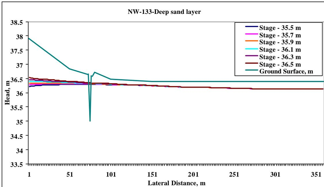
Figure 5.6 Spatial distribution of heads in deep sand layer at the NW transect for different ditch control levels on 13 May 2004.
