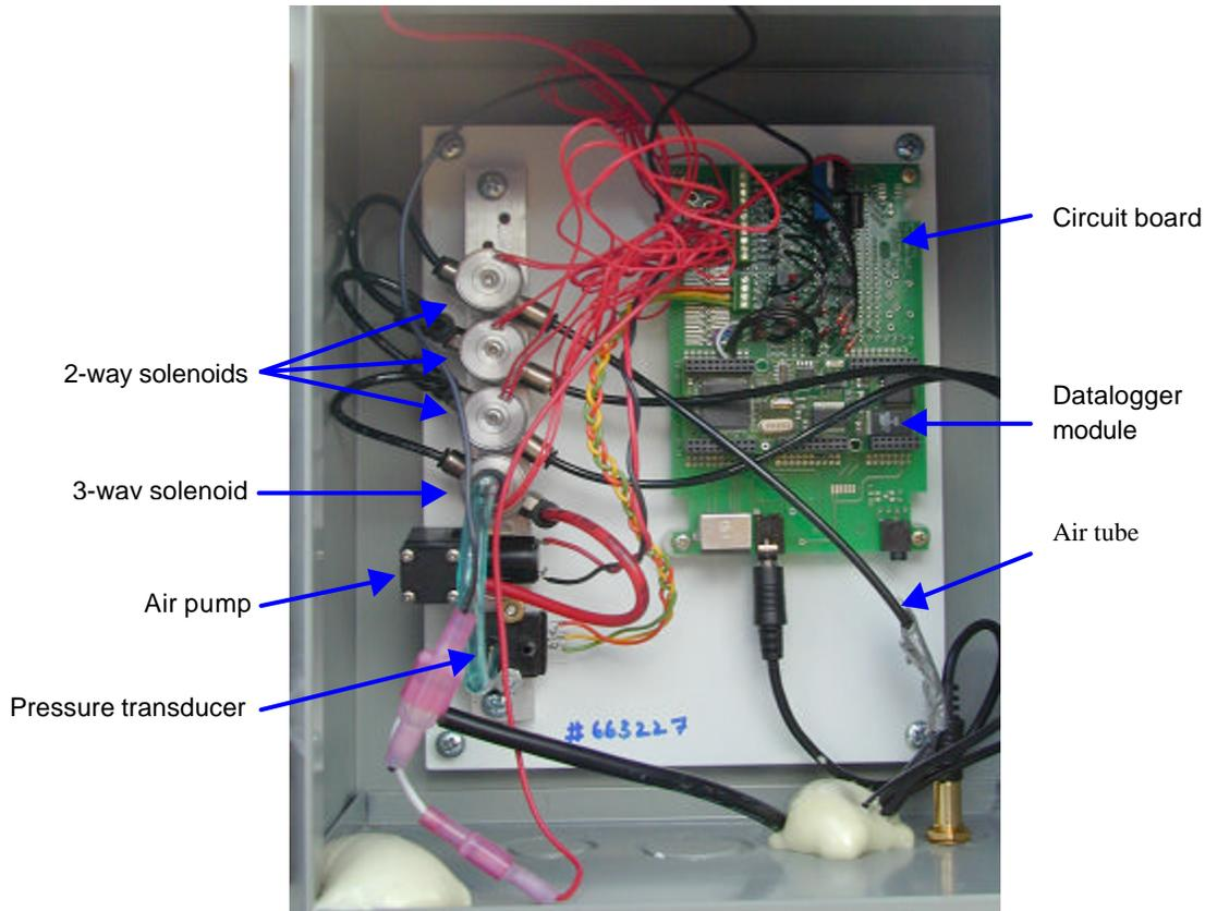
Figure 3.12 Monitoring unit in its enclosure.
