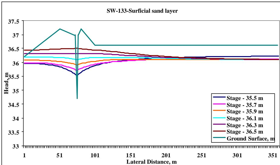
Figure 5.23 Spatial distribution of heads in surficial sand layer at the SW transect for different ditch control levels on 13 May 2004.
