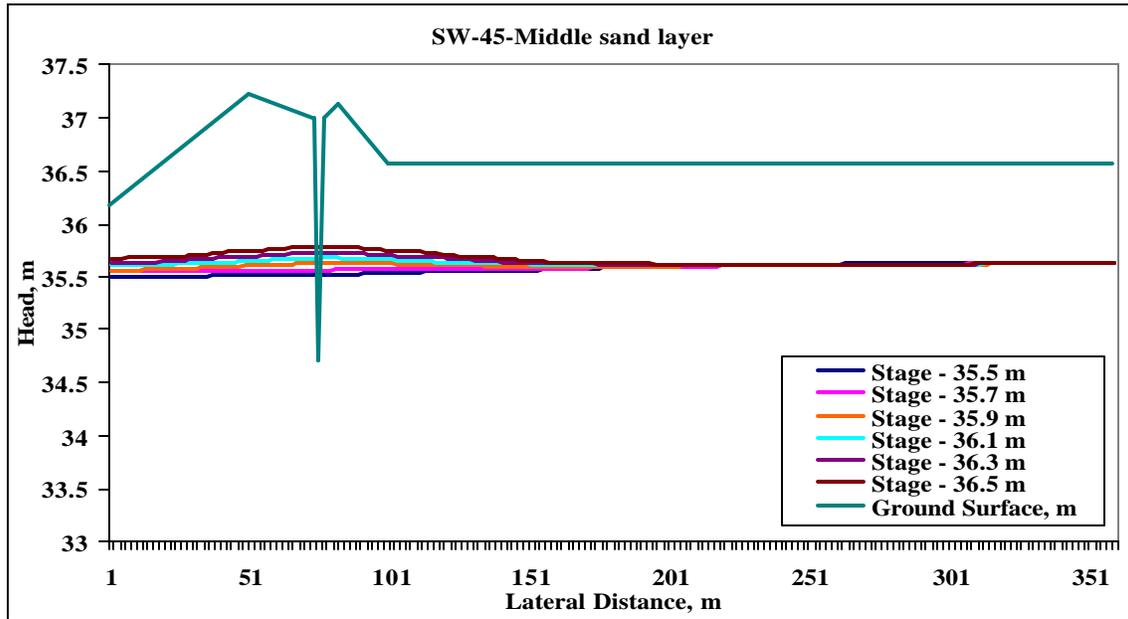
Figure 5.24 Spatial distribution of heads in middle sand layer at the SW transect for different ditch control levels on 15 February 2004.
