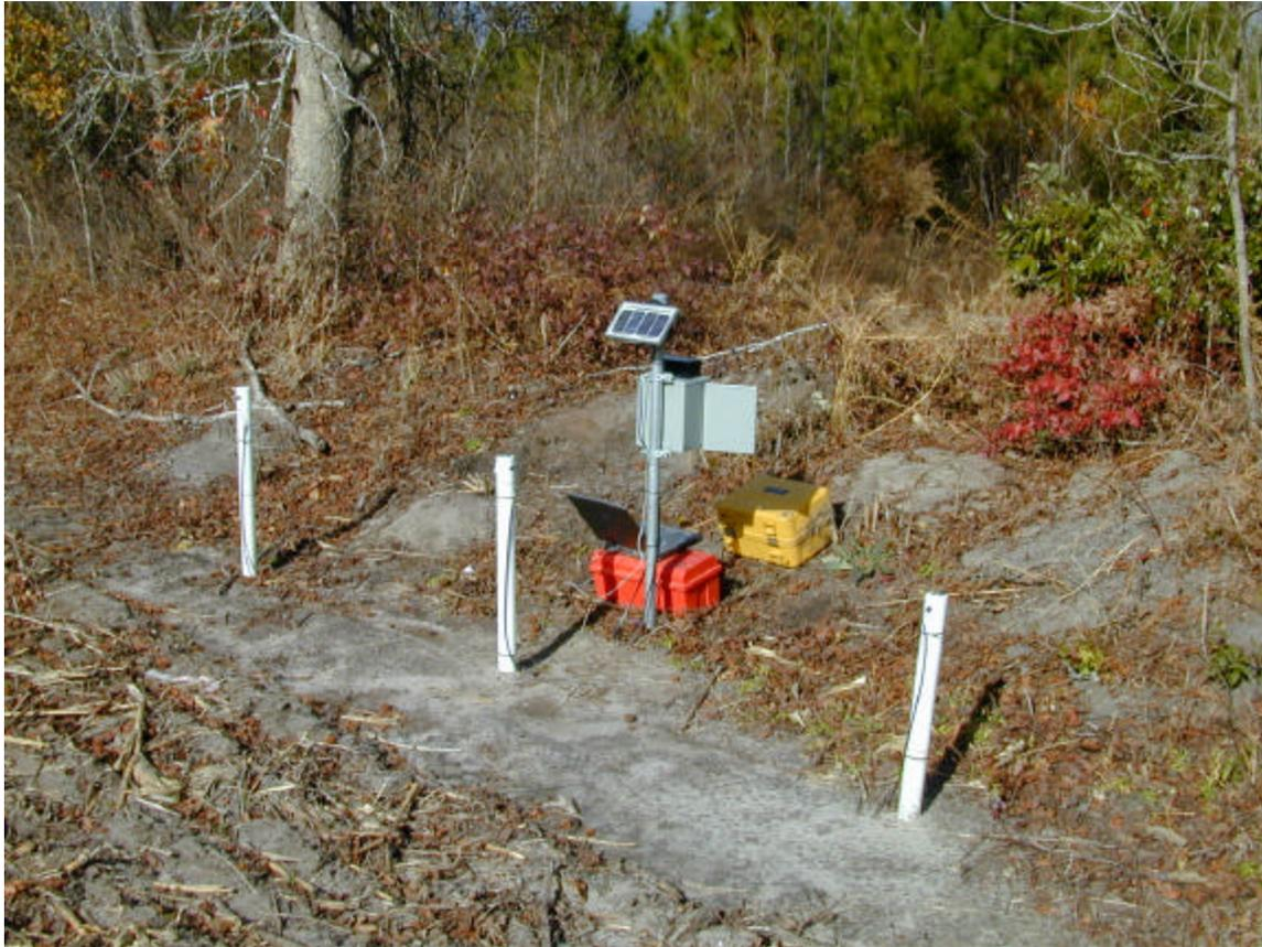
Figure 3.10 Nest of three piezometers with water level monitoring system.
