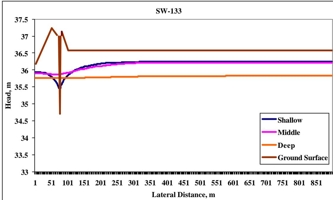
Figure 4.35 Heads in the three conducting layers at the SW transect corresponding to dry period (13 May 2004).
