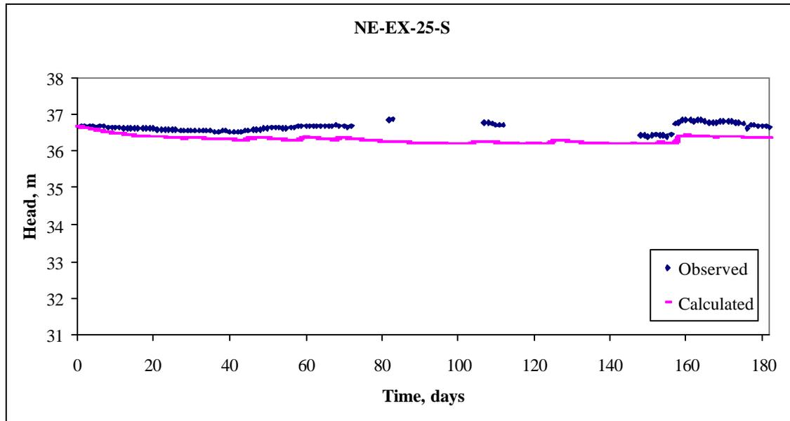
Figure 4.19 Calibration plot example (at exterior 25 m piezometer nest) at the NE transect.
