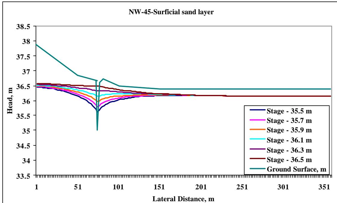
Figure 5.1 Spatial distribution of heads in surficial sand layer at the NW transect for different ditch control levels on 15 February 2004.
