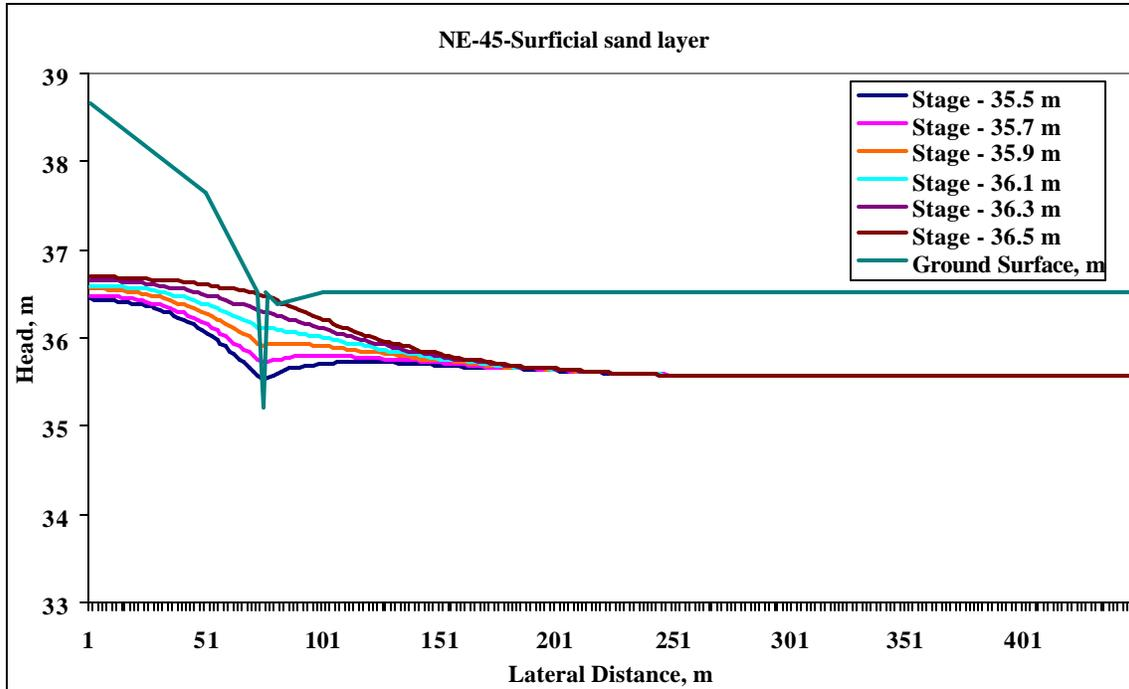
Figure 5.8 Spatial distribution of heads in surficial sand layer at the NE transect for different ditch control levels on 15 February 2004.
