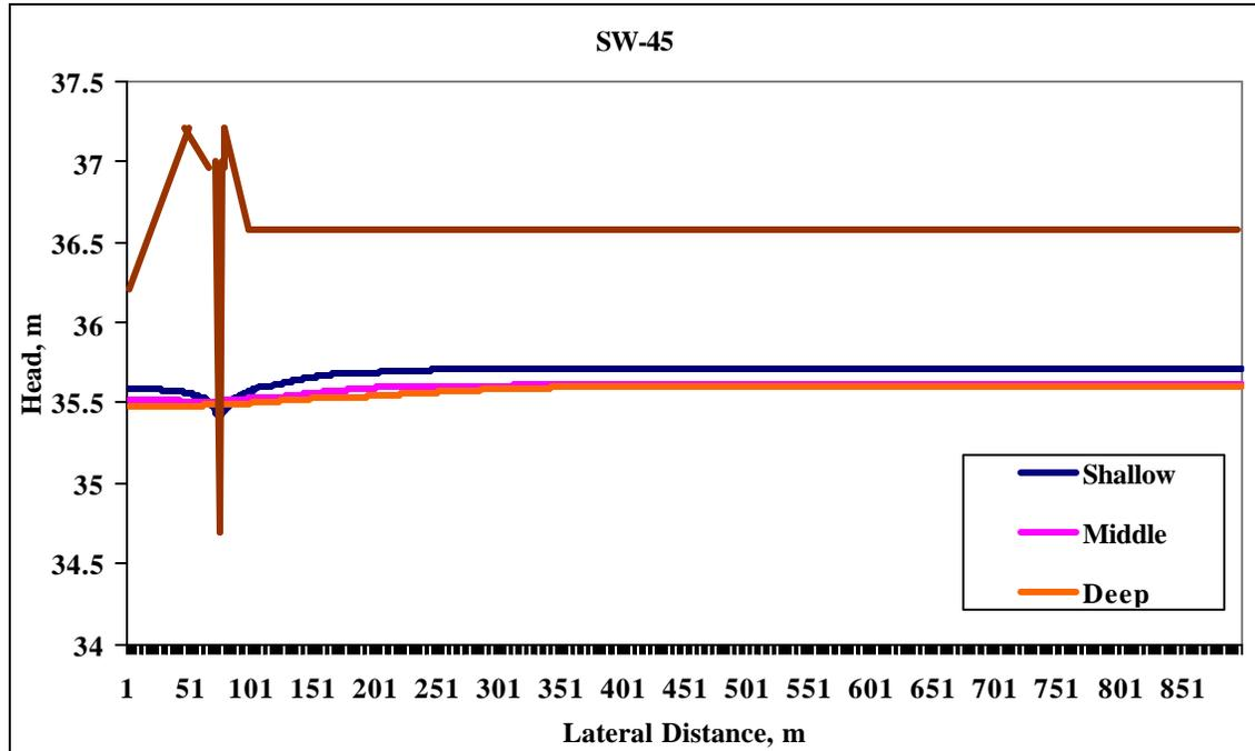
Figure 4.33 Heads in the three conducting layers at the SW transect corresponding to dry period (15 February 2004).
