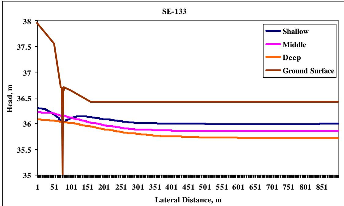
Figure 4.29 Heads in the three conducting layers at the SE transect on 13 May 2004.
