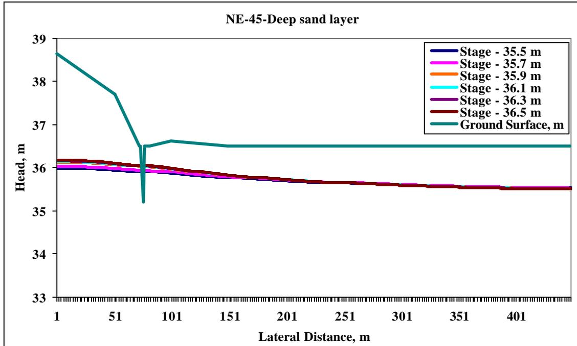
Figure 5.12 Spatial distribution of heads in deep sand layer at the NE transect for different ditch control levels on 15 February 2004.
