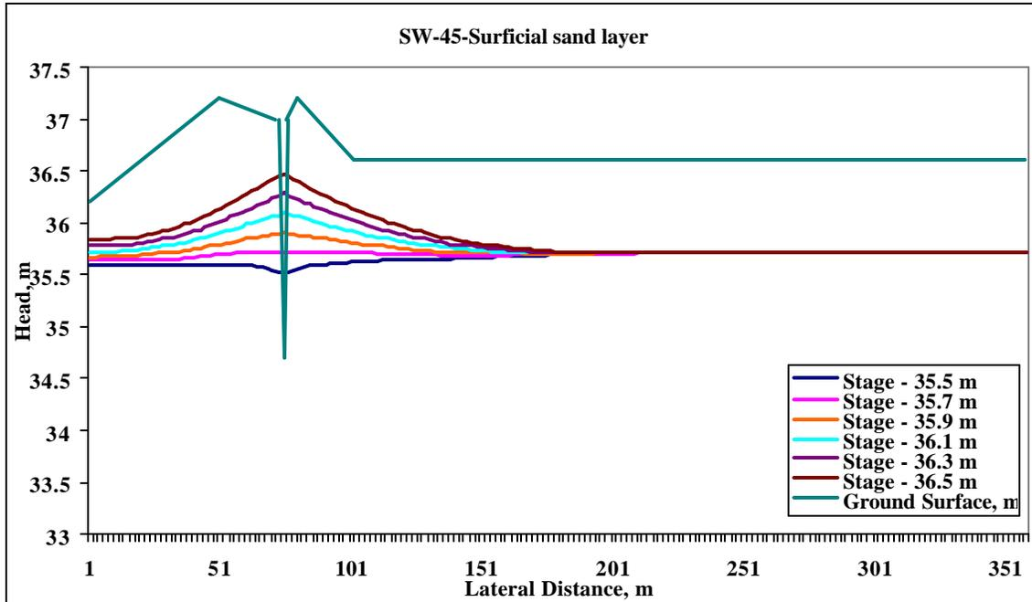
Figure 5.22 Spatial distribution of heads in surficial sand layer at the SW transect for different ditch control levels on 15 February 2004.
