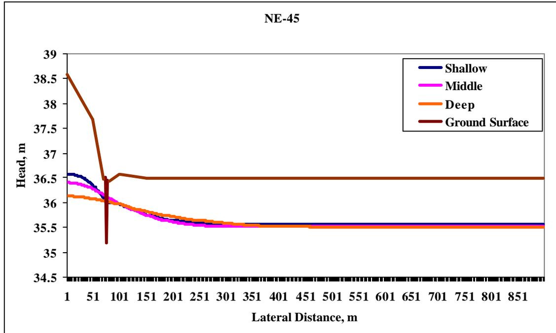
Figure 4.21 Heads in the three conducting layers at the NE transect on 15 February 2004.
