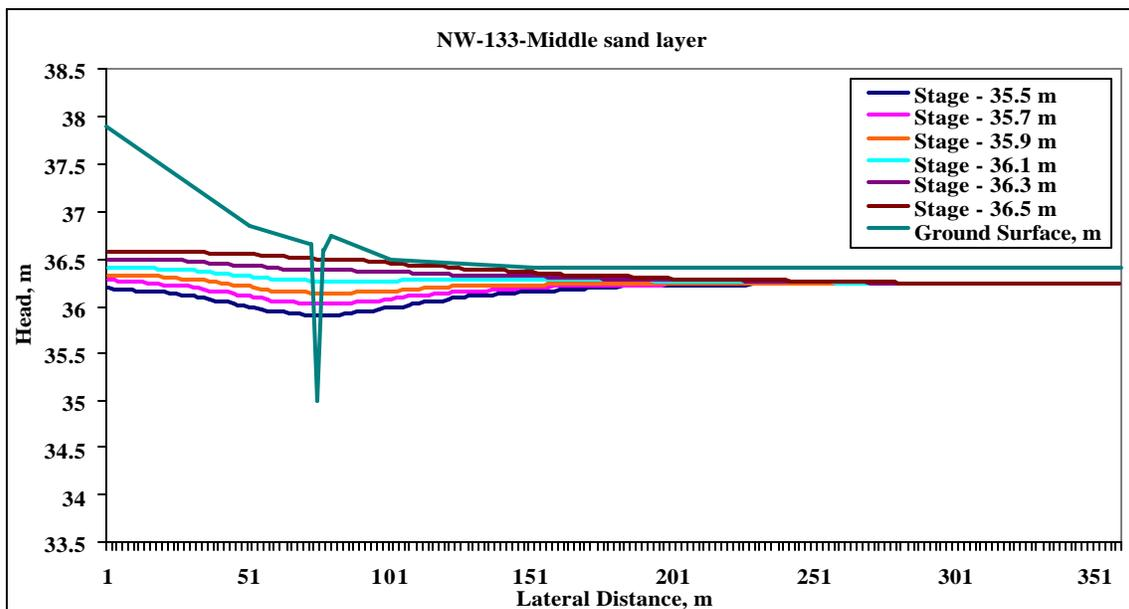
Figure 5.4 Spatial distribution of heads in middle sand layer at the NW transect for different ditch control levels on 13 May 2004.
