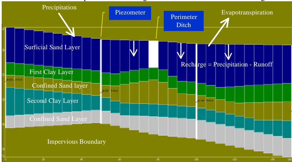
Figure 4.1 Model setup for the NW transect.
