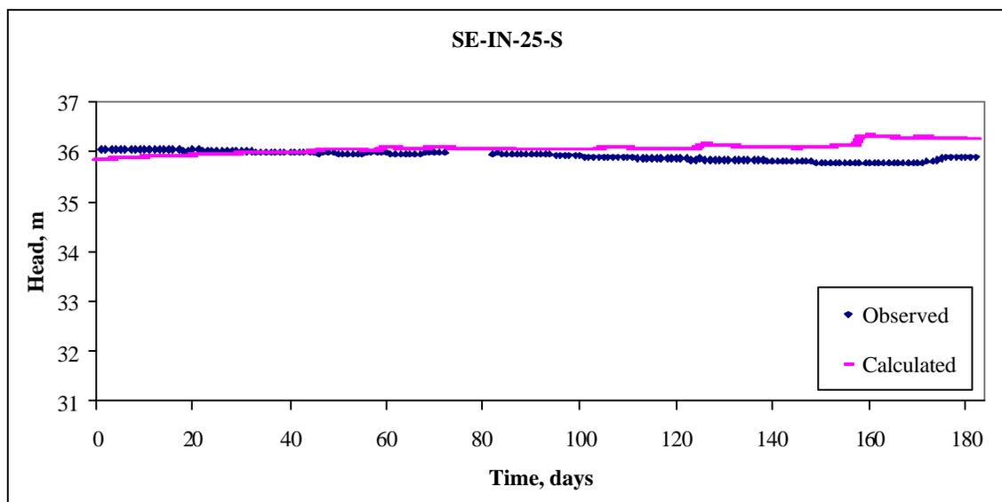
Figure 4.25 Calibration plot example (at interior 25m piezometer nest) at the SE transect.
