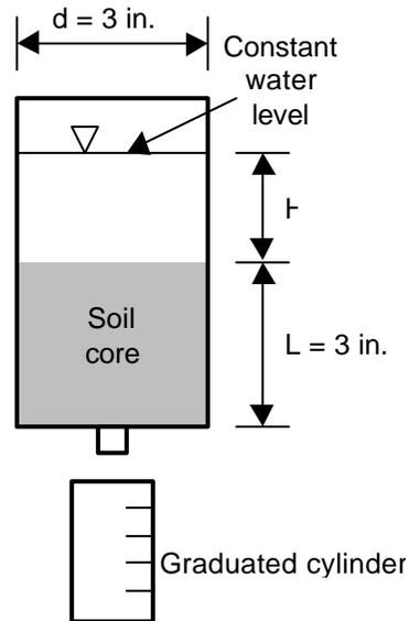
Figure 3.9 Schematic of  $K_{sat}$  apparatus.
