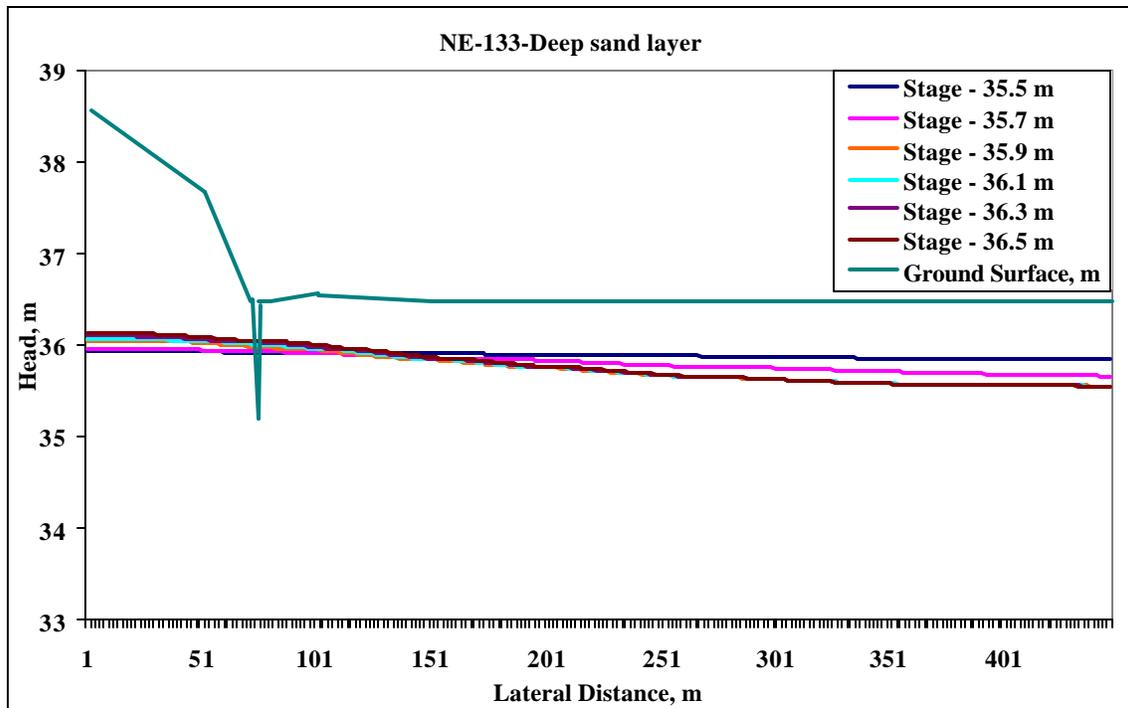
Figure 5.13 Spatial distribution of heads in deep sand layer at the NE transect for different ditch control levels on 13 May 2004.
