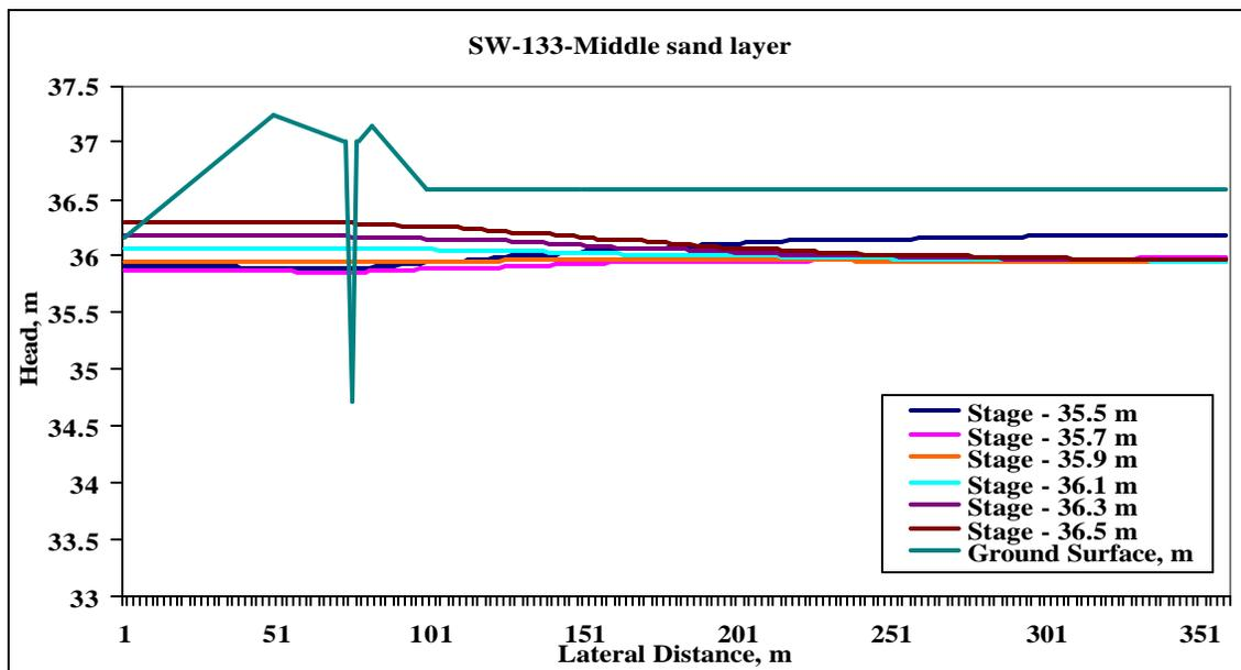
Figure 5.25 Spatial distribution of heads in middle sand layer at the SW transect for different ditch control levels on 13 May 2004.
