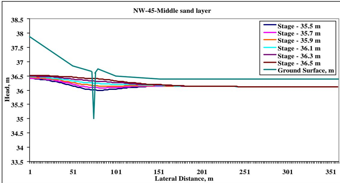
Figure 5.3 Spatial distribution of heads in middle sand layer at the NW transect for different ditch control levels on 15 February 2004.
