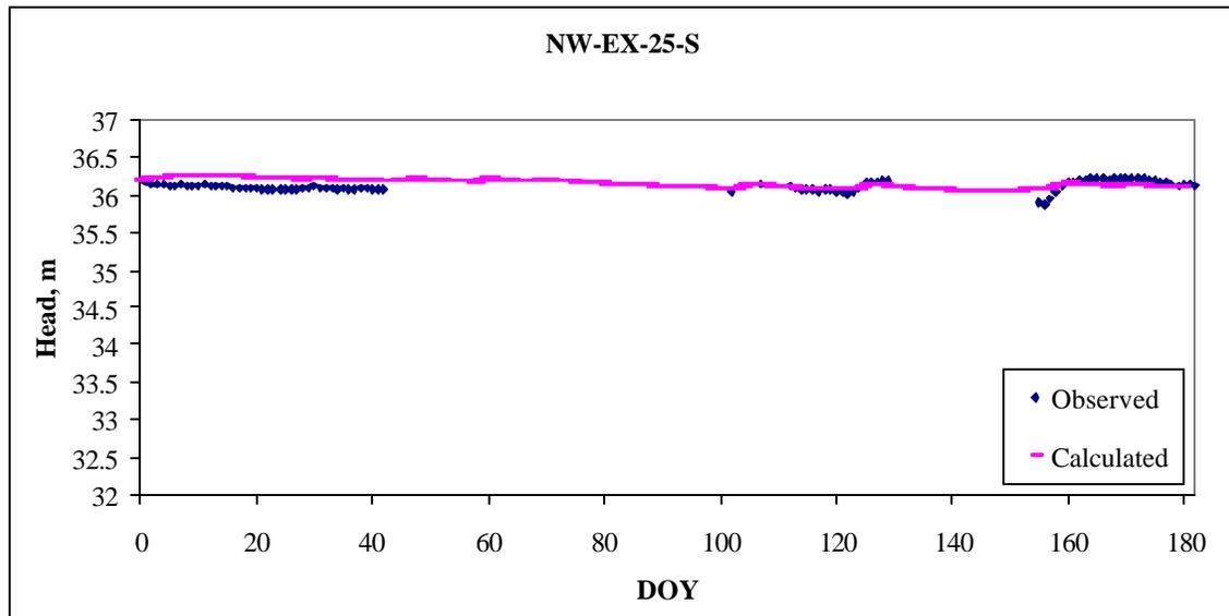
Figure 4.13 Calibration plot example (at exterior 25 m piezometer nest) at the NW transect.
