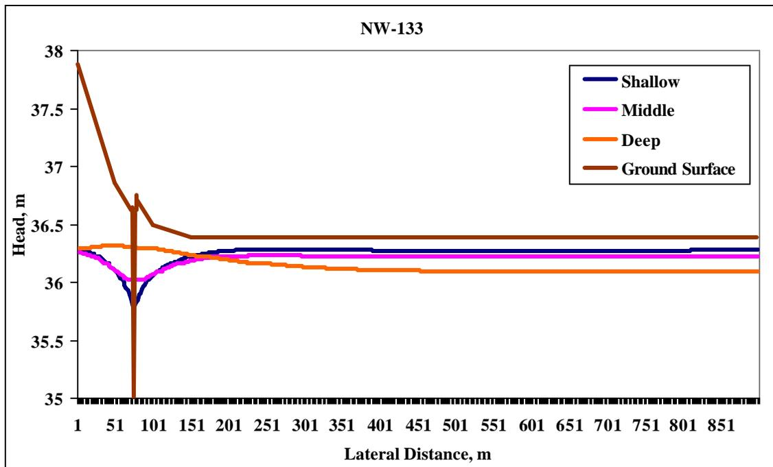
Figure 4.17 Heads in the three conducting layers at the NW on 13 May 2004.
