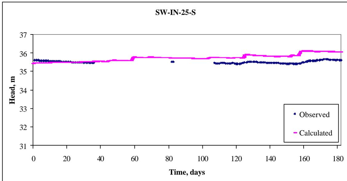
Figure 4.31 Calibration plot example (at interior 25m piezometer nest) at the SW transect.
