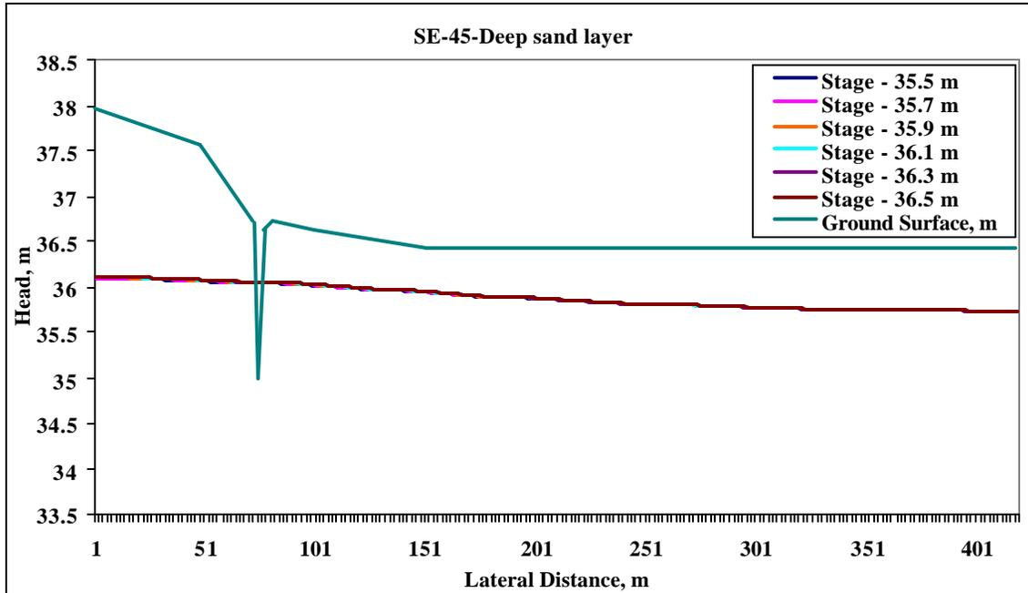
Figure 5.19 Spatial distribution of heads in deep sand layer at the SE transect for different ditch control levels on 15 February 2004.
