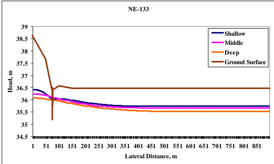
Figure 4.23 Heads in the three conducting layers at the NE transect on 13 May 2004
