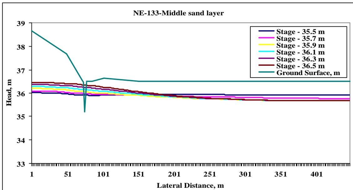
Figure 5.11 Spatial distribution of heads in middle sand layer at the NE transect for different ditch control levels on 13 May 2004.
