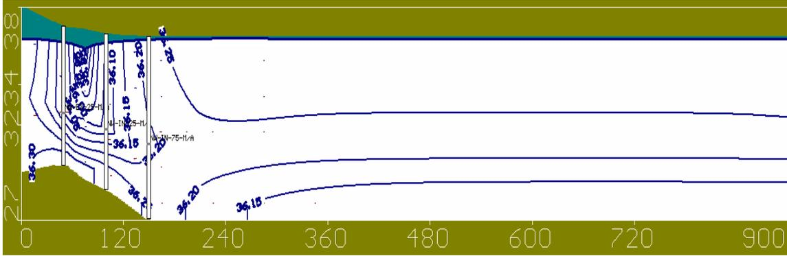
Figure 4.16 Equipotential Lines on 13 May 2004 at the NW transect extended model.
