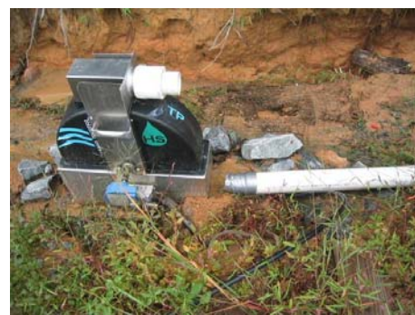
Figure 2.33. Liquid PAM dosing system.
