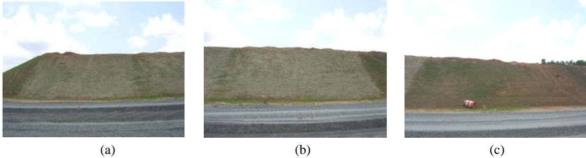
Figure 1.6. Oakdale Rd I hydroseeding plots June 2005. a. Wood hydromulch. b. Wood hydromulch + 20 lb/ac PAM. c. Straw + tackifier + 20 lb/ac PAM.
