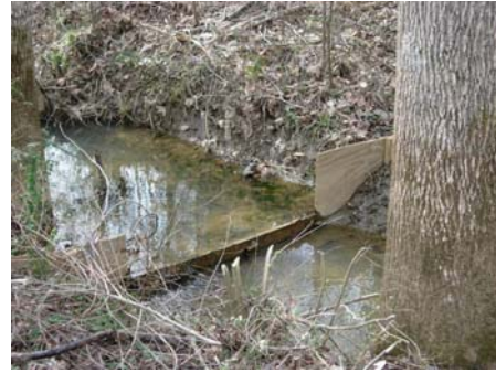
Figure 3.3. Stream 2 monitored cross section with rectangular weir.
