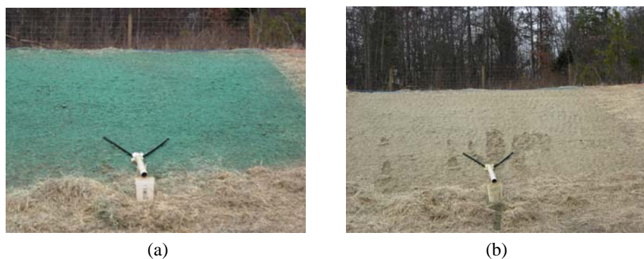
Figure 1.15. Wood hydromulch without PAM a. February 2, 2006 b. February 10, 2006, showing some failure starting at mid-slope.
