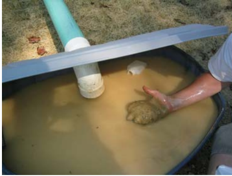
Figure 1.2. Runoff from PAM-treated plot showing flocculated sediment.
