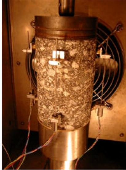
Figure 3.1 LVDT mounting and spacing
