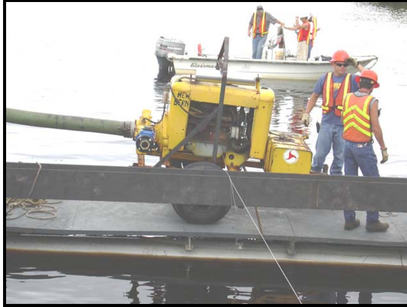
Figure 5-11 Hale model centrifugal trash pump used at first jetting site.
