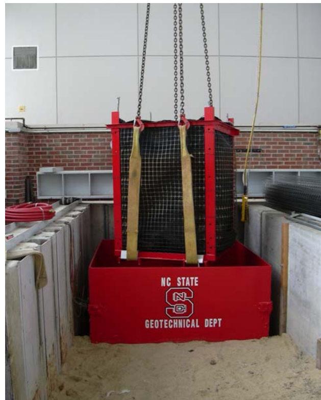
Figure 3-3 Saturation Tank and Specimen Basket
