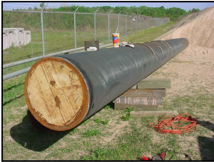
Figure 5-7 Steel Test Pile with plate welded onto bottom end.
