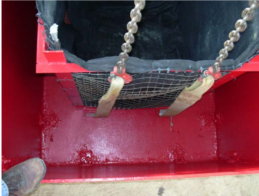
Figure 3-4 Overhead View of Saturation Tank with Specimen Basket in Place
