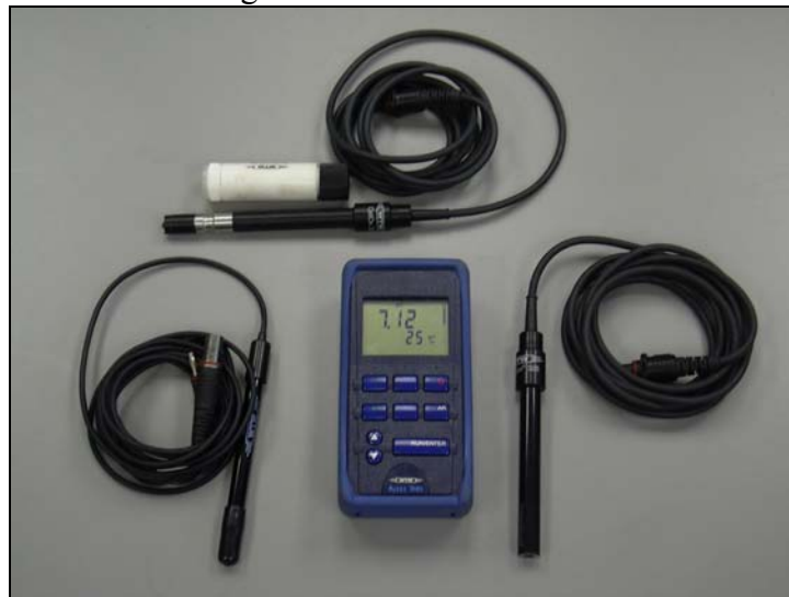
Figure 6-3 WTW measurement systems, Multi-340i with probes.
