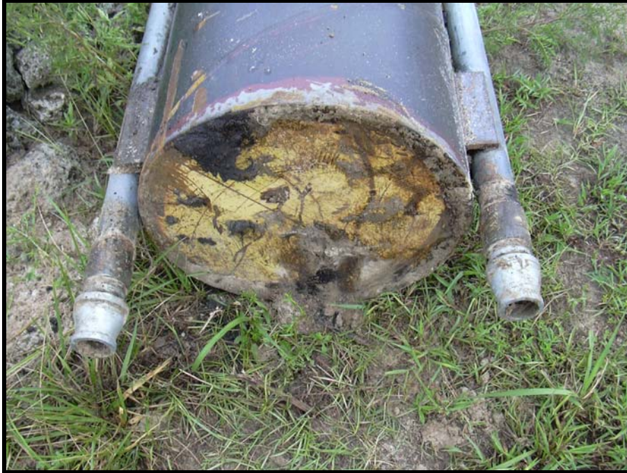
Figure 5-8 Nozzle ends at the ends of the jet pipe, shown with 2 inch (5.08cm) nozzles.
