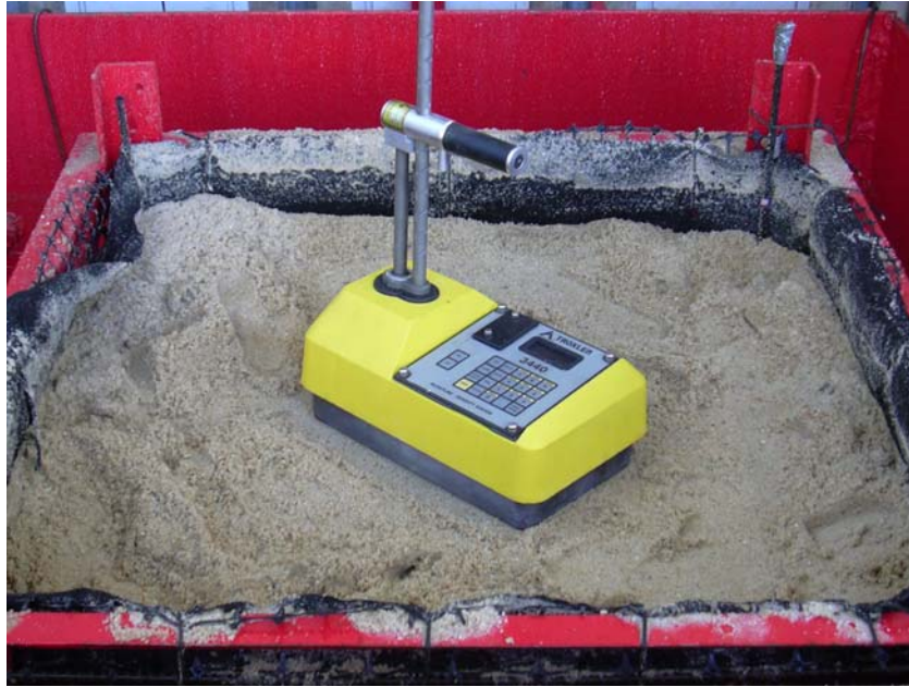
Figure 3-8 Density Check at Midpoint of Lift Height
