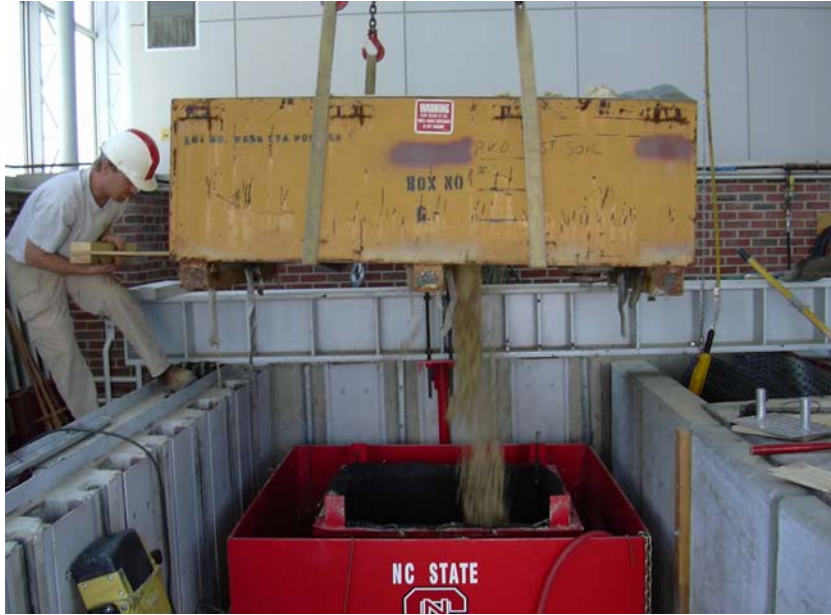
Figure 3-6 Free-fall of Specimen Soil for Desired Lift Height
