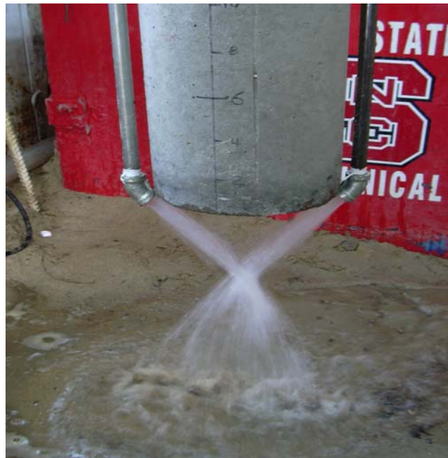
Figure 3-10 Angled Jet Nozzles for Jetting Modification
