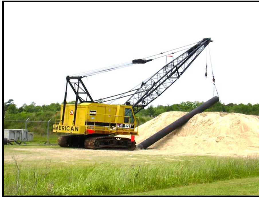
Figure 5-10 American model 5220 crane used for maneuvering test piles.
