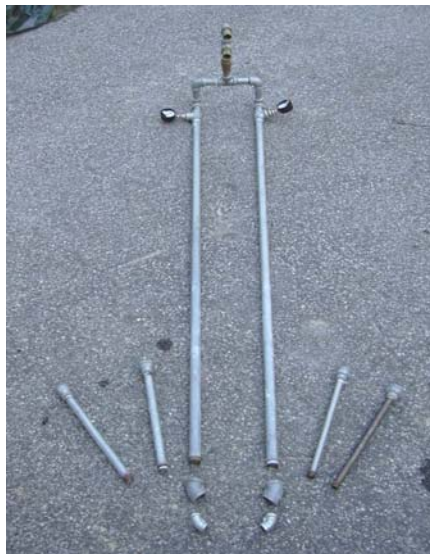
Figure 3-5 Laboratory Jetting Apparatus and Various Nozzles
