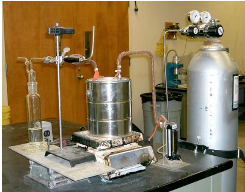
Figure 3-4 Extraction Device for Transferring Antistripping Additive from Asphalt Mix to the Aqueous Phase
