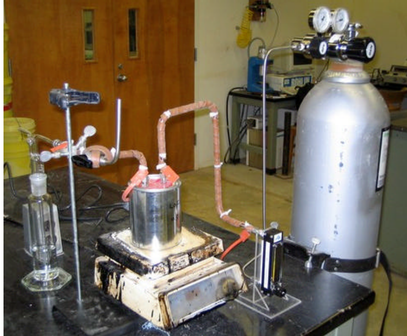
Figure 3-3 Extraction Device for Transferring Antistripping Additive from Asphalt Binder to the Aqueous Phase
