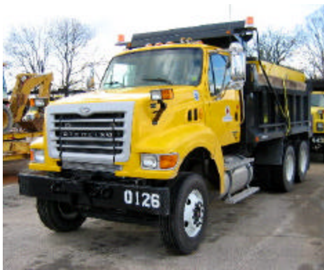
Figure 6-4. Front and Side Views of a Tier 2 Double Rear Axle (Tandem) Dump Truck (12.8 l engine displacement)
