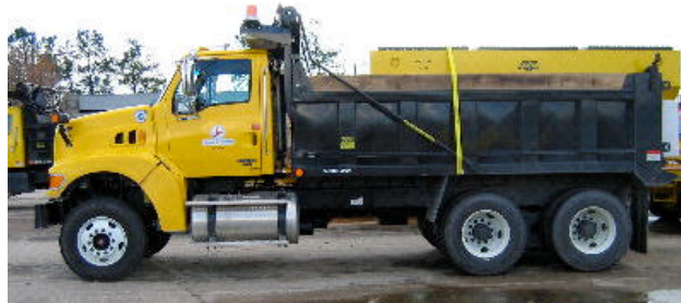
Figure 6-4. Front and Side Views of a Tier 2 Double Rear Axle (Tandem) Dump Truck (12.8 l engine displacement)
