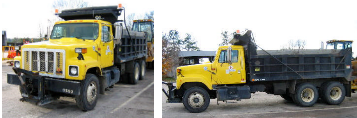
Figure 6-2. Front and Side Views of a Tier 1 Double Rear Axle (Tandem) Dump Truck (10.8 l engine displacement)
