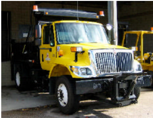
Figure 6-3. Front and Side Views of a Tier 2 Single Rear Axle Dump Truck (7.6 l engine displacement)
