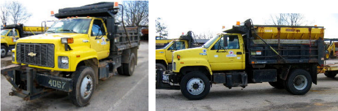
Figure 6-1. Front and Side Views of a Tier 1 Single Rear Axle Dump Truck (7.2 l engine displacement)
