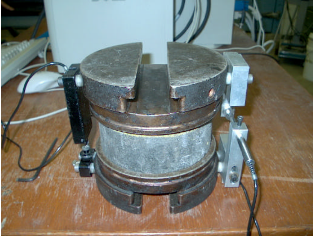
Figure 5.3 Simple Shear (FSTCH and RSTCH) Test Specimen
