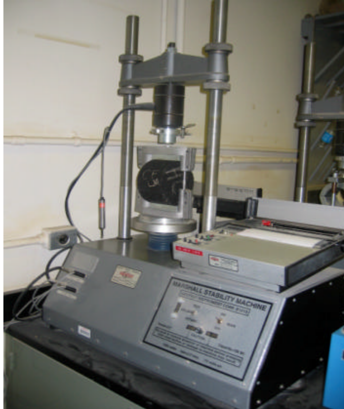
Figure 4.1. Loading frame used for measuring Indirect Tensile strength
