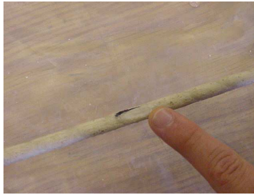
Figure E.1 Roughed-up area on GFRP rebar specimen
