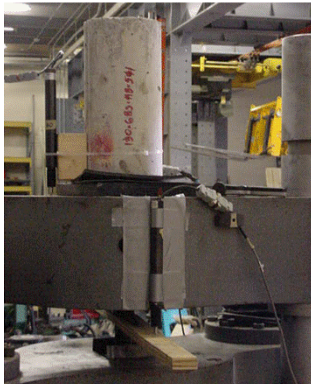
Figure 5.5 Actual Pullout Test Setup within UTM at UNC Charlotte
