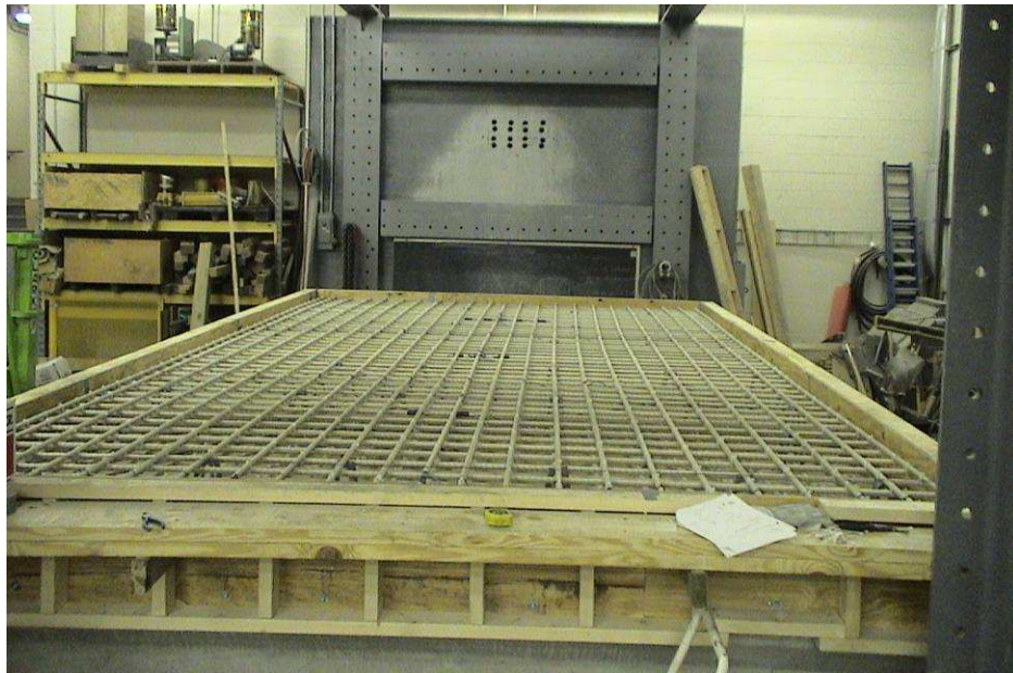
Figure 4.3 Reinforcement Details of Laboratory Model
