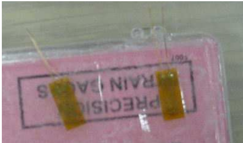
Figure 5.7 Strain Gages used to measure elongation of GFRP Rebar
