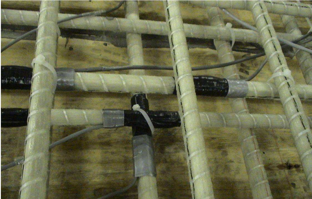
Figure 4.11 Strain Gages on the GFRP Rebar
