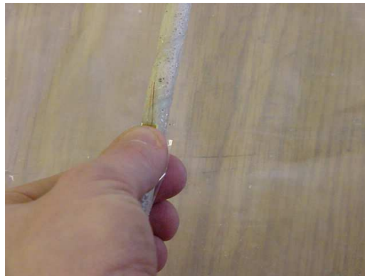
Figure E.3 Applying pressure to strain gage
