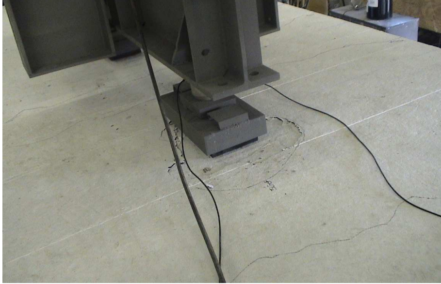
Figure 4.16 Punching Through the Concrete Deck – Top of the Deck (Bay 1)
