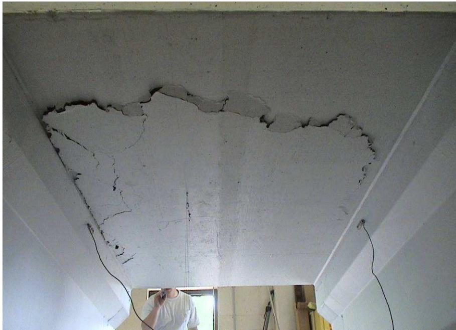
Figure 4.17 Punching Through the Concrete Deck – Bottom of the Deck (Bay 1)
