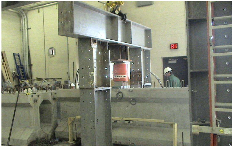
Figure 3.16 Prestressed Girder Testing
