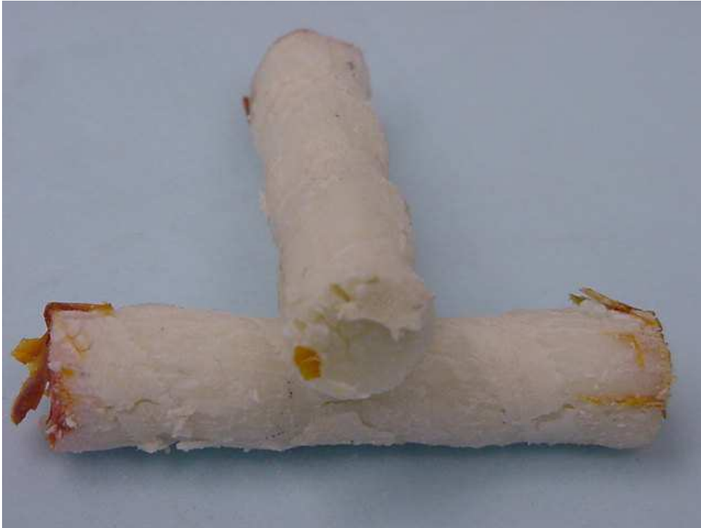
Figure 7.7 Kodiak 130°F Absorption Specimens at 9 Month Duration
