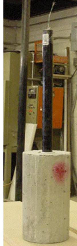
Figure 5.3 Bond-Slip Reinforced Substrate
