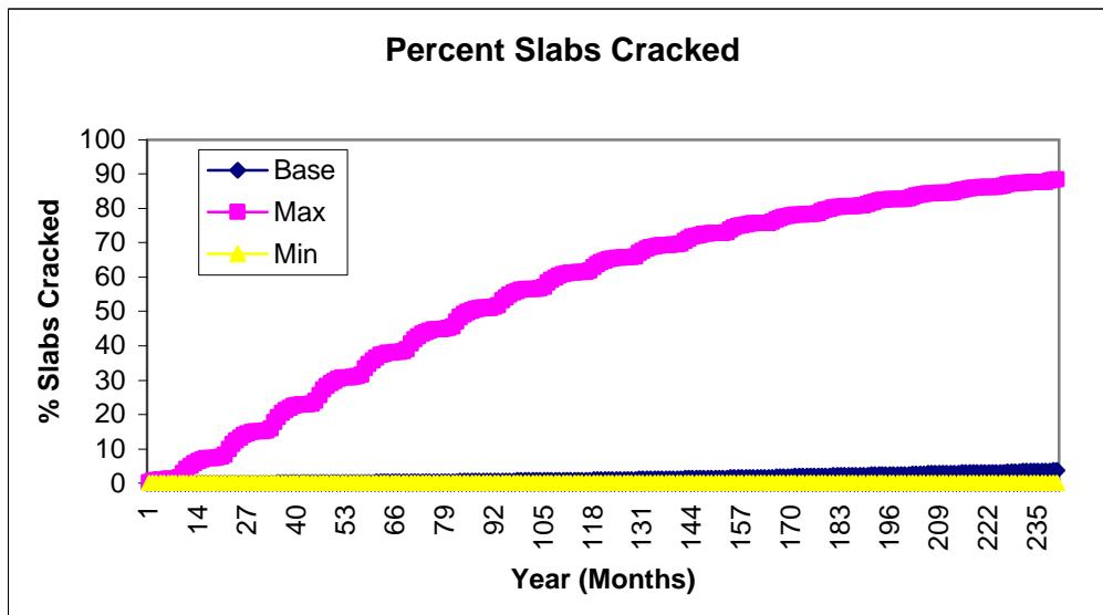
**Figure D -328 0201 Coefficient of Thermal Expansion- JPCP**
