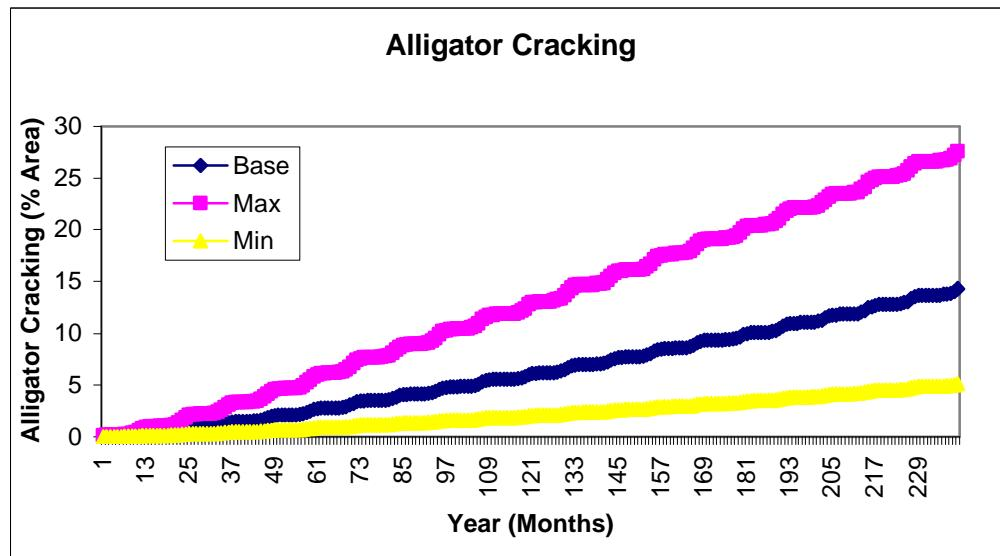
**Figure D -188 0901 – Airvoids – Treated Base**
