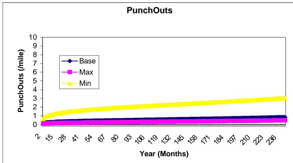
**Figure D -517 5827 ThermalConductivity - CRCP**
