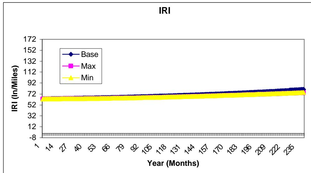
**Figure D -440 3011 Subgrade Modulus**
