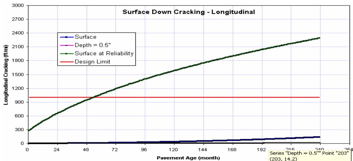
**Figure E - 10 Run-1-with 90% Alligator Cracking – Maximum - Thermal Conductivity**
