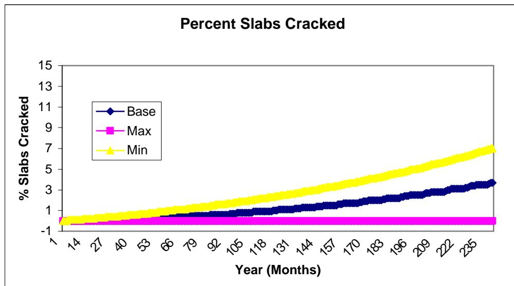
**Figure D -430 3011 ThermalConductivity - JPCP**
