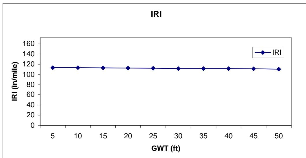
**Figure D -573 5037 Ground Water Table**
