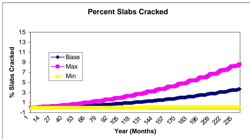
**Figure D -403 0209 Surface Shortwave Absorptivity**
