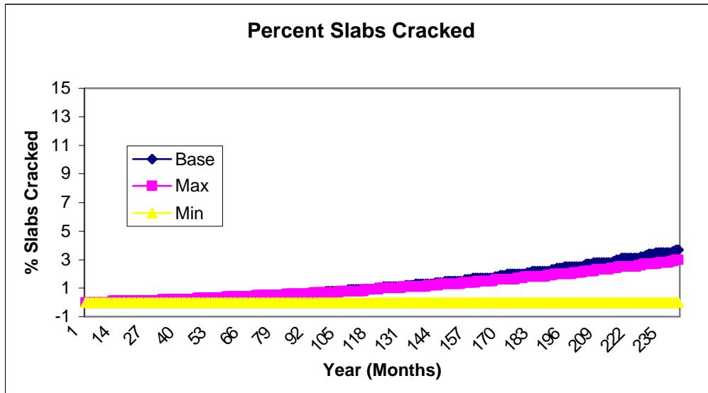
**Figure D -424 3011 Coefficient of Thermal Expansion - JPCP**
