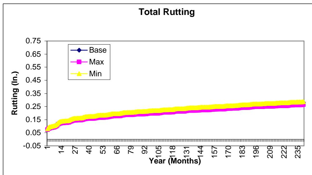
**Figure D -120 1814 – Subgrade Modulus**
