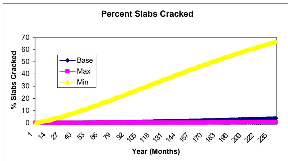
**Figure D -379 0209 ThermalConductivity - JPCP**
