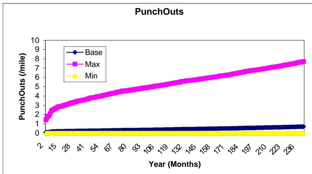
**Figure D -541 5037 Coefficient of Thermal Expansion - CRCP**
