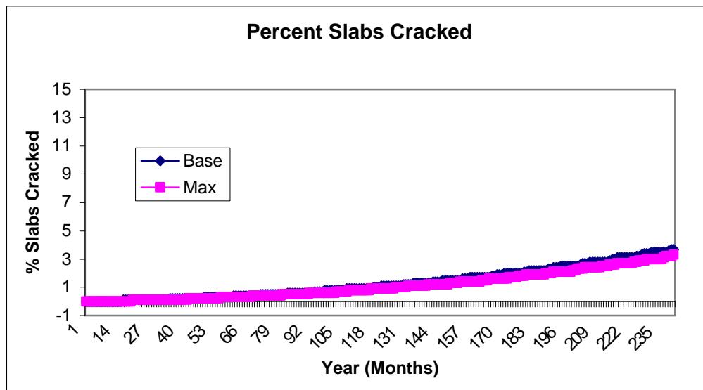
**Figure D -371 0209 Coefficient of Thermal Expansion - JPCP**
