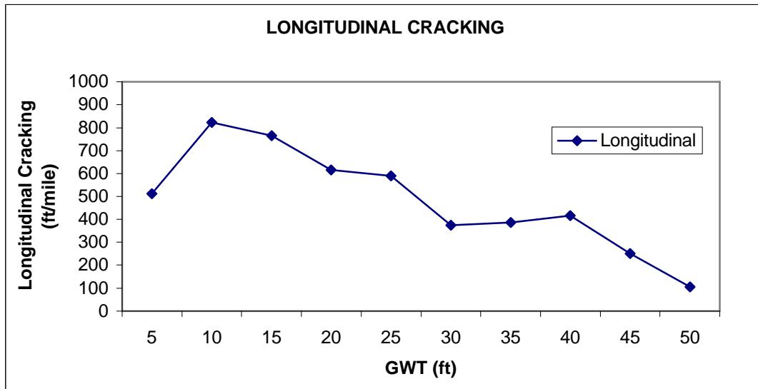
**Figure D -570 1814 Ground Water Table**
