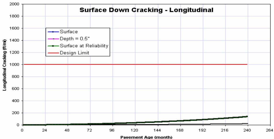
**Figure E - 18 Run-1-with 50% Reliability case Alligator Cracking – Minimum - Thermal conductivity**
