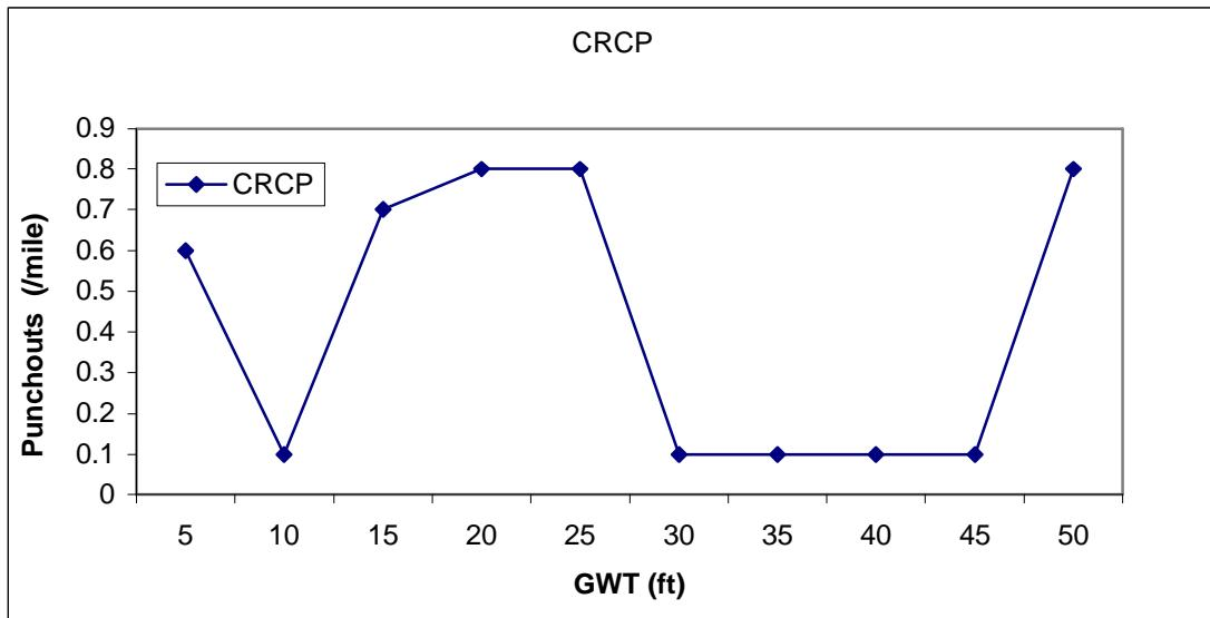
**Figure D -574 5037 Ground Water Table**
