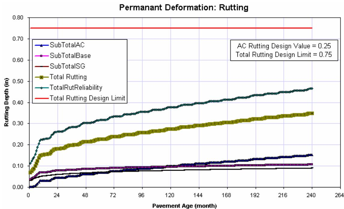
**Figure E - 4 Run-1-with 90% IRI - Base case**
