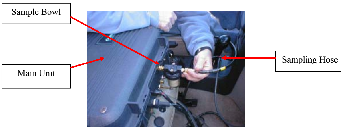
Figure C-6. Attachment of the Sampling Hose to the Main Unit
