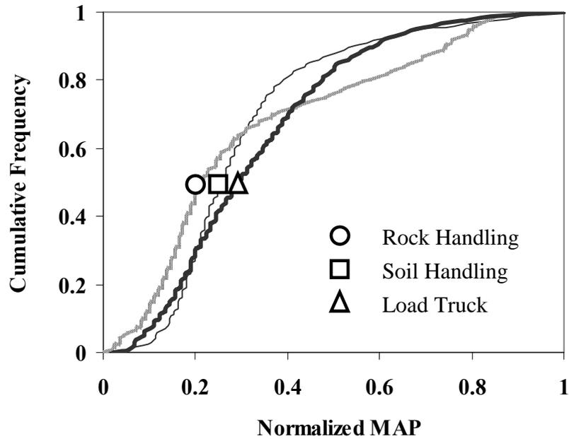
**Figure 15. Cumulative Frequency of Normalized MAP for Three Representative Duty Cycles for a Front-End Loader**
