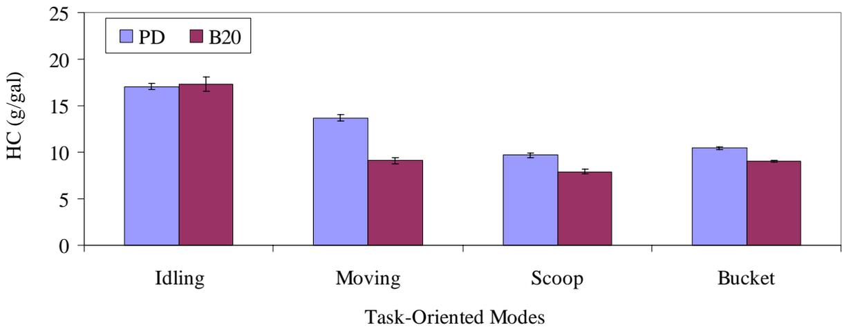
**Figure 13. Comparison Between Petroleum Diesel and B20 Biodiesel of Average Fuel Use and Emission Rates of Each Pollutant on a Per Gallon of Fuel Consumed Basis for Task-Oriented Based Modes for Backhoe 1**
