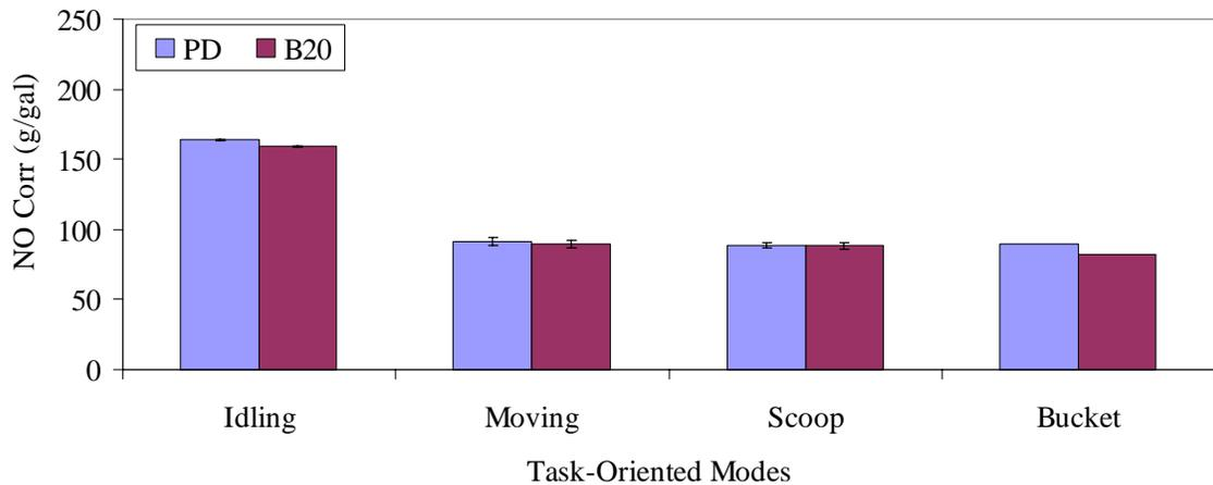
(c) Fuel-based NO as equivalent NO<sub>2</sub> emission rate, corrected for ambient temperature and humidity
