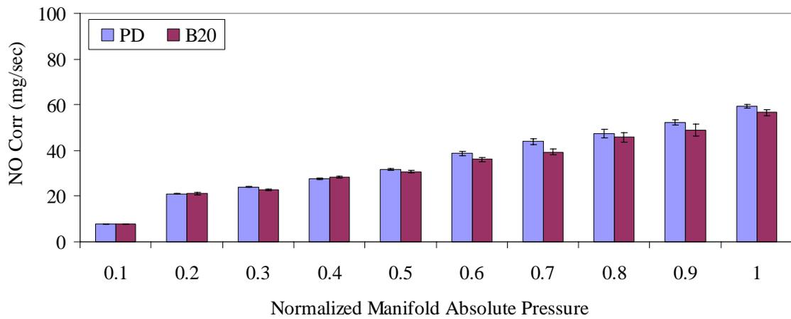
(b) Time-based NO as equivalent NO<sub>2</sub> emission rate, corrected for ambient temperature and humidity
