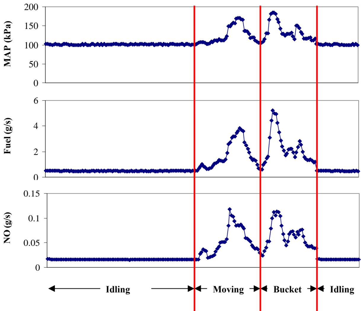
**Figure 9. Example of a Time Series Plot of Manifold Absolute Pressure, Fuel Use, and NO as Equivalent NO<sub>2</sub> Emission Rate for a Front-End Loader**
