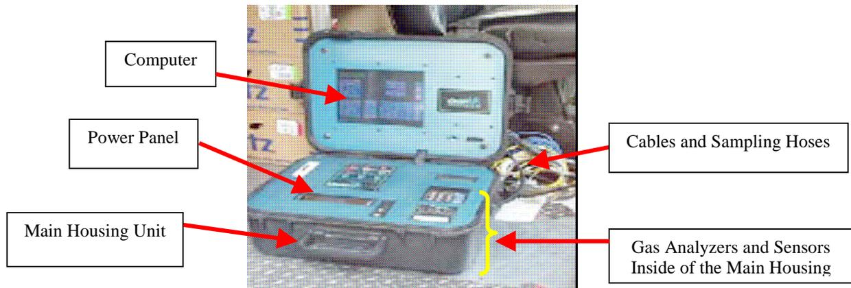
**Figure 1. Montana System Components**
