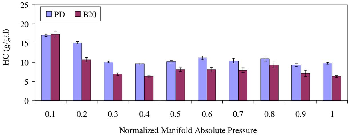
**Figure 11. Comparison between Petroleum Diesel and B20 Biodiesel of Average Fuel Use and Emission Rates of Each Pollutant on a Per Gallon of Fuel Consumed Basis for Engine-Emission Based Modes for Backhoe 1**
