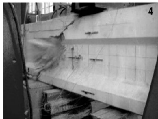
Figure 4.39 Progressive failure of AASHTO2C girder (front side)
