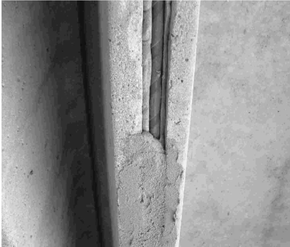
Figure 8.7 NSM bar in groove
