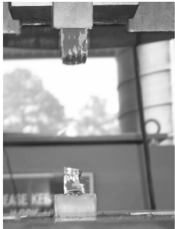
Figure 4.20 Failure through the fibers (left) and failure through cross section (right)
