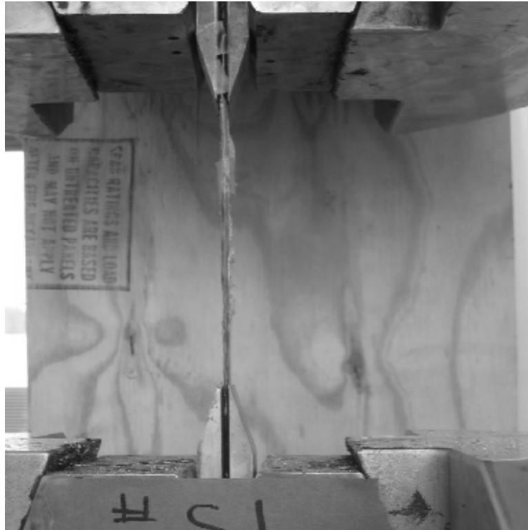
Figure 4.19 Typical CFRP tension test setup
