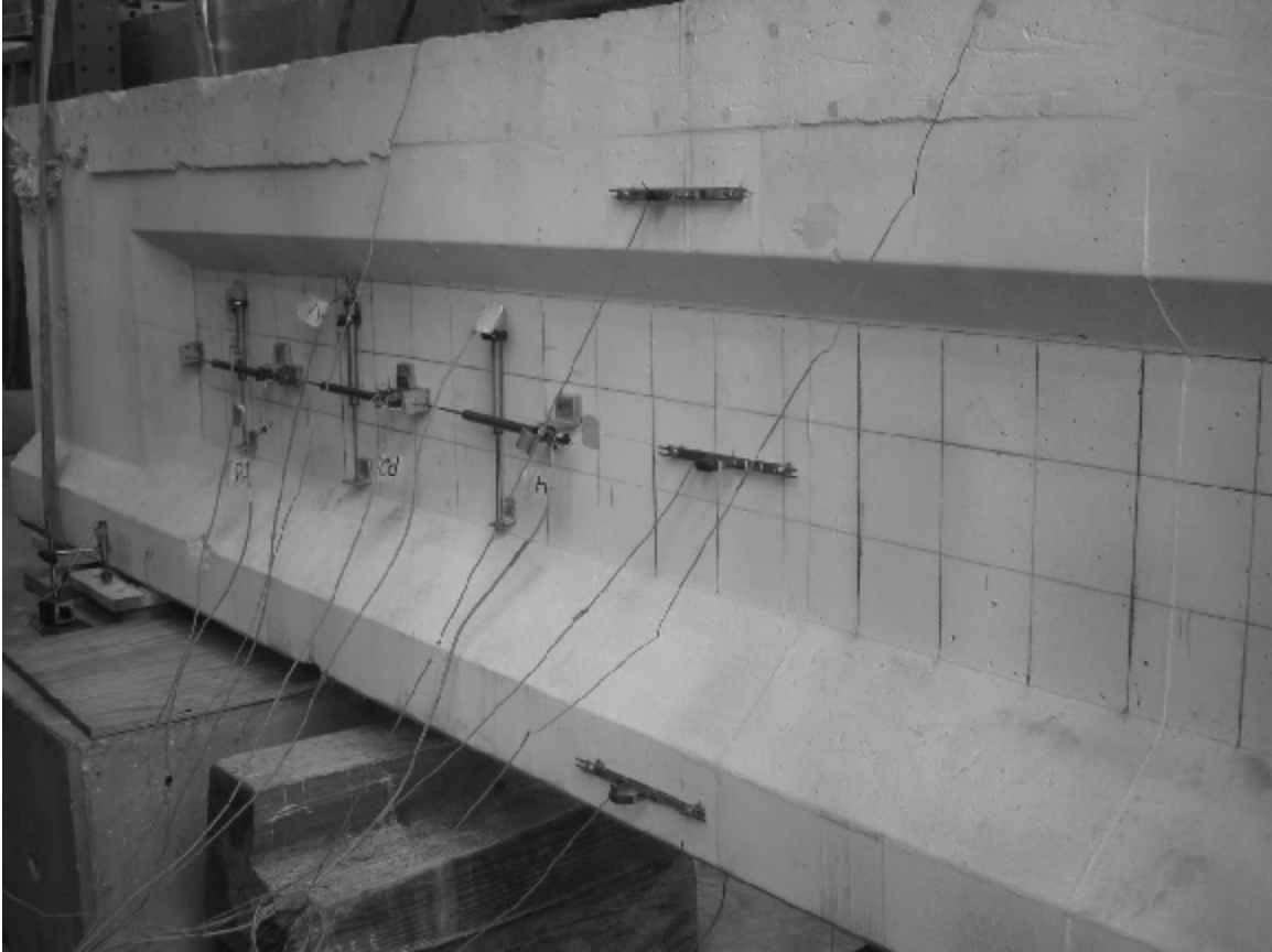
Figure 4.33 Typical layout of linear potentiometers for AASHTO2C and AASHTO2R
