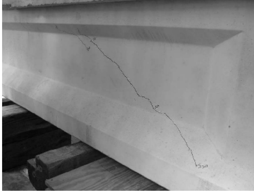
Figure 4.38 Initial shear cracks in AASHTO2C girder (back side)
