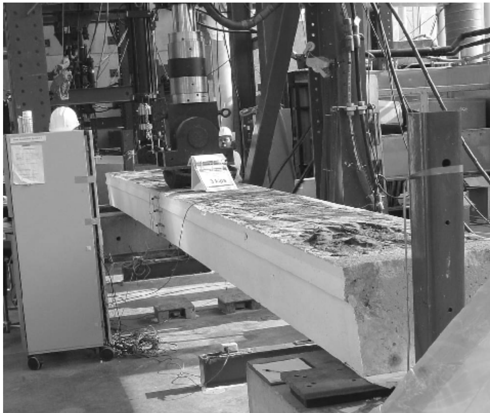
Figure 3.6 Typical test setup for C-Channel girders tested under static loading conditions
