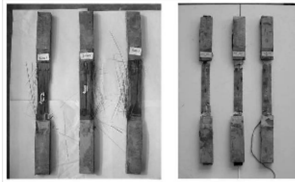
Figure 3.5 Typical pre-cured (left) and wet lay-up (right) specimens after tension testing
