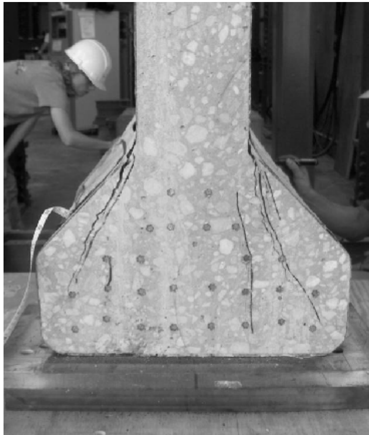
Figure 4.40 Failure in transfer zone of girder AASHTO2R
