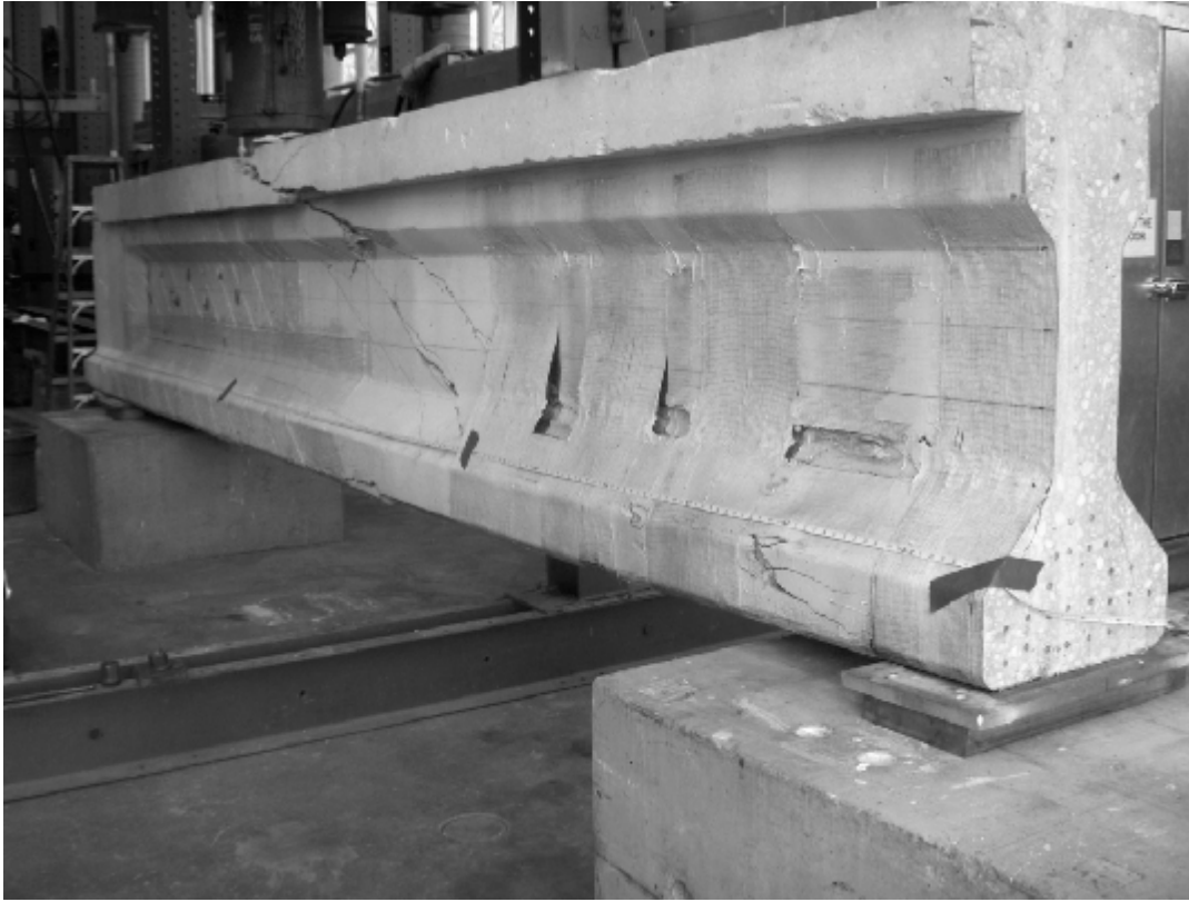
Figure 4.41 Failure of AASHTO2R girder (front side)
