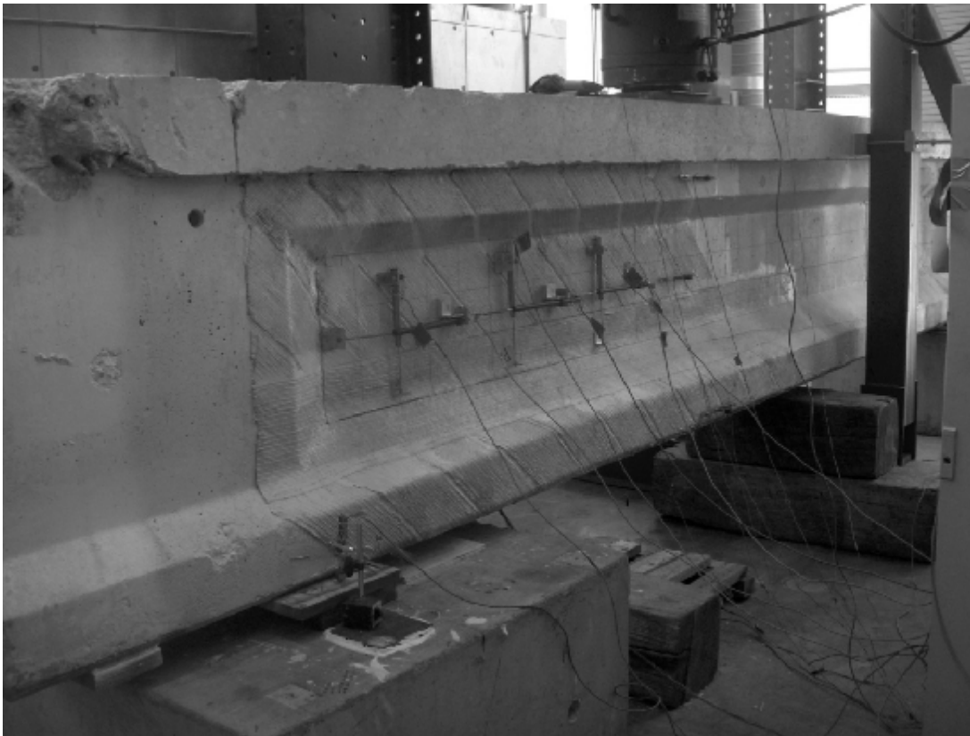
Figure 4.12 AASHTO2R test specimen
