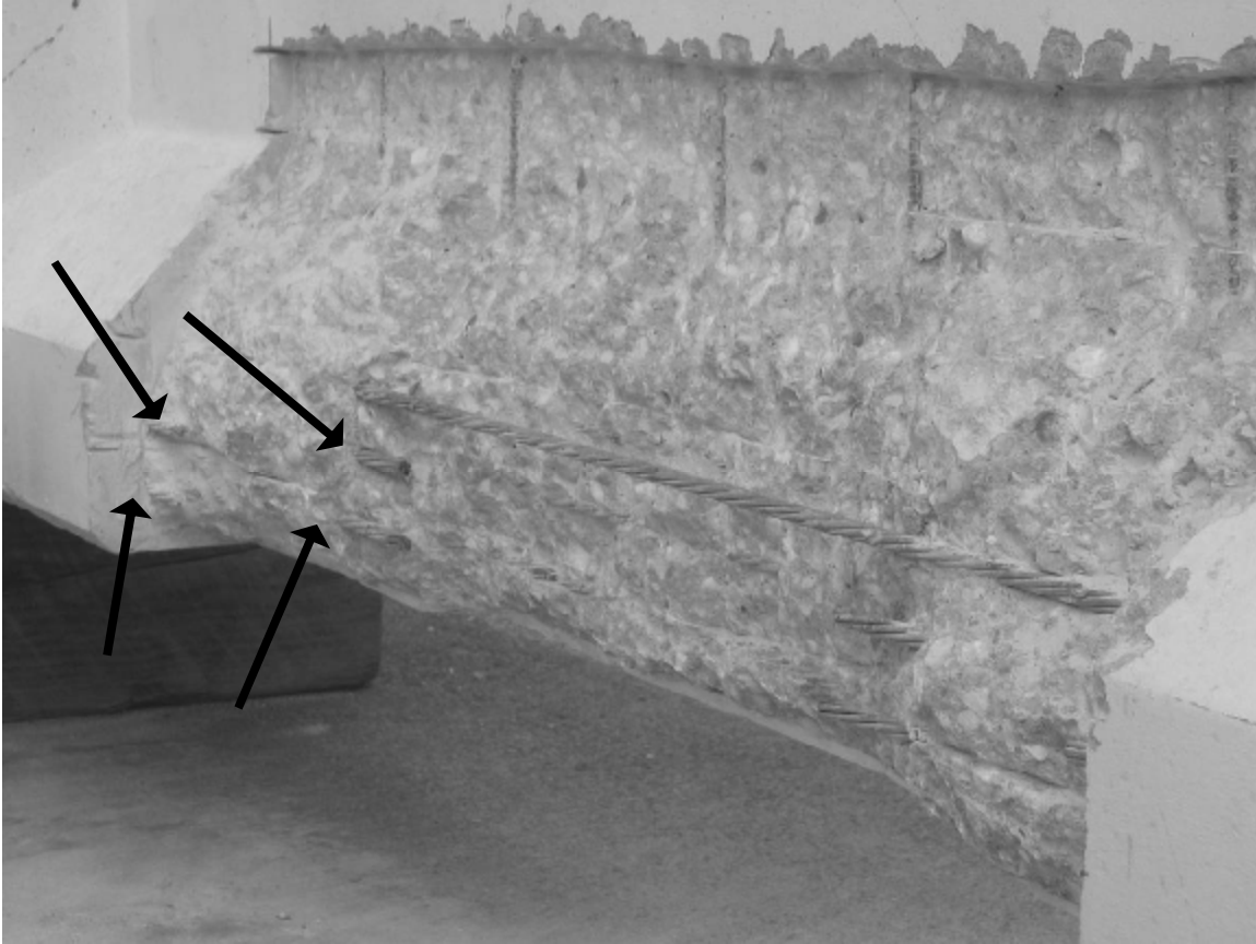
Figure 4.14 AASHTO2R after completion of simulated damage
