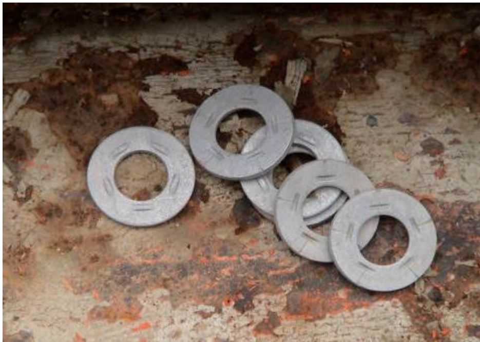
Figure A-16. Collapsible Washer Used for Tightening Bolts
