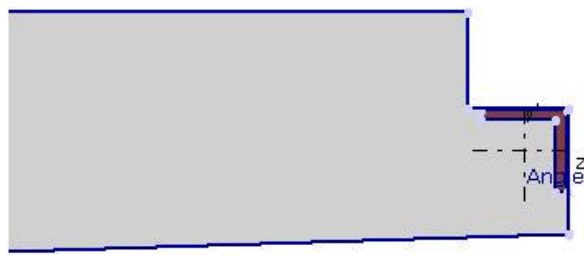
Figure 2-5. Larsa™ Embedded Steel Angle Detail
