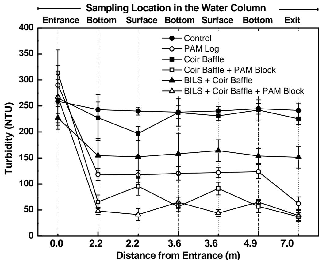
Figure 2-5. Treatment effects on turbidity within the stilling basin under with either no baffles or three coir baffles.
