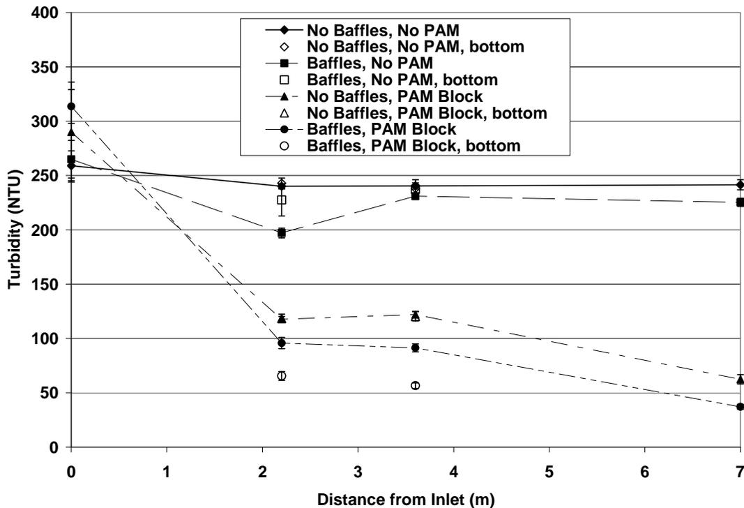
Figure 1-7. Turbidity at different points in the stilling basin as affected by porous baffles and dosing with a solid PAM block. The 7 m point is the outlet spillway.
