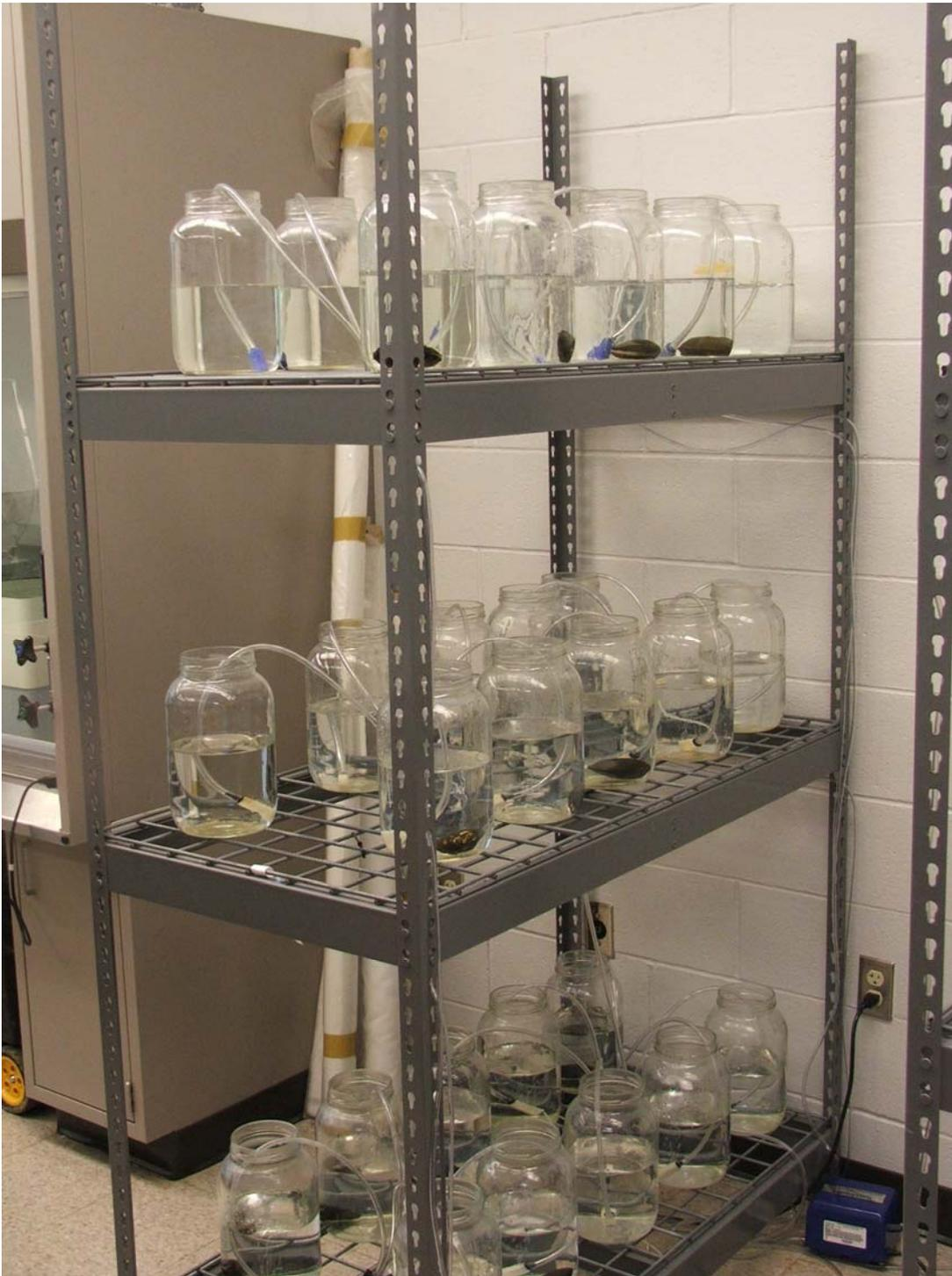
**Figure 5-1. Jar setup with aeration for 28 day Pb exposure study.**
