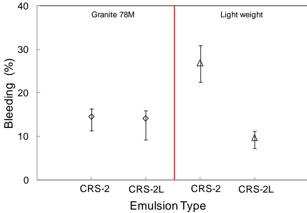
Figure 5-6 Calculated bleeding rates of the single seal
