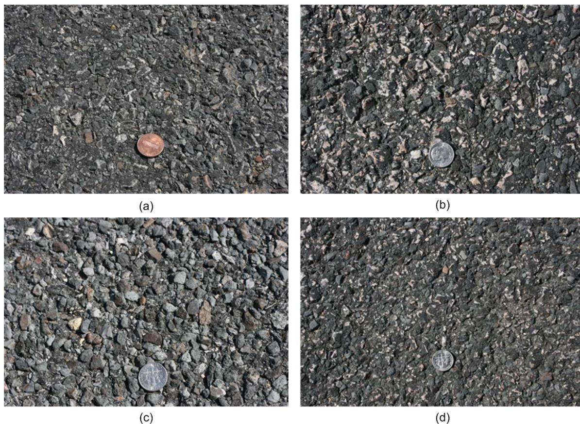
**Figure 7-4 Surface texture of the triple seal for comparison between Phase I and Phase II construction programs: (a) CRS-2 in Phase I; (b) CRS-2 in Phase II; (c) CRS-2P in Phase I; (d) CRS-2P in Phase II**
