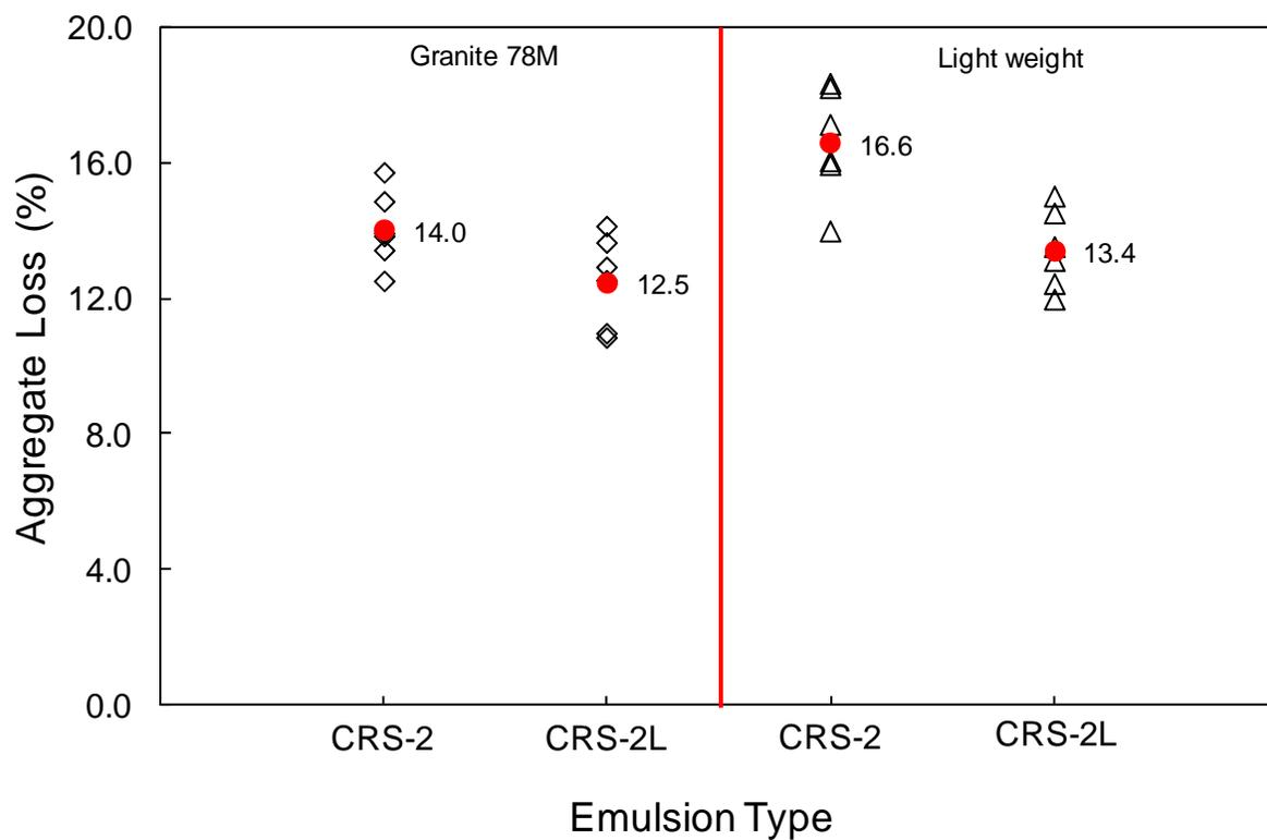
**Figure 4-10 Aggregate loss of a single seal**
