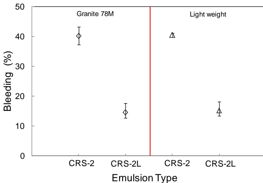
**Figure 5-10 Calculated bleeding rates of double seal**
