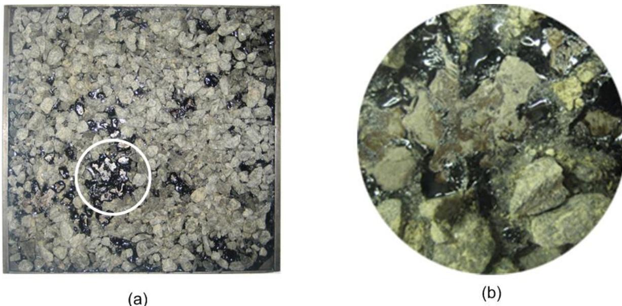
**Figure 4-7 Separation of emulsion from the Vialit steel plate when an impact is applied to the sample conditioned at  $-20^{\circ}\text{F}$ : (a) after testing the specimen; (b) circle area, magnified**
