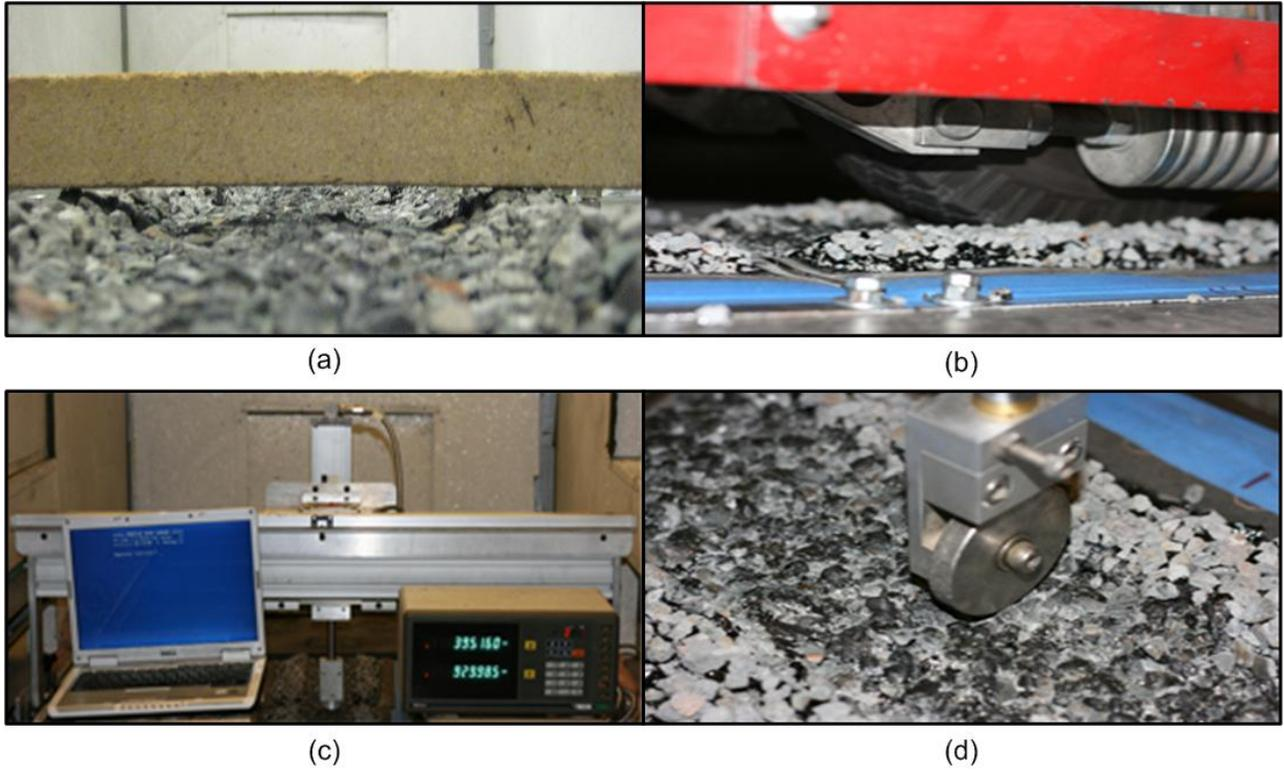
**Figure 3-7 Front view of rut depth and profile system: (a) final rut depth of the triple seal after MMLS3 testing; (b) MMLS3 tire on the triple seal; (c) transverse profile measurement using Mitutoyo profilometer; (d) profilometer on the specimen**
