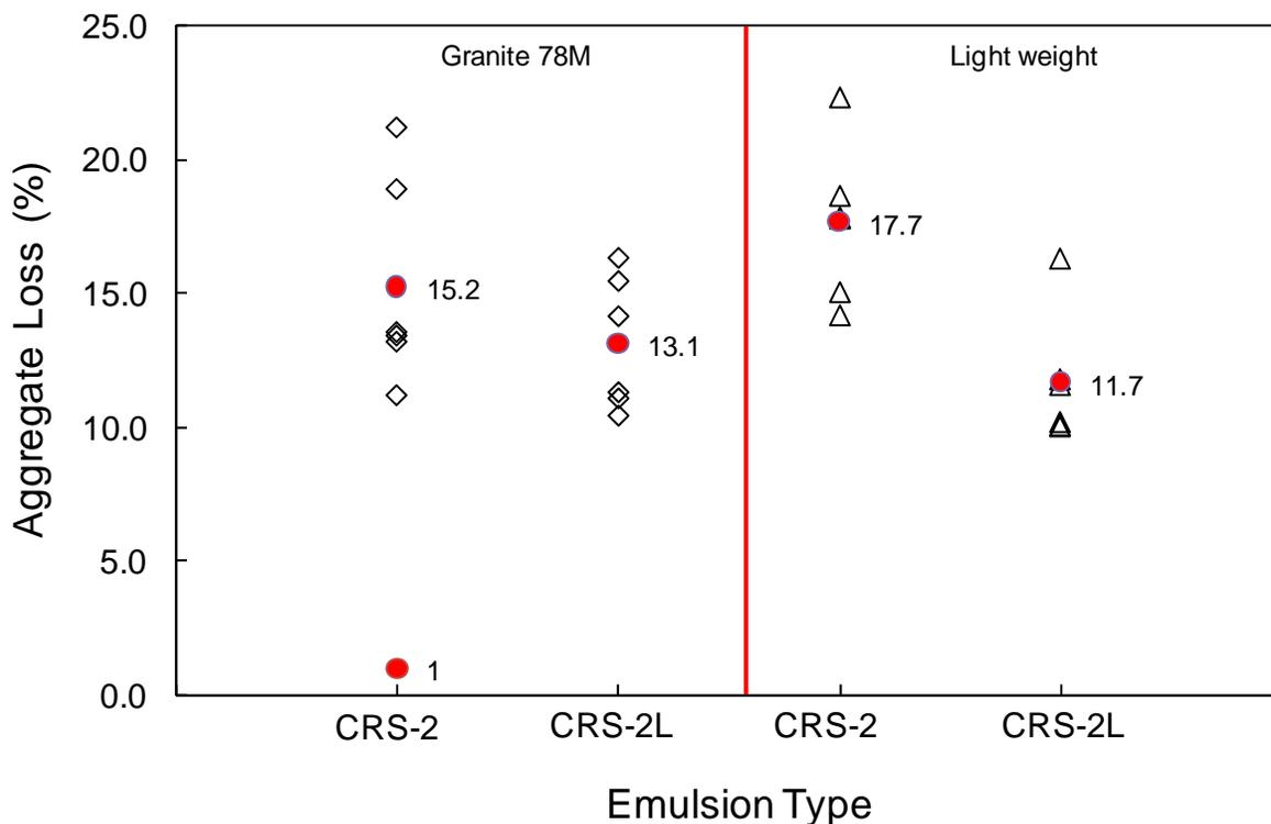
**Figure 4-11 Aggregate loss of a double seal**
