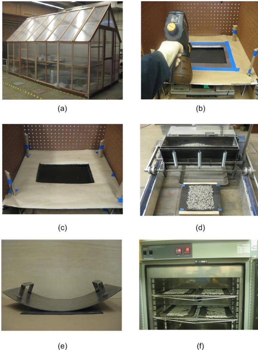
**Figure 3-3 Chip seal specimen fabrication procedure: (a) greenhouse; (b) emulsion application gun; (c) applied CRS-2 on the felt paper; (d) applied aggregate on the emulsion by ChipSS; (e) hand steel compactor with neoprene sheet; (f) sample curing in the oven**
