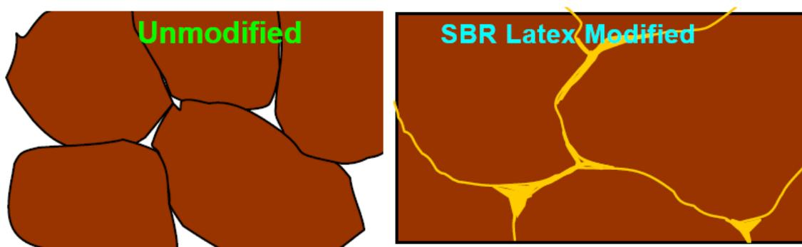
**Figure 2-1 Schematic diagram of fully cured unmodified and SBR latex polymer-modified asphalt (Takamura 2003)**
