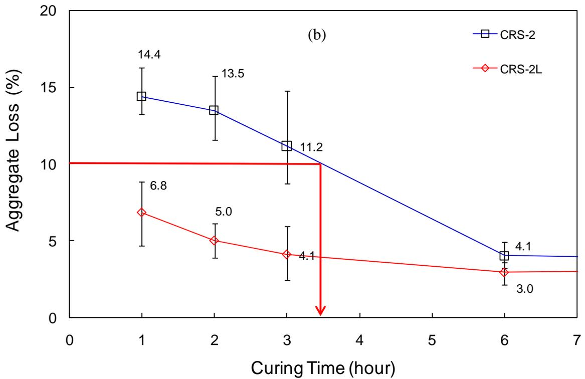
**Figure 4-4 Average aggregate loss measured from the Vialit test as a function of curing time (first three hours): (a) granite 78M; (b) lightweight**
