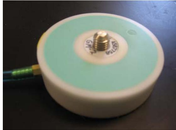
Figure 6.5 The specimen placed in the piston prior to fixing the reaction plate over it
