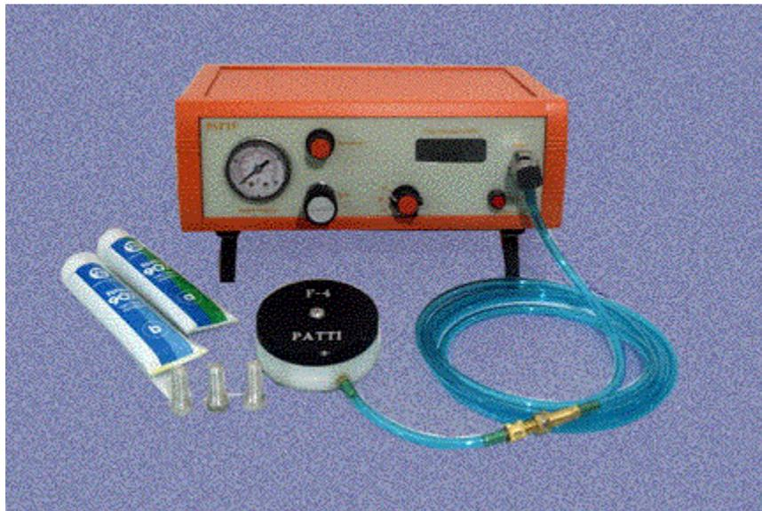
Figure 6.1 Pneumatic Adhesion Tensile Testing Instrument
