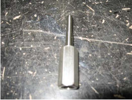
Figure 6.2 The adaptor designed to control the thickness of the sample
