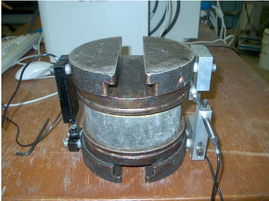
Figure 5.3 Simple Shear (FSTCH and RSTCH) Test Specimen
