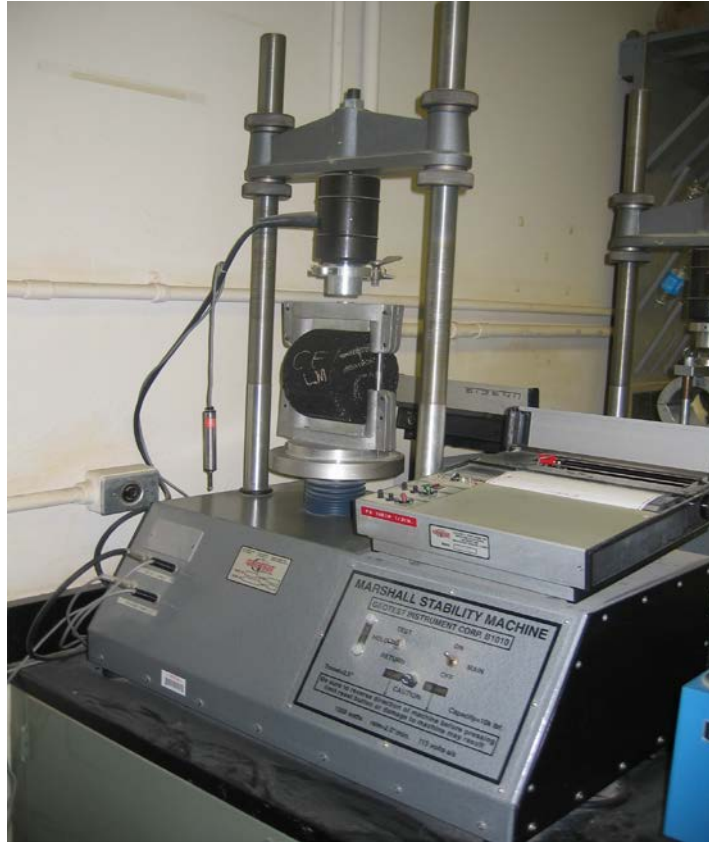
Figure 3.4 Loading frame used for measuring Indirect Tensile strength
