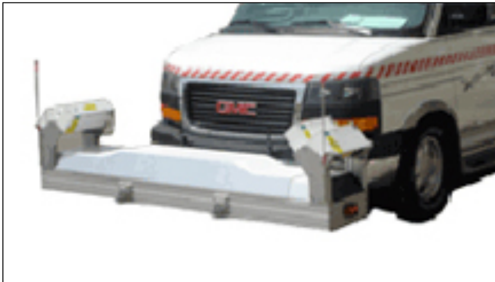
Figure 19 Hawkeye 2000 digital laser profiler
