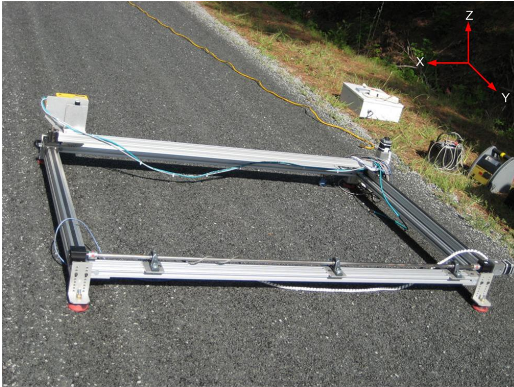
Figure 20 Photo of the 3-D laser profiler scanning a chip seal field section
