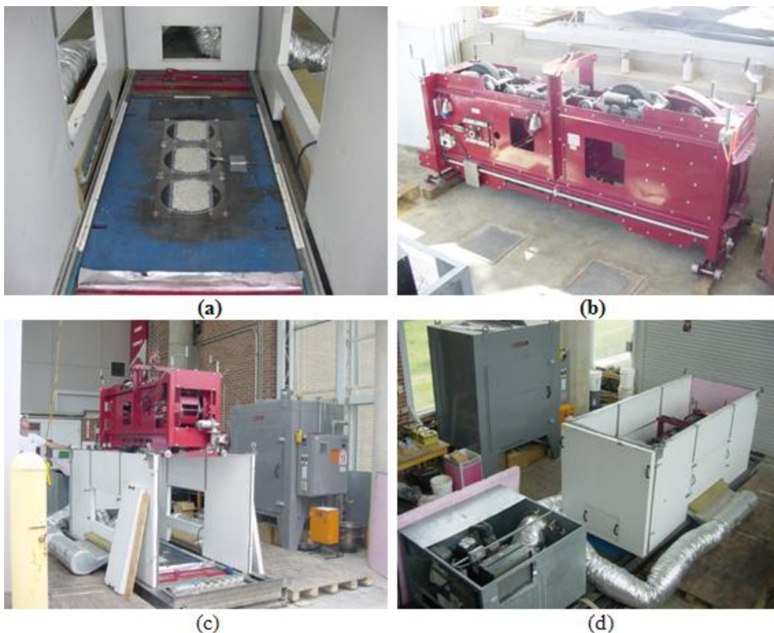
Figure 7 MMLS3 test preparation: (a) installation of specimens on a steel base, (b) side view of the MMLS3, (c) positioning the MMLS3 in the temperature chamber, and (d) complete MMLS3 test setup for testing
