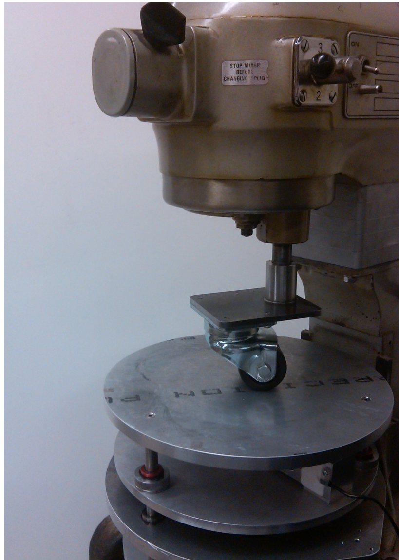
Figure 46 Modified sweep tester showing the free-rotating wheel on top of the adjustable platform
