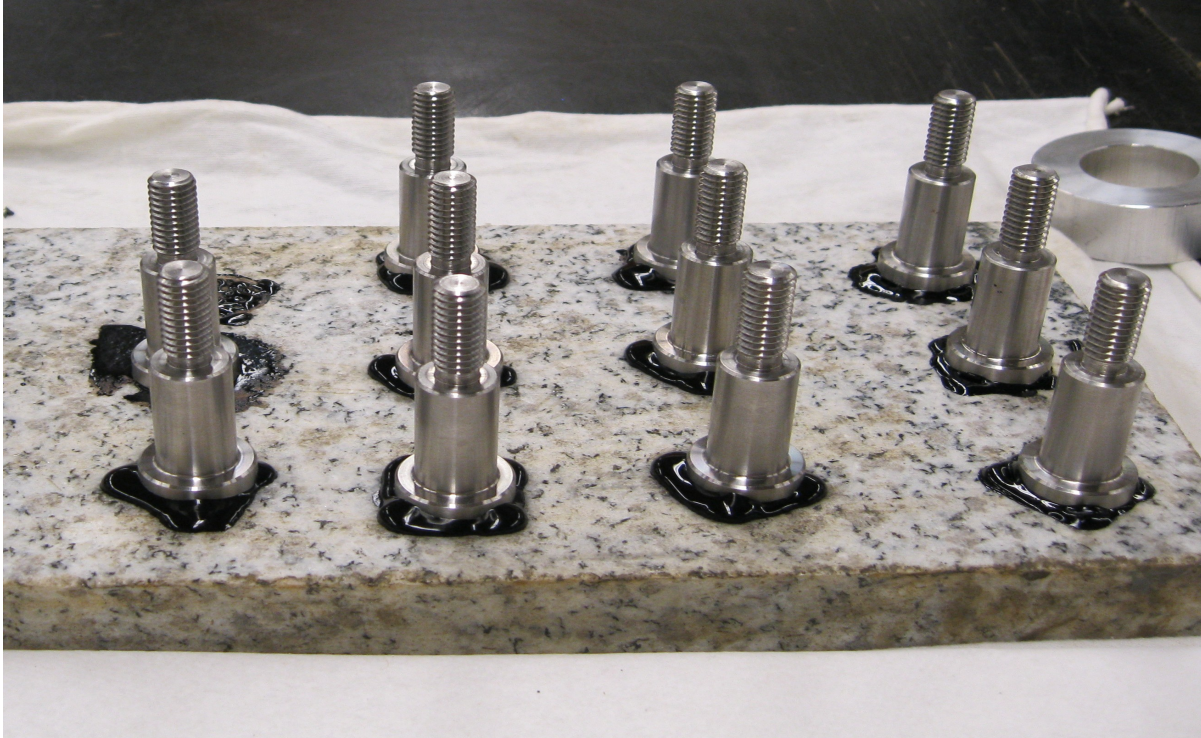
Figure 49 Pullout stubs on top of granite substrate with CRS-2L emulsion, after curing
