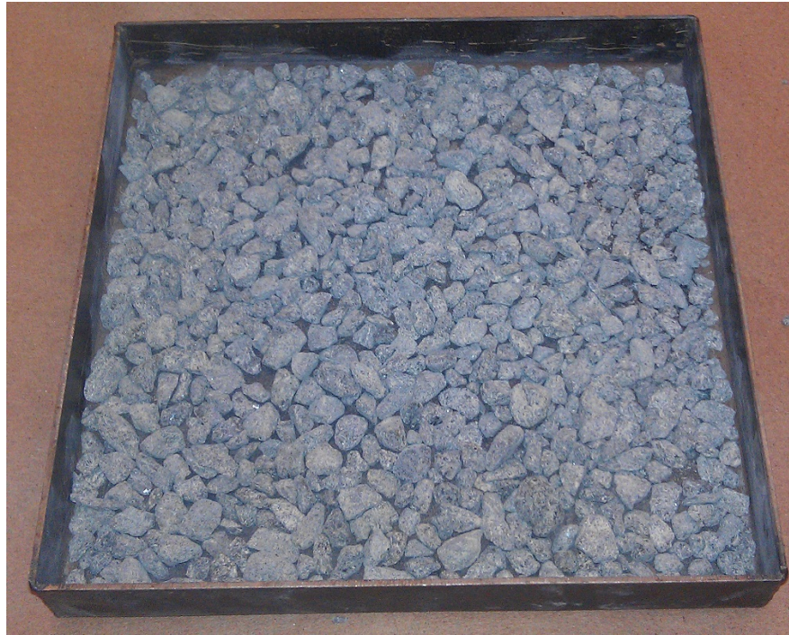
Figure 56 Single-layer aggregate board test using 8 in. x 8 in. steel plate
