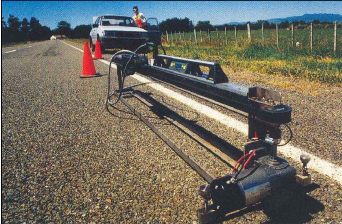
Figure 18 Stationary laser profilometer (SLP)
