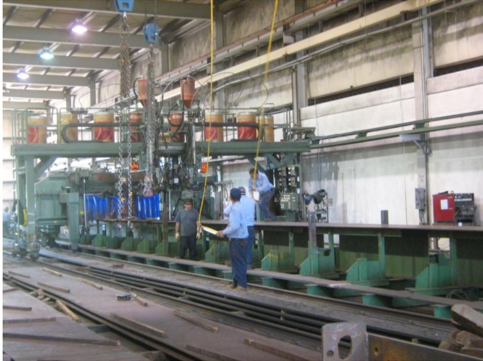
Figure 18: Machine for performing web to flange fillet welds
