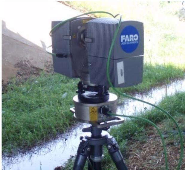
Figure 30: Faro LS 880HE laser scanner
