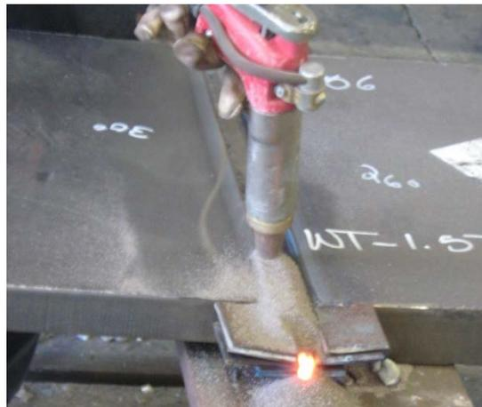
Figure 15: Welding of a flange splice
