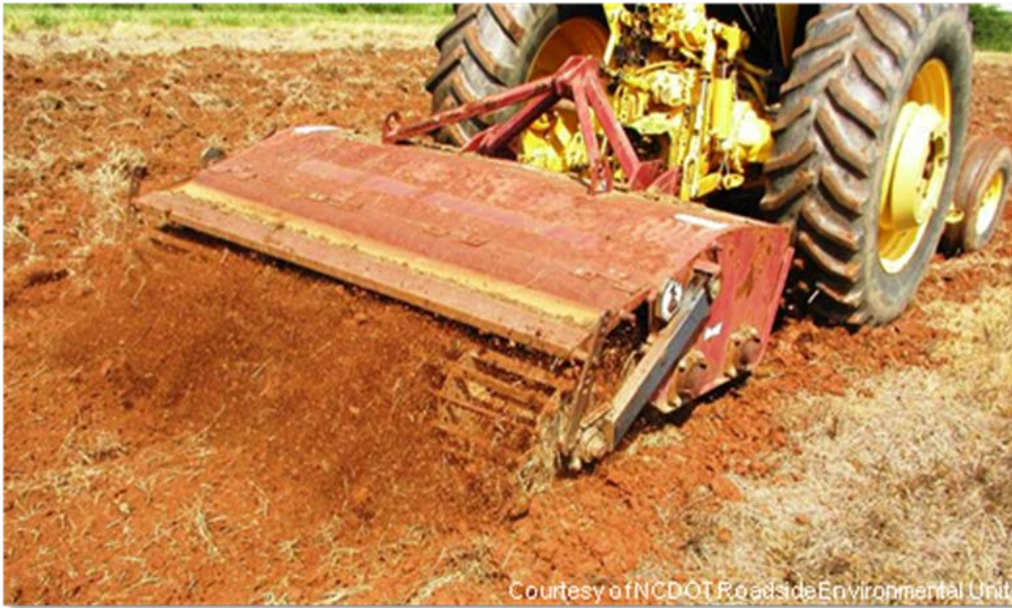
Figure A2.1 Rotary tillage with New Holland 6640 tractor (New Holland North America, Inc., New Holland, Pa.) coupled with M&W Dyna-Drive surface cultivator (NCDOT)
