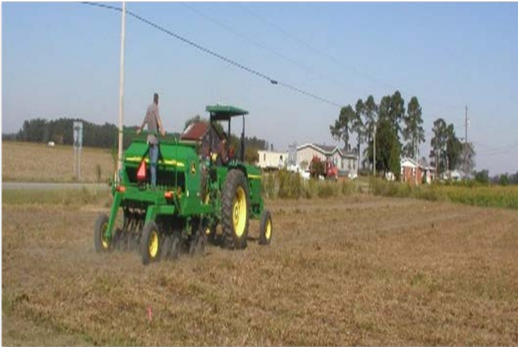
Figure A2.1 Rotary tillage with New Holland 6640 tractor (New Holland North America, Inc., New Holland, Pa.) coupled with M&W Dyna-Drive surface cultivator (NCDOT)
