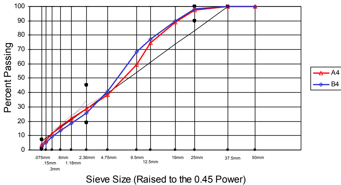
Figure C.4 Sieve analysis result from 4 th layer of I 540
