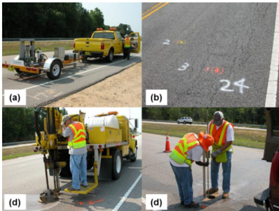
Figure 2.8 Photographs of field investigation procedure: (a) FWD testing, (b) coring spot marking, (c) coring machine mounted on truck, and (d) DCP testing.
