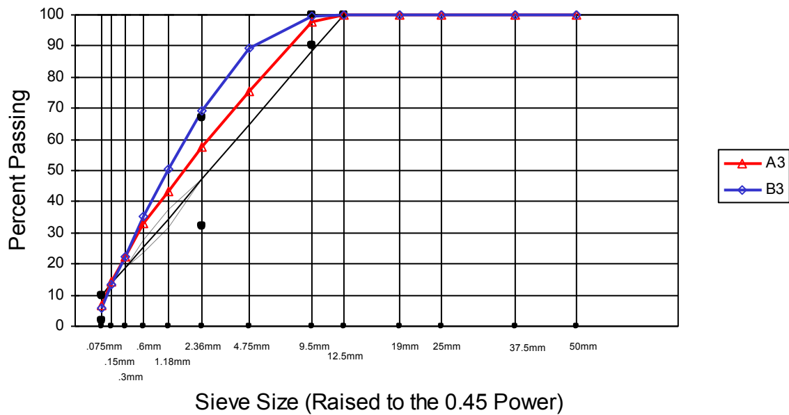
Figure C.87 Sieve analysis result from the 3 rd layer of NC-194
