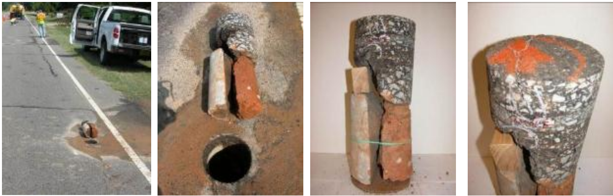
Figure B.77 Photographs of Sample Core Taken for the Verification of Roadway Expansion
