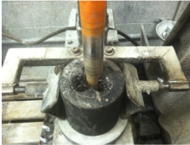
Figure 3.13 Photograph of vertical coring for 38 mm specimen.
