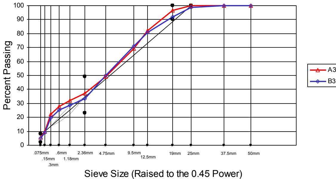
Figure C.21 Sieve analysis result from the 4 th layer of US-17
