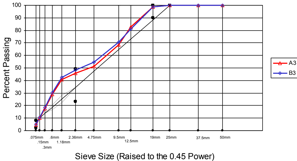
Figure C.53 Sieve analysis result from the 3 rd layer of US-74
