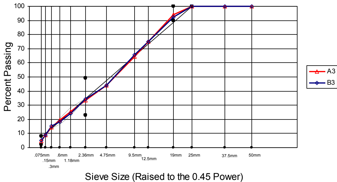
Figure C.71 Sieve analysis result from the 3 rd layer of NC-209
