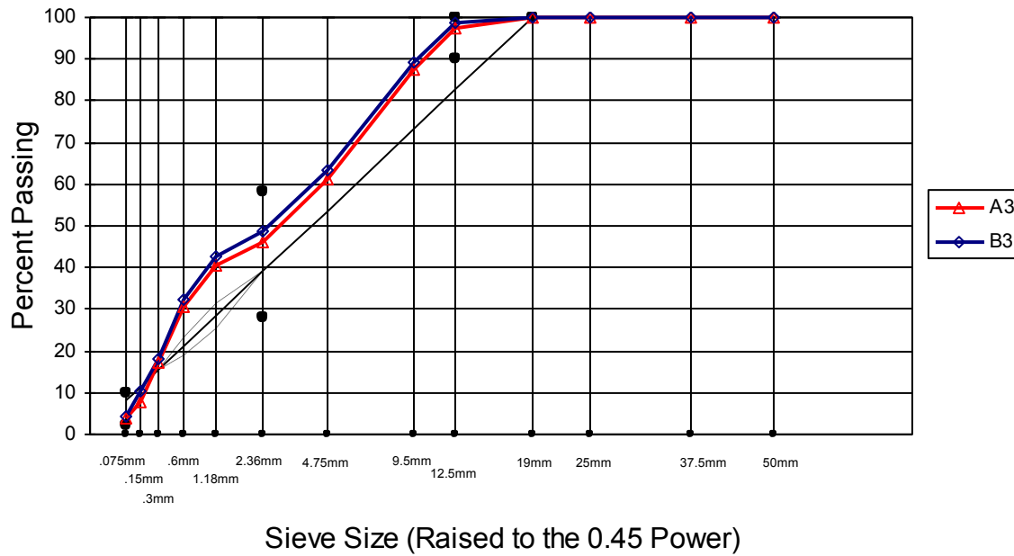
Figure C.108 Sieve analysis result from the 3 rd layer of NC-55
