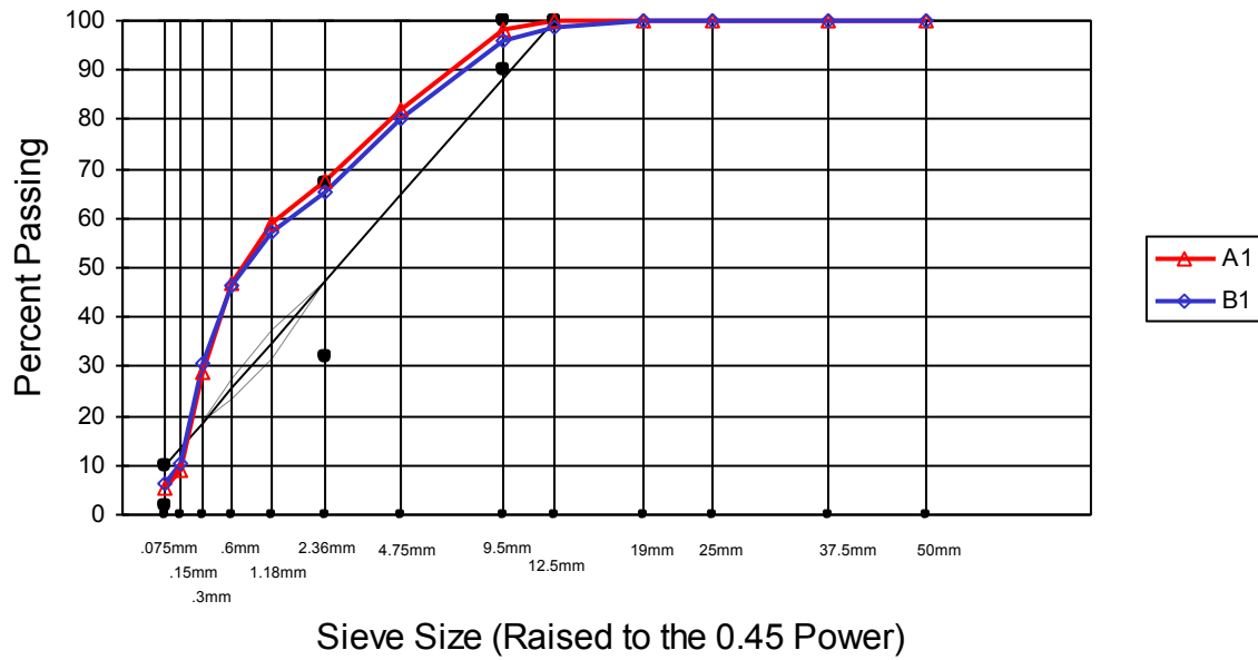
Figure C.110 Sieve analysis result from the 1 st layer of NC-179
