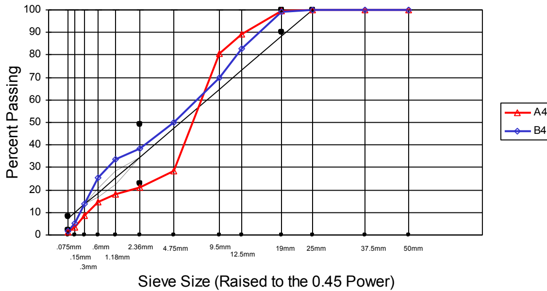
Figure C.108 Sieve analysis result from the 3 rd layer of NC-55
