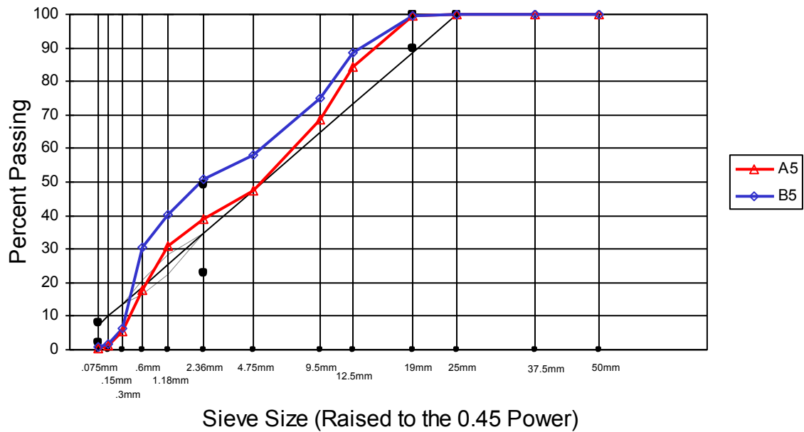
Figure C.33 Sieve analysis result from the 5 th layer of NC-87
