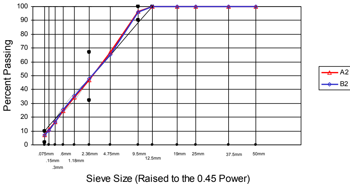
Figure C.85 Sieve analysis result from the 1 st layer of NC-194
