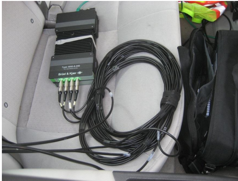
Figure 3.9 PULSE ® Analyzer in the Backseat of the Test Vehicle
