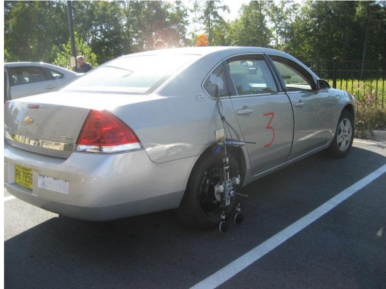
Figure 3.28 OBSI System Installed on the Test Vehicle Ready for Testing
