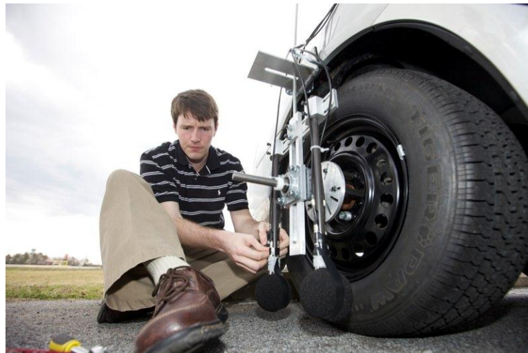
Figure 3.12 Installation of the OBSI System for the First Field Trial Testing
