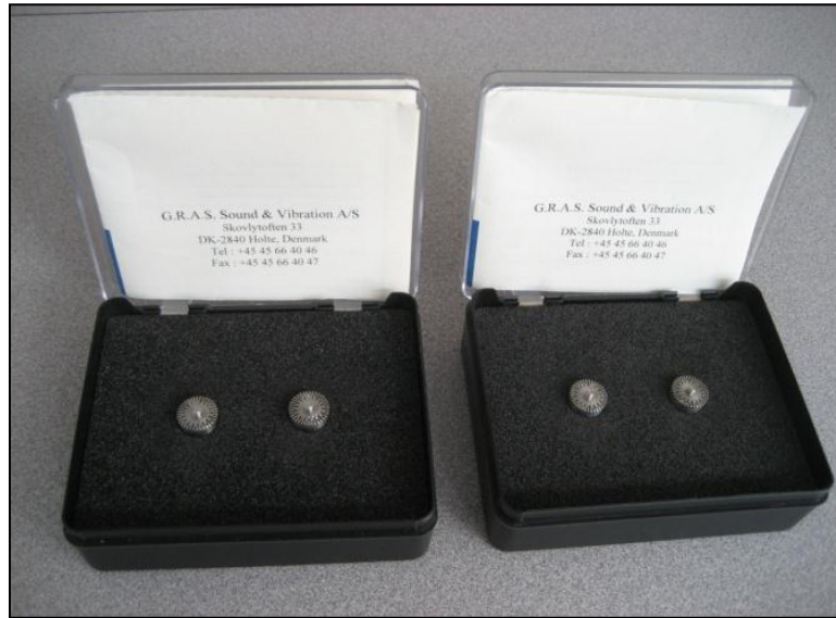
Figure 3.3 Two Pairs of G.R.A.S. ½ in. Microphones
