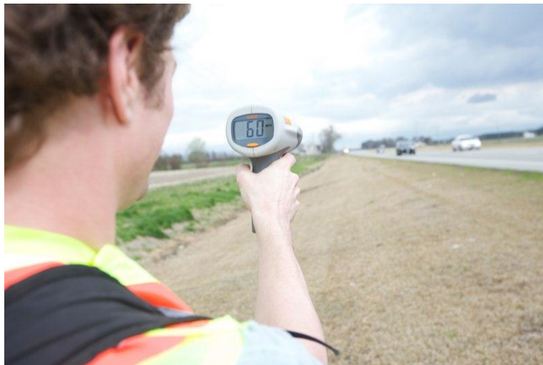
Figure 3.18 Checking the Driving Speed of Test Vehicle during the Trial Test
