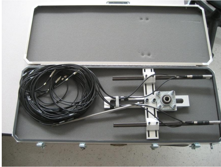
Figure 3.5 Microphones on the Fixture with 7-pin Cables in the Case
