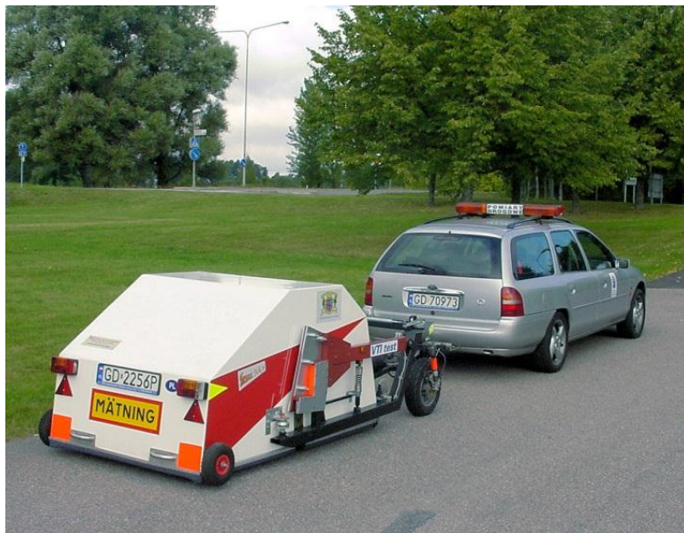
Figure 2.3 CPX Used By the Swedish National Road and Transport Research Institute
