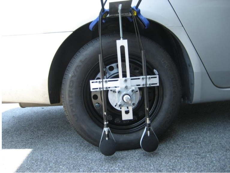
Figure 3.13 Microphones with Windscreens, Mounting Fixture and Cables
