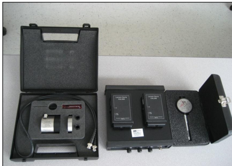
Figure 3.4 Calibration Equipment for Microphone, Sound Intensity and Tire
