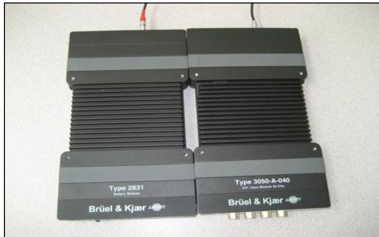
Figure 3.2 B&K PULSE® Type 3050-A-040 Analyzer and Battery
