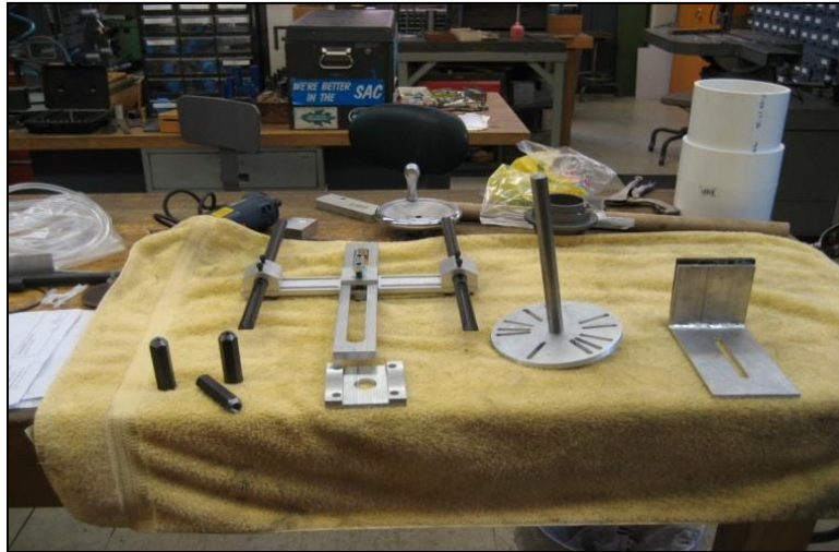
Figure 3.1 OBSI Microphone Mounting Fixture Parts Fabricated at ECU
