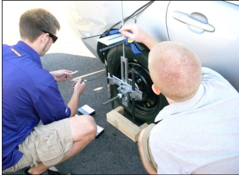
Figure 3.26 Checking the Positions of Microphones
