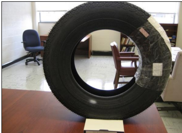
Figure 3.6 P225/60R16 Standard Reference Testing Tire (SRTT)
