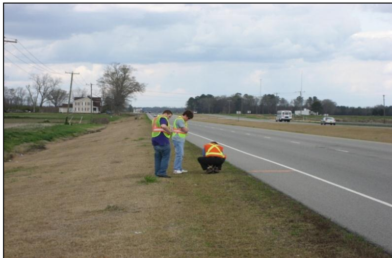
Figure 3.20 Laying-Out the 440 Feet Testing Section
