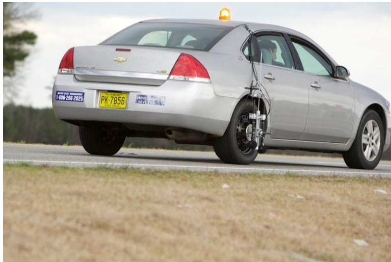
Figure 3.14 OBSI Test Vehicle and Microphone Mounting System
