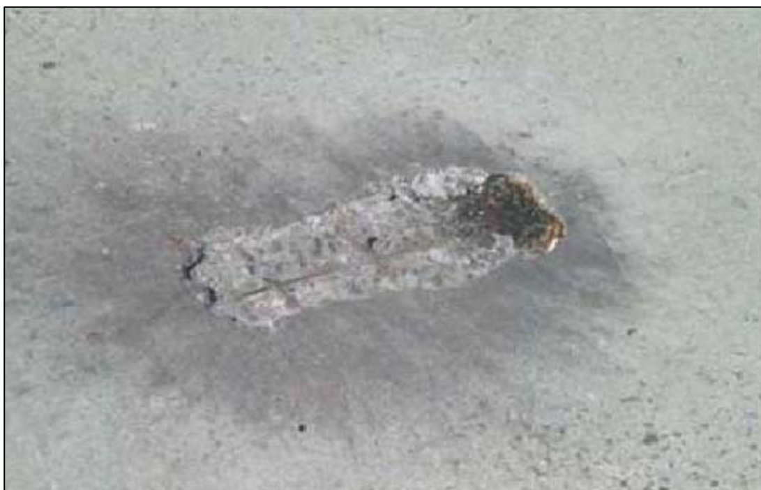
Exhibit 28: Concrete Pavement Spall
