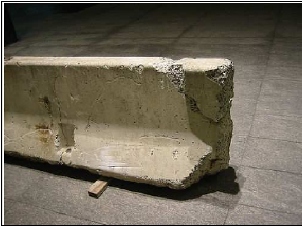
Exhibit 21: Damaged Concrete Barrier
