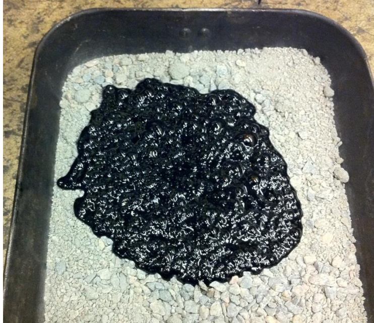
Figure 2-4 Foamed Asphalt Produced by “The Foamer”
