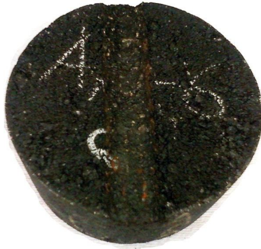
Figure 7-2 Rutted Specimen after Performing APA Test
