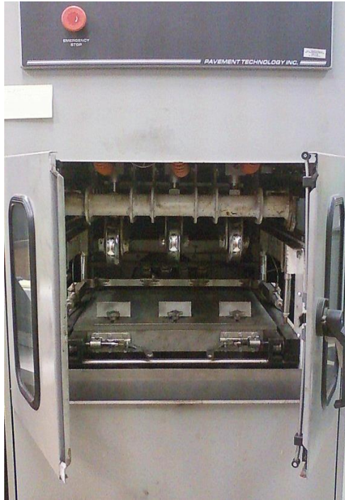
Figure 7-1 Asphalt Pavement Analyzer Used for Testing Rutting Susceptibility
