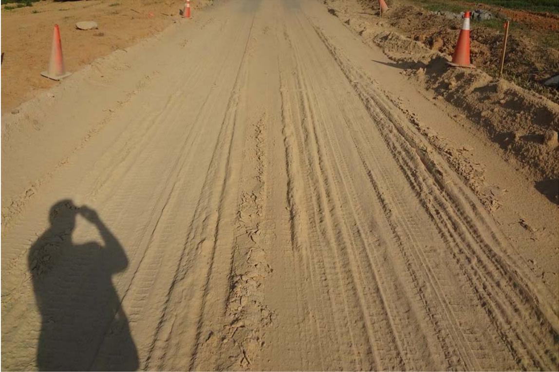
Figure 7-4. Test section 1, after 300 traffic passes.
