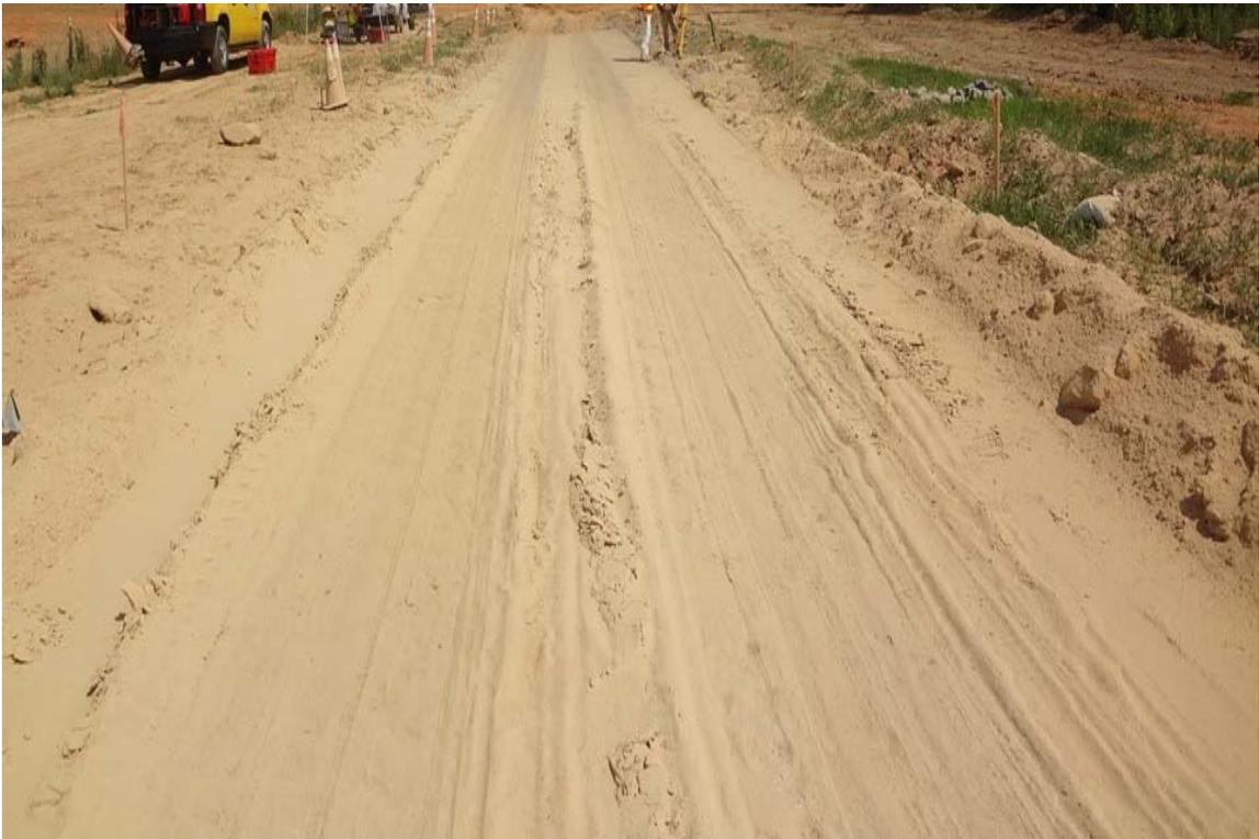
Figure 7-5. Test section 1, after 1000 traffic passes.
