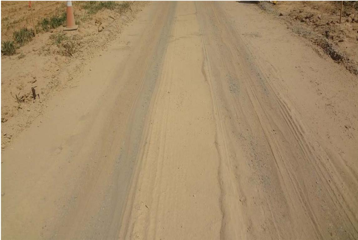
Figure 7-6. Test section 2, Geogrid reinforced, after 1000 traffic passes.
