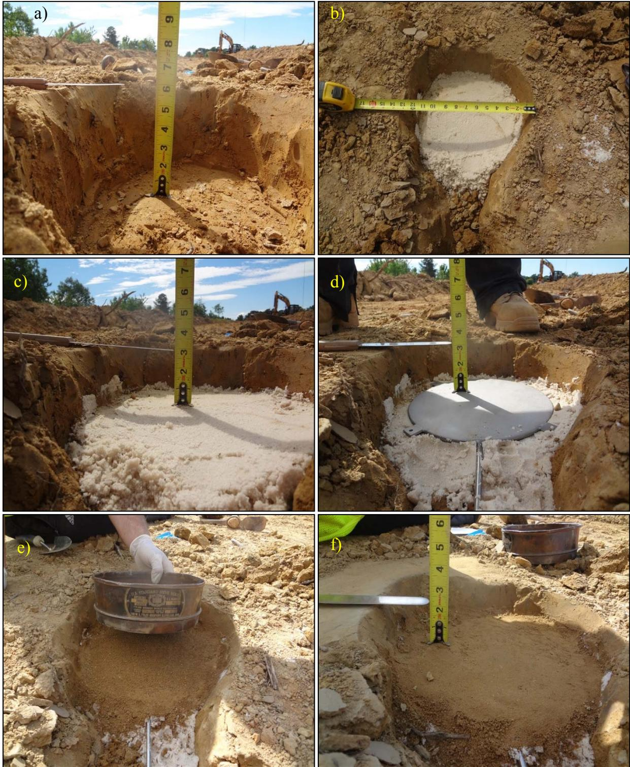
Figure 3-7. a) Depth of the EPC below the stabilized layer; b) 10”~11” hole; c, d) 3” hand-compacted silica sand; and e, f) 1” soil (fraction that passed sieve No. 10).
