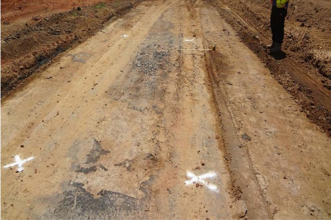
Figure 7-8. Test section 4, lime stabilized, after 10 traffic passes.
