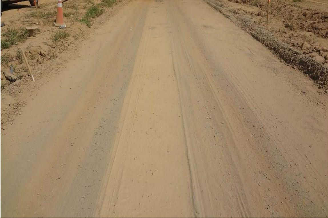
Figure 7-7. Test section 3, Geotextile reinforced, after 1000 traffic passes.
