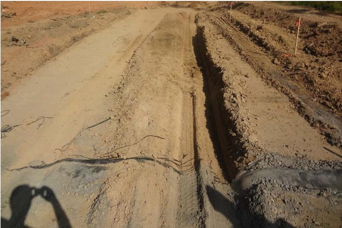
Figure 7-9. Test section 4, lime stabilized, after 100 traffic passes.
