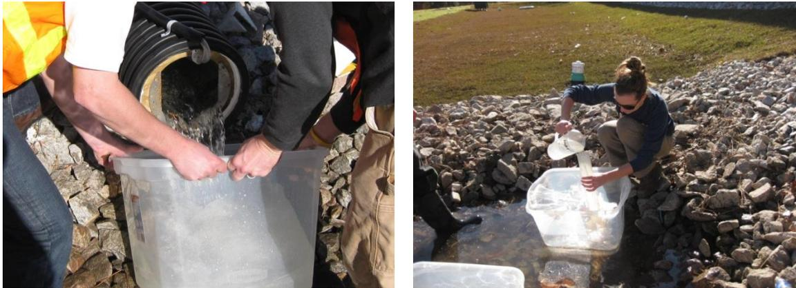
Figure 11. Timed water collection into bucket (left) and measurement of volume collected (right).
