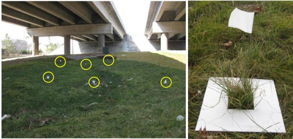
Figure 61. Flag placement in swale (left) and grass counting template (right).
