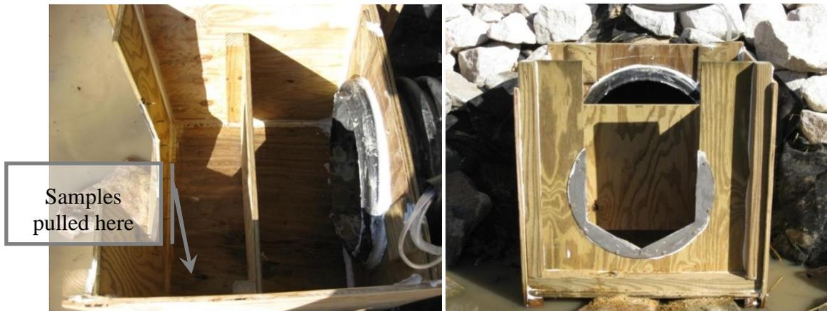
Figure 20. Baffled weir box at the outlet of the swale (top and front view).
