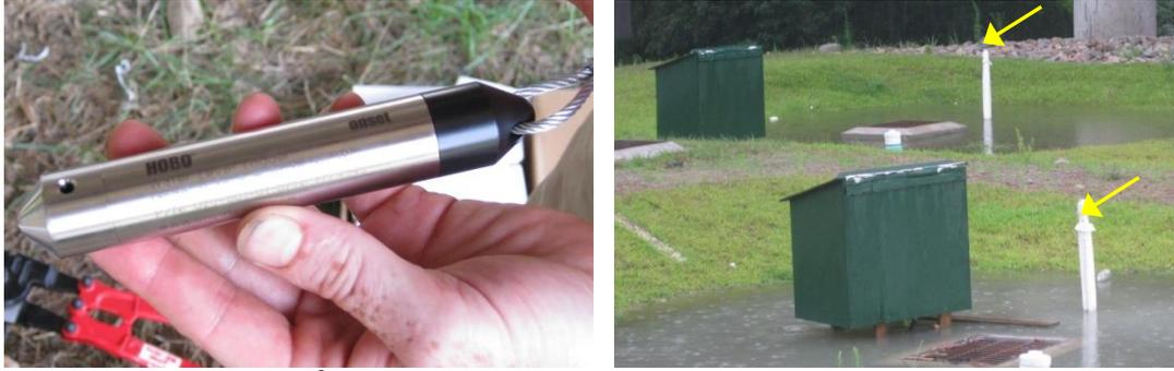
Figure 13. HOBO® water level logger (left) and installed wells at cell outlets (right).
