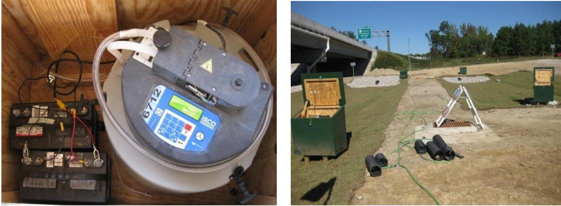
Figure 15. ISCO 6712™ portable sampler (left) and green housing boxes (right).
