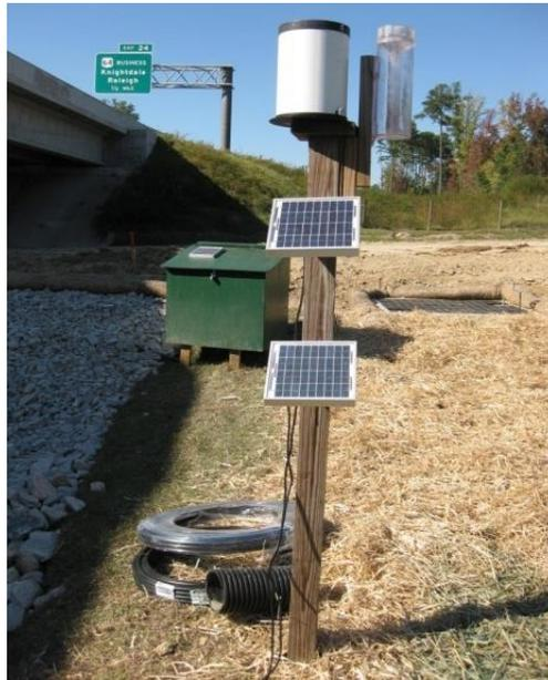
Figure 9. Manual rain gauge and ISCO 674 rain gauge.
