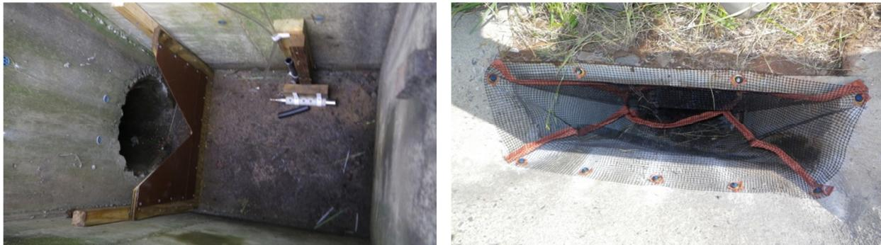
Figure 2. 90° weir and sampling intake at the Brevard site (at left) and monitoring gross solids at Black Mountain (at right).
