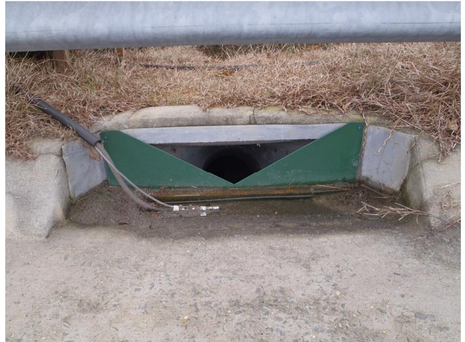
Figure A.5. Photos of the catchment (top left) and monitoring setup (left – roadway catchment; right - weir and sample intake) at Faison, NC particle size distribution monitoring location.
