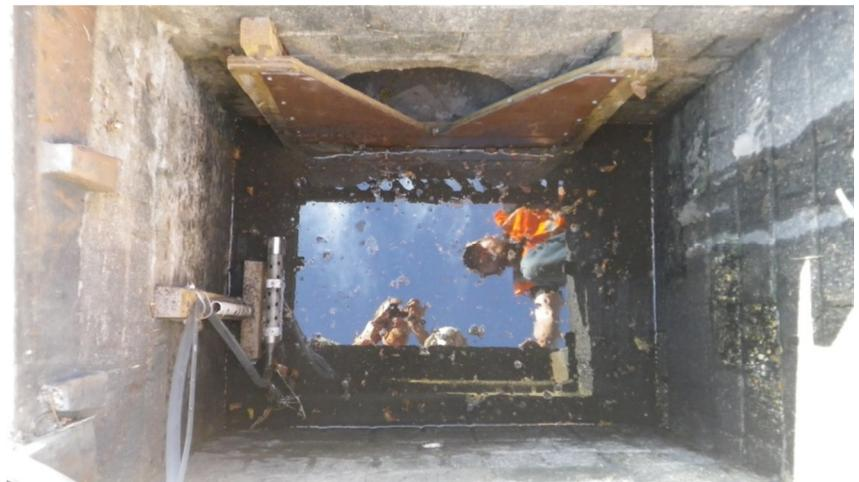
Figure A.7. Photos of the catchment (top left) and monitoring setup (right - sample intake in catch basin) at the Wilson, NC particle size distribution monitoring location.
