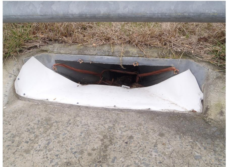
Figure A.9. Photos of the catchment (left) and monitoring setup (gross solids monitoring mesh in drain) at the Faison, NC gross solids monitoring location.
