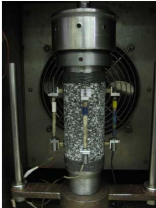
Figure 3.14 Direct tension fatigue test set-up.
