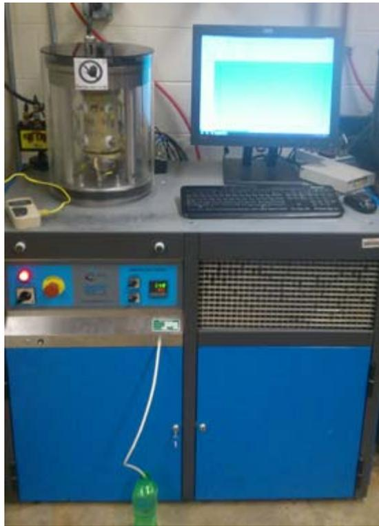
Figure 3.11 TRLPD test set-up with AMPT.
