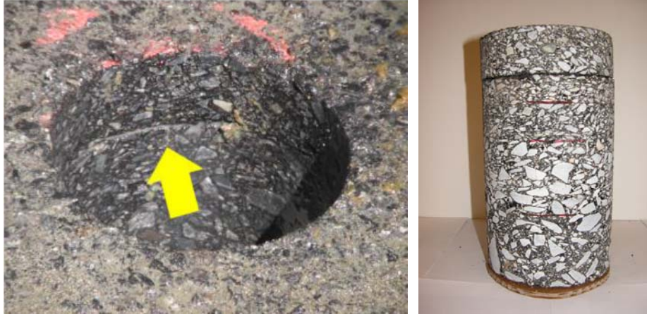
Figure A.2 Debonding (layer interface separation) in core-extracted hole (NC-24) (Park 2013).
