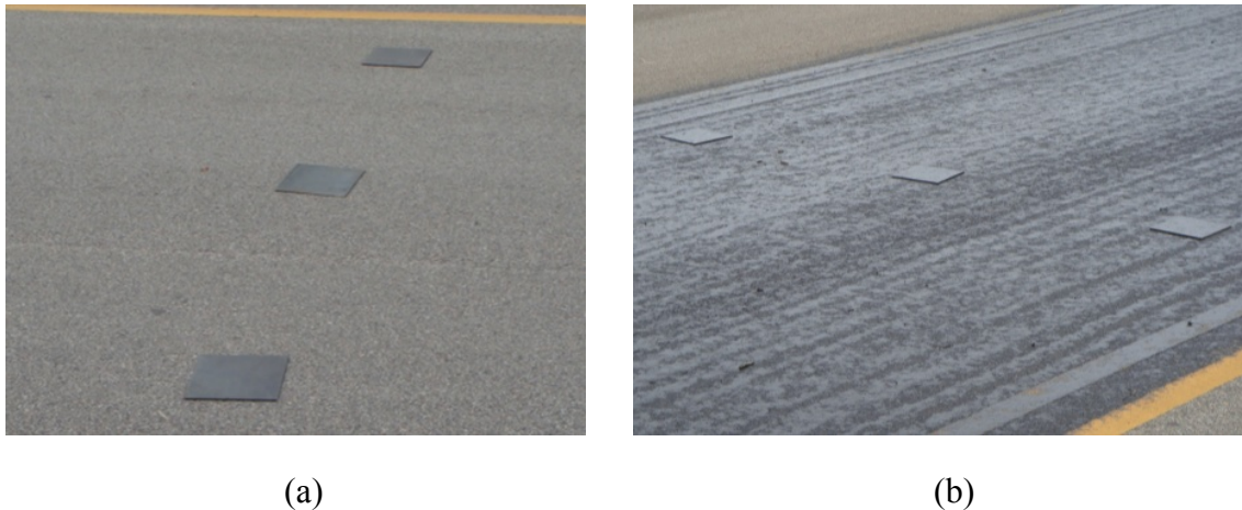
Figure C.21 Steel plates placed on the surface of asphalt pavement for measurement of tack coat application rate: (a) before tack coat application and (b) after tack coat application.
