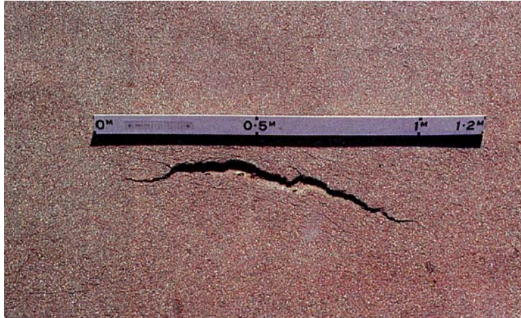
Figure A.5 Crescent-shaped slippage crack (National Association of Australian State Road Authorities 1987).
