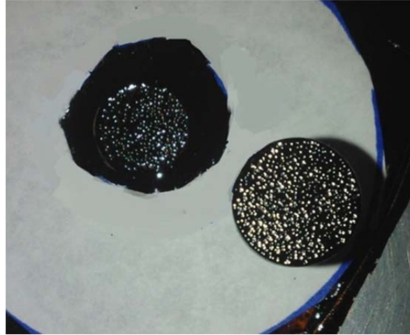
Figure 4-7 Failure mode of the PATTI test samples (i.e., cohesion failure of the emulsion).
