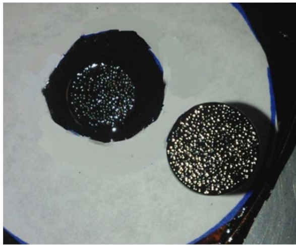
Figure D.59 Failure mode of the PATTI test samples (i.e., cohesion failure of the emulsion).
