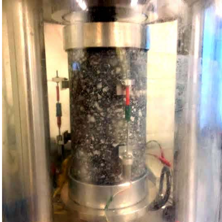
Figure 6.2 Typical Setup of Test Specimen
