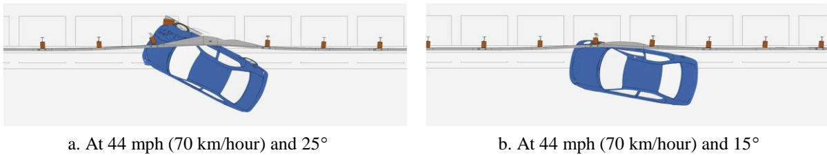
Fig. 4.28: Permanent deformation of the 31-inch guardrail at the curb face and impacted by a Dodge Neon.
