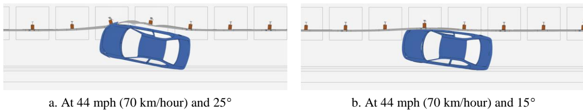
Fig. 4.76: Permanent deformation of the 29-inch guardrail at 6 feet from the curb face and impacted by a Dodge Neon.
