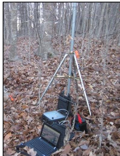
Figure 3. Telemetry tower setup with two 9-element yagi antenna and datalogging receiver at the base.
