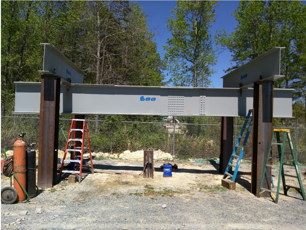
Figure B-17: Photo of reaction frame with load beam over H-pile.
