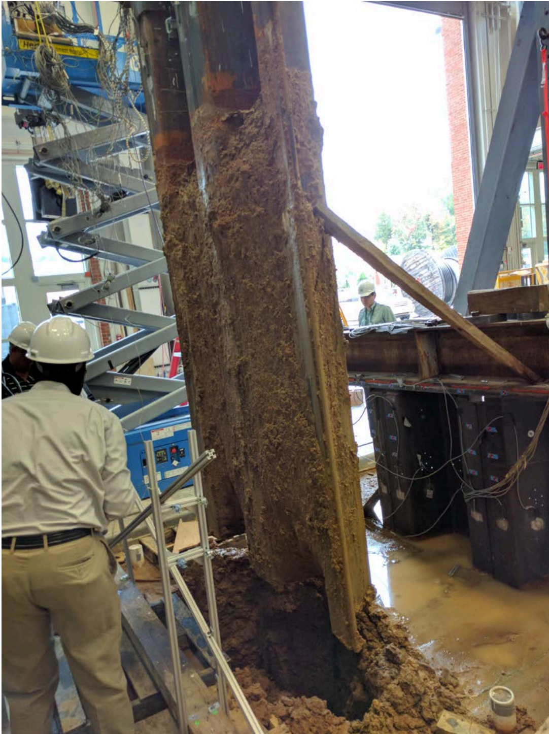
Figure 3-28: Photo showing soil plugging along the embedment depth of the sheet pile wall.
