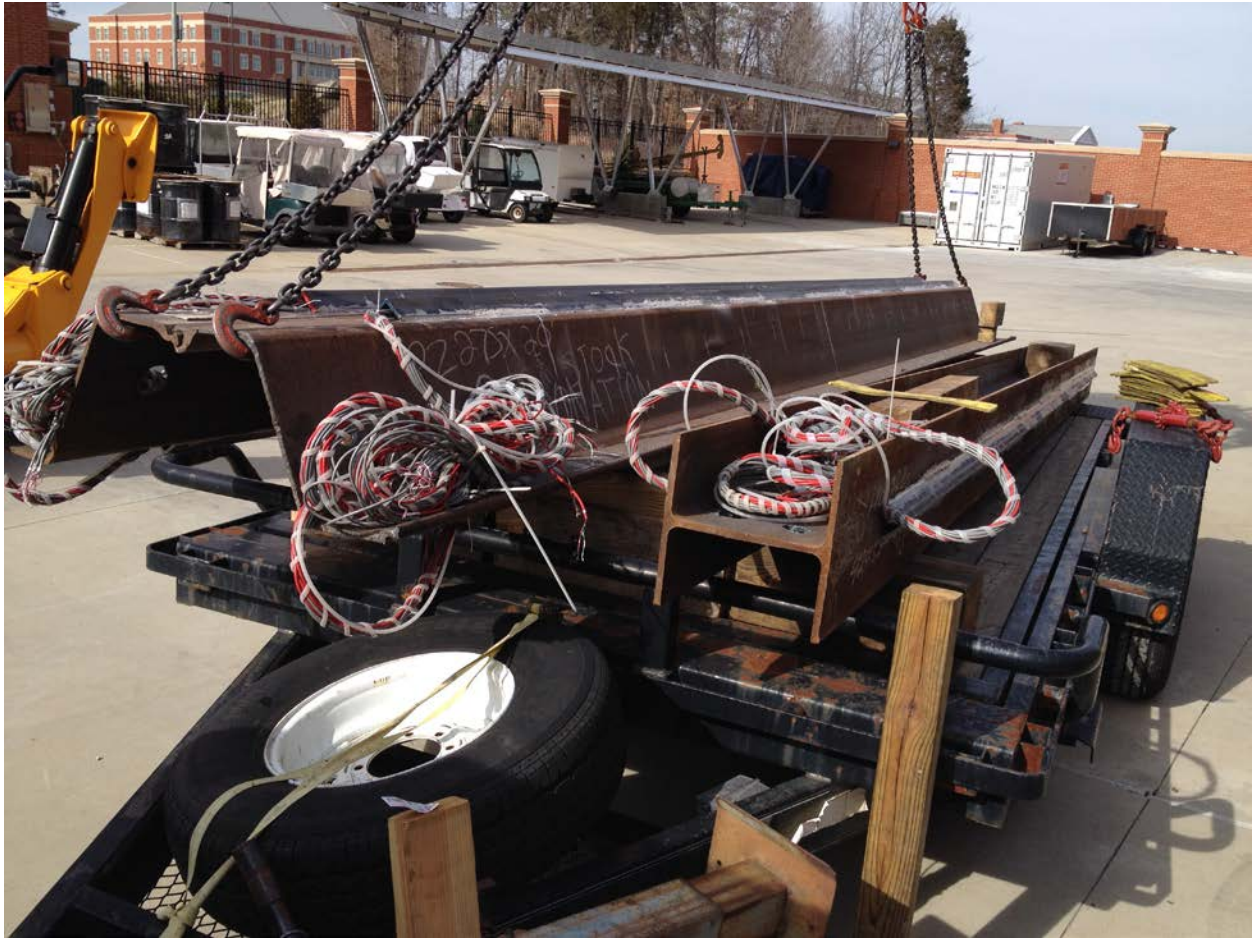
Figure 4-7: Photo of instrumented test piles delivered at field site.
