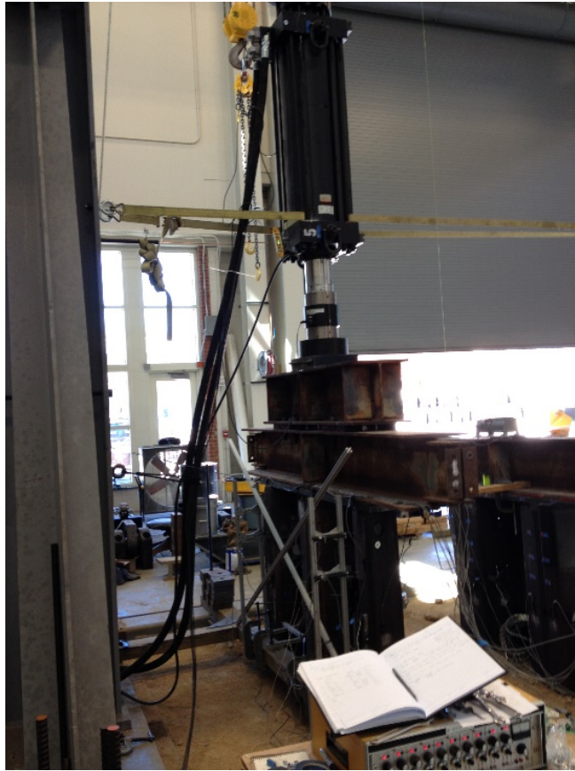
Figure 3-15: Load distribution beam assembly used for axial load tests.
