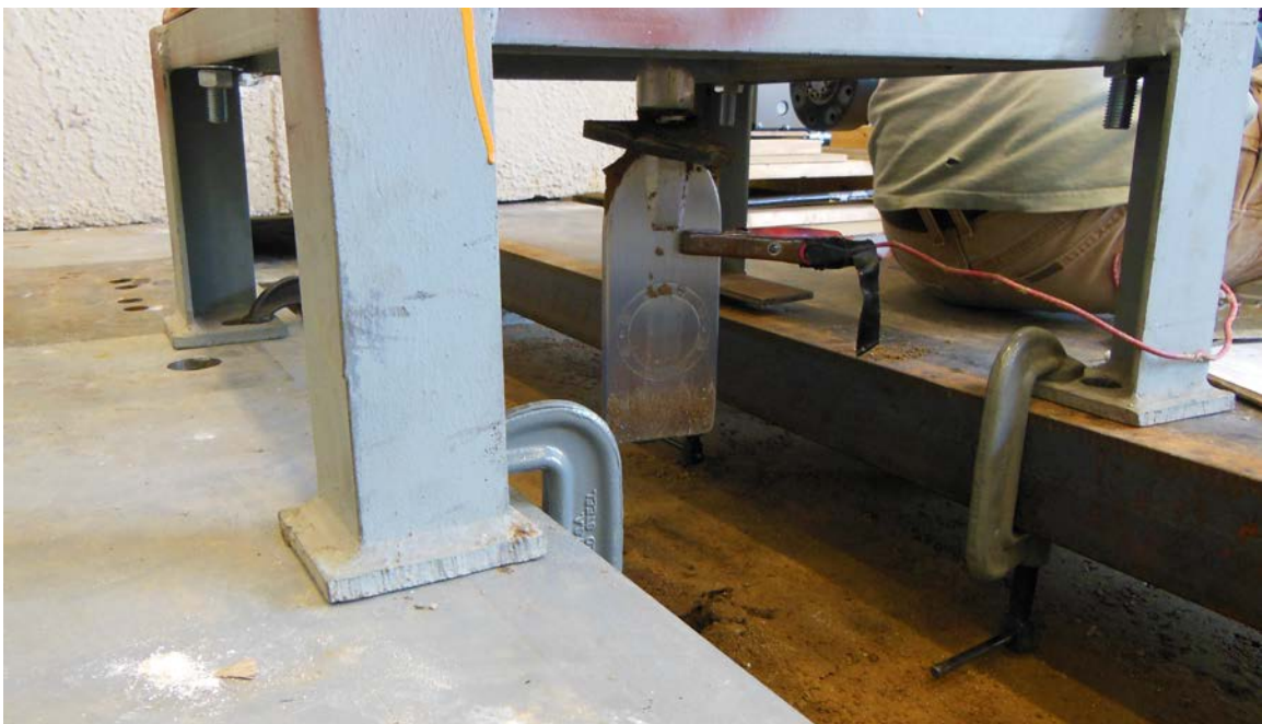
Figure A-8: Photos of DMT testing prior to sheet pile installation.
