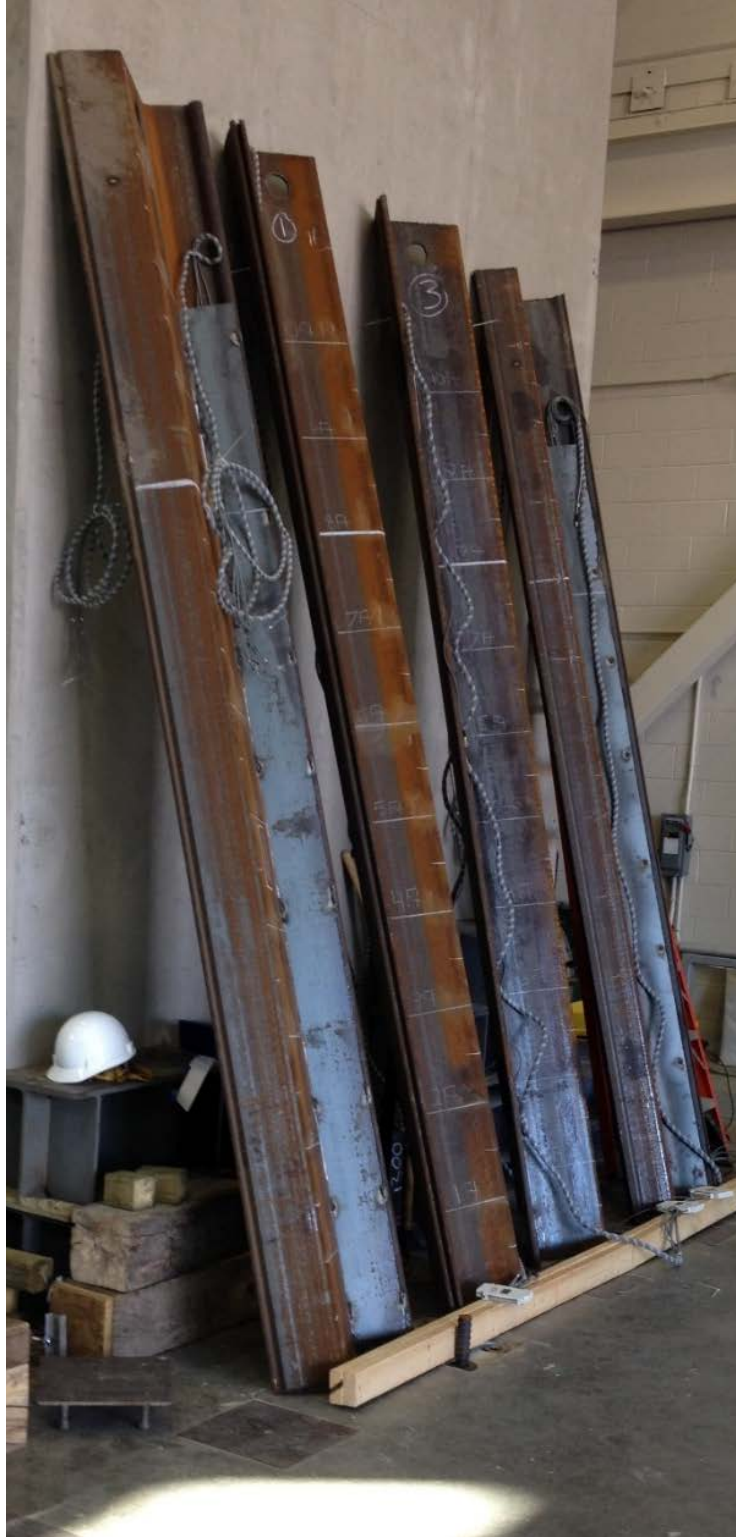
Figure 3-10: Photo of 12-ft length sheet pile sections used in laboratory load testing program.
