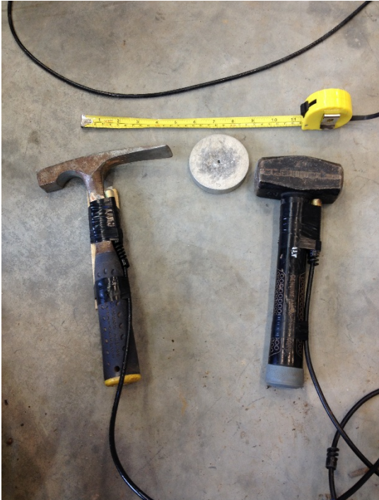
(a) Hammers used for MASW testing
