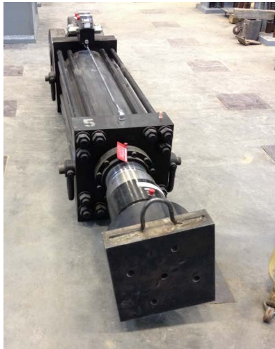
Figure 3-16: Photo of MTS actuator (328-kip capacity in compression).
