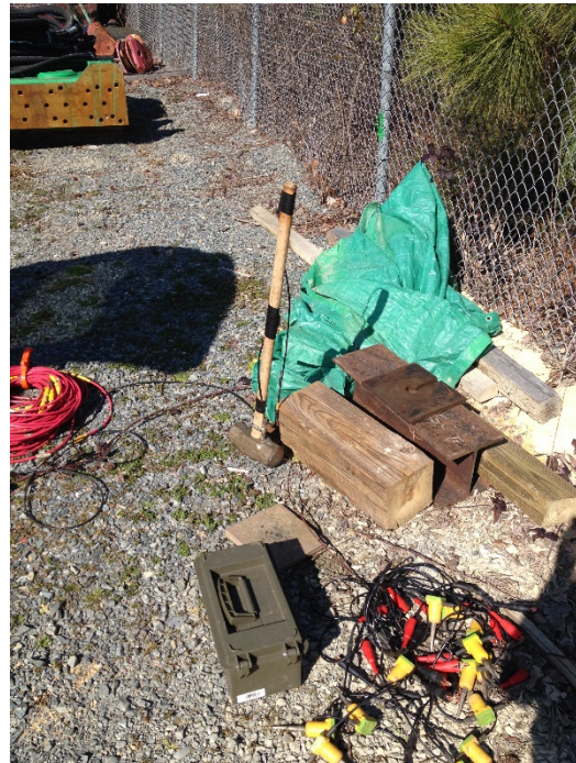
(b) MASW seismic source
