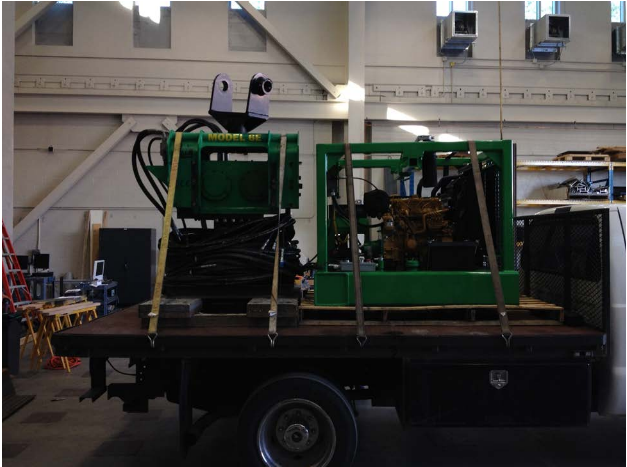
Figure A-17: Photo of ICE 6E vibratory hammer used at UNCC High bay.
