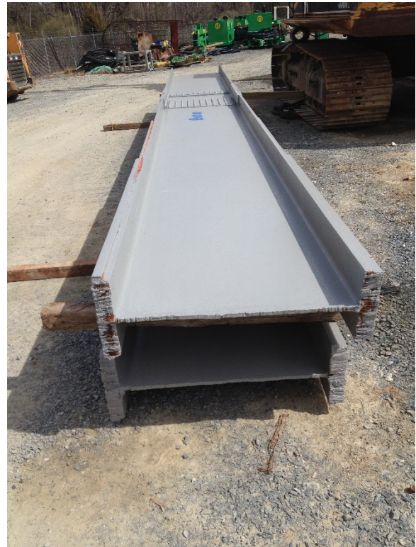
(b) Beams for reaction frame
