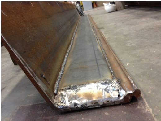
(c) Welding for sensor protection
