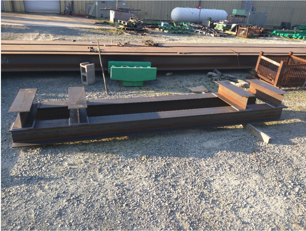
Figure B-15: Photo of reaction pile installation guide frame.
