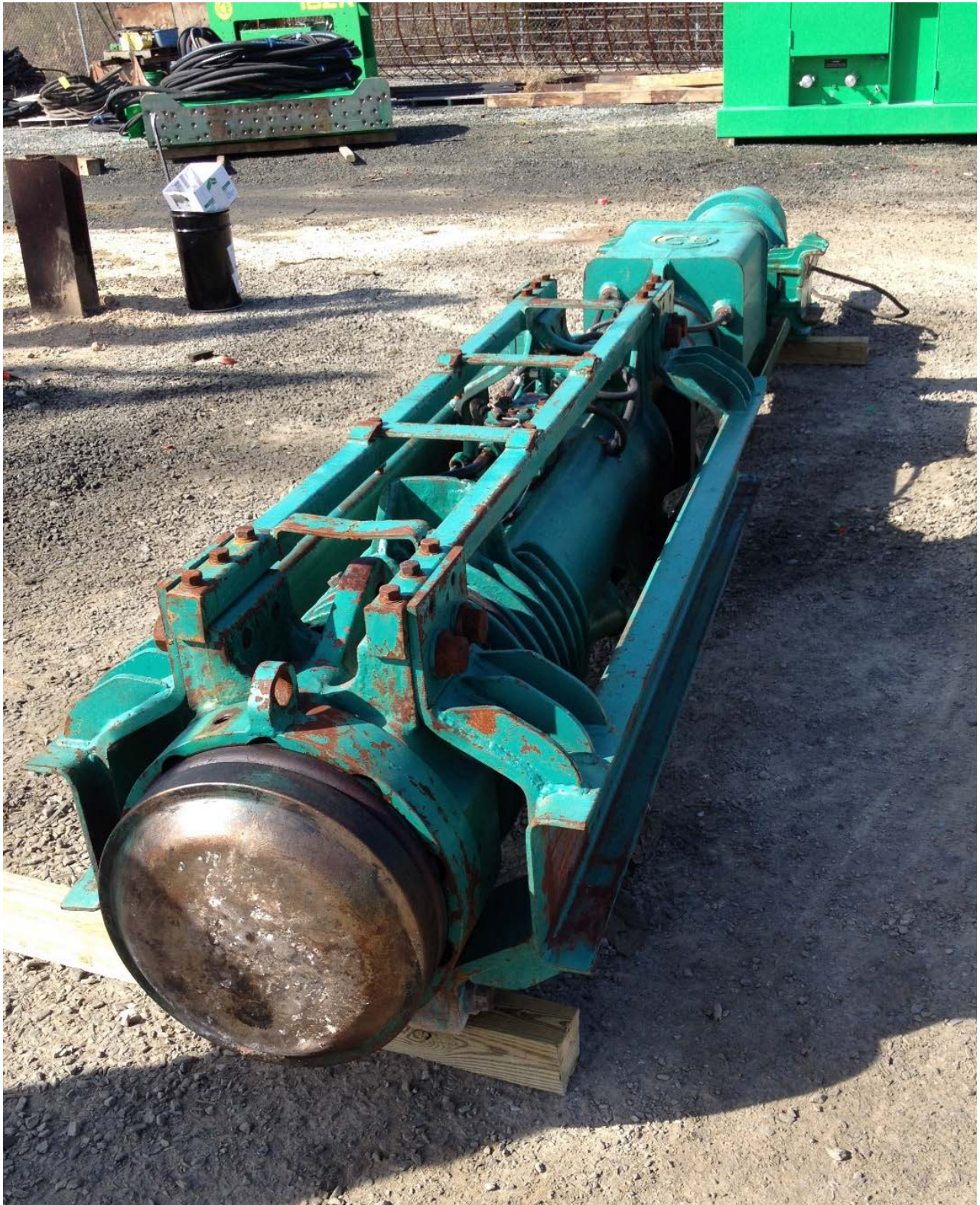
Figure 4-9: Photo of single-acting diesel hammer ICE I-12 used for final pile installation.
