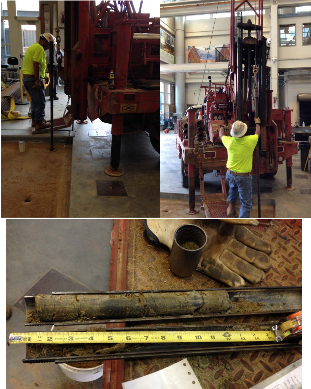
Figure A-6: Photos of geotechnical drilling with SPT testing by S&ME (Charlotte office).
