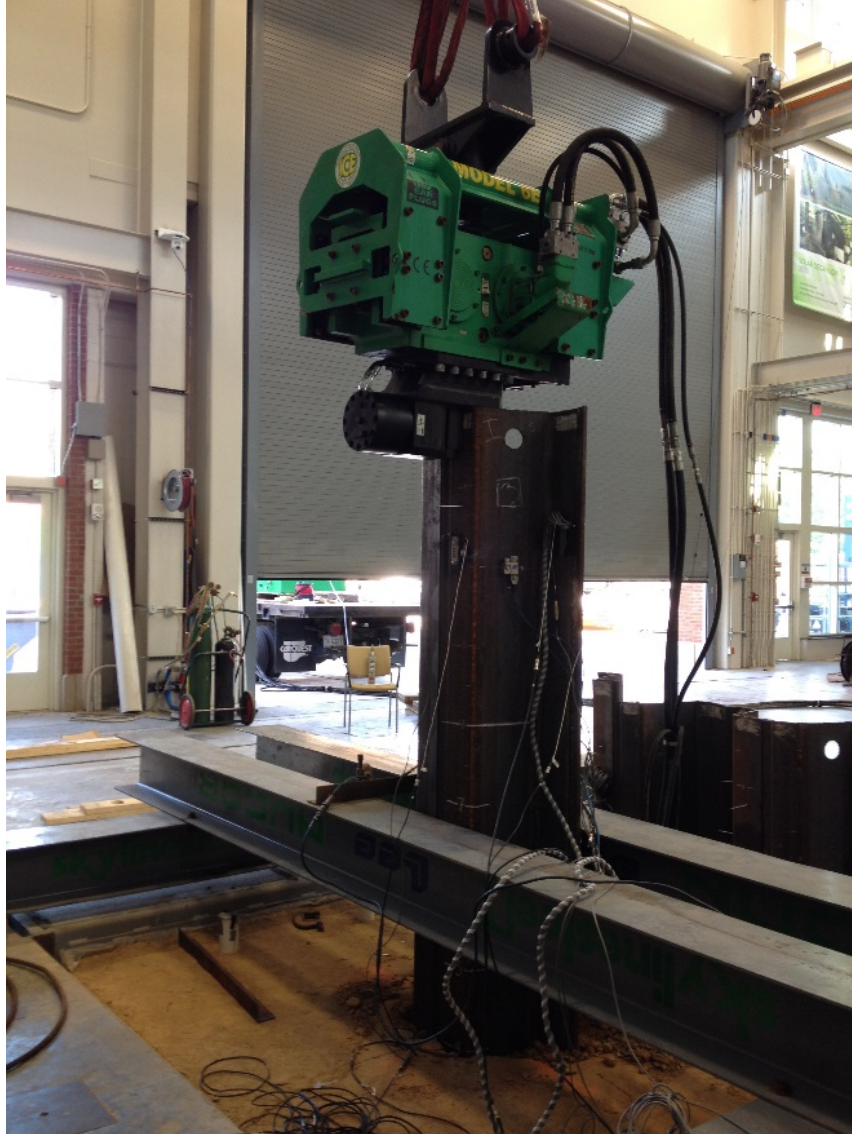
Figure A-18: Driving with ICE Model 6E vibratory hammer.
