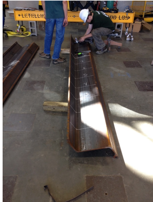
(b) Marking piles for sensors
