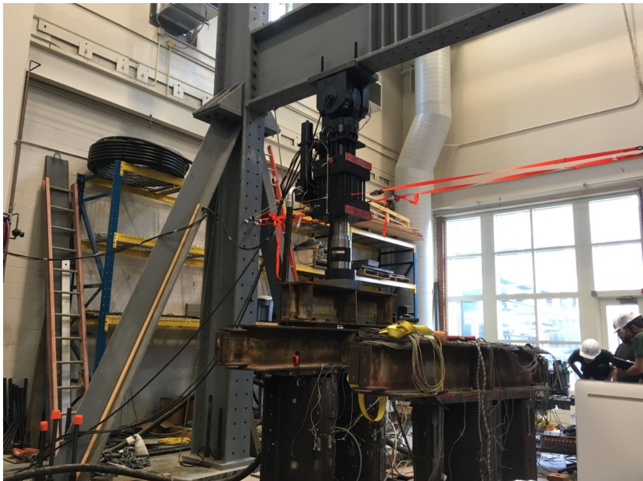
Figure 3-14: Axial load test setup.
