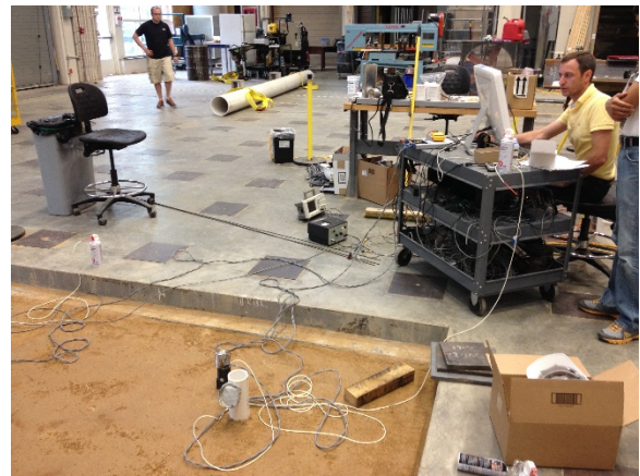
(c) Observing crosshole data and modifying computer program
