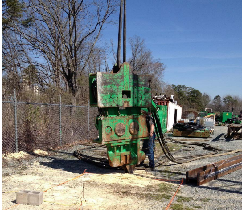
(a) ICE 28C vibratory hammer
