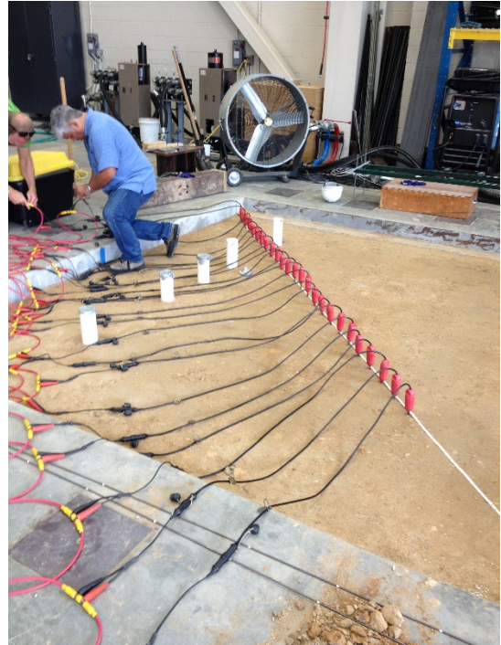
(b) MASW testing
