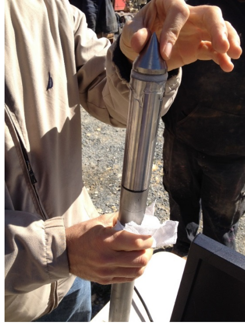
(b) SCPTu cone with saturated porous element around pore pressure sensors
