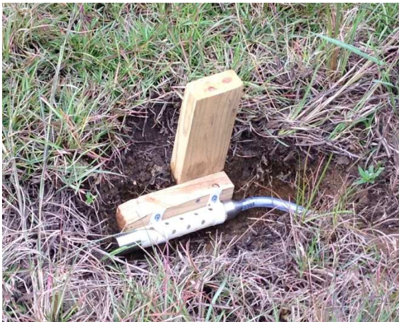
Figure 4-13: A sampler intake strainer set up for monitoring at the I-40 swale inlet (left) and a view of the sampler intake during a storm event (right).
