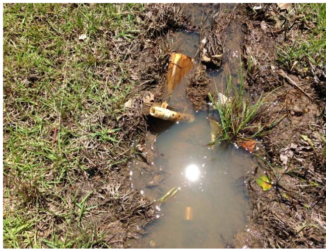
Figure 4-28: Damage to the inlet sampler head from a mower.
