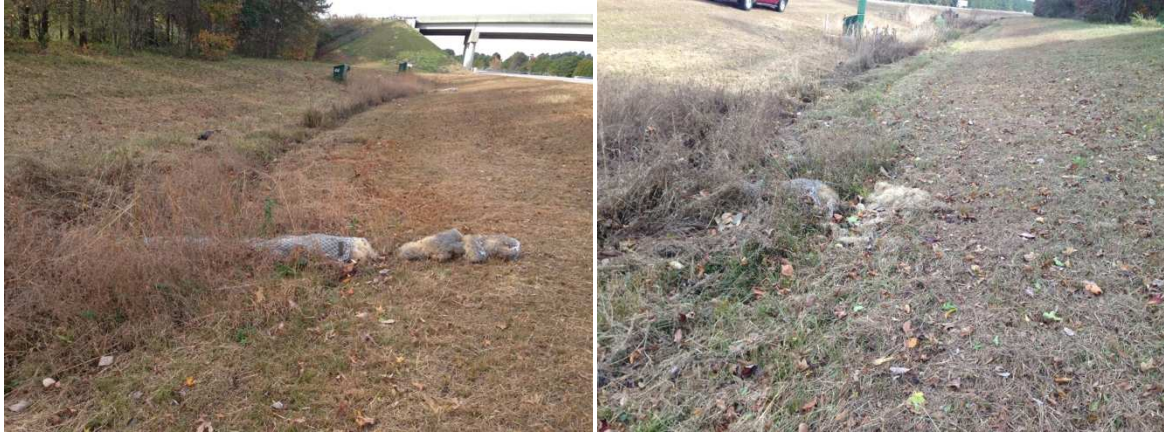
Figure 4-27: Photographs of damage to wattle check dams from mowers.
