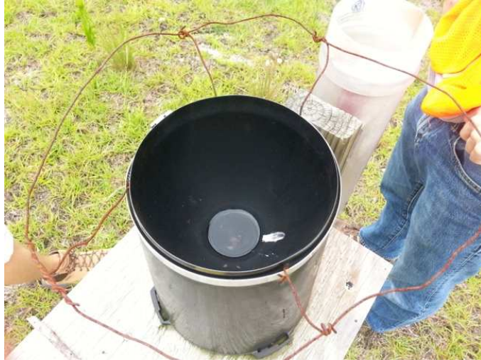
Figure 4-18: ISCO 674 rain gauge bucket clogged due to bird feces.
