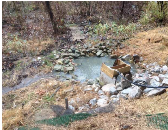
Figure 4-12: Mango Creek outlet monitoring point showing ISCO sampler housing and weir box (top left), weir box from above with baffle placed inside (top right), outlet weir during a storm event (bottom).
