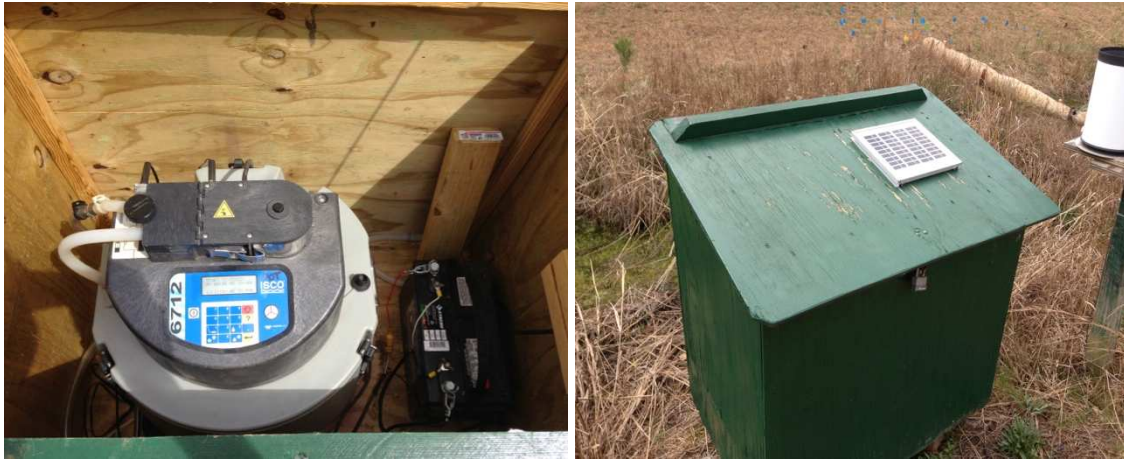
Figure 4-9: ISCO 6712 automated sampler and a 12-volt deep cycle battery in housing (left) and a mounted 5-watt solar panel (right).
