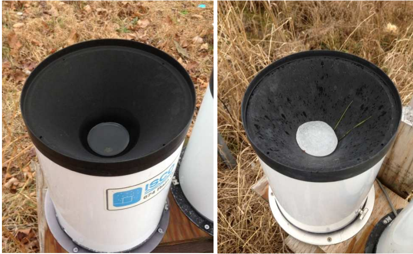
Figure 4-29: ISCO 674 rain gauges clogged from bird feces (left) and from frozen precipitation (right).
