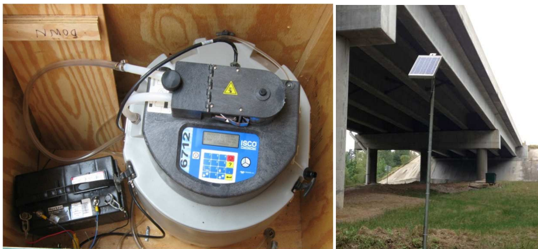
Figure 4-5: ISCO 6712 automated sampler and a 12-volt deep cycle battery in housing (left) and a mounted 20-watt solar panel (right).
