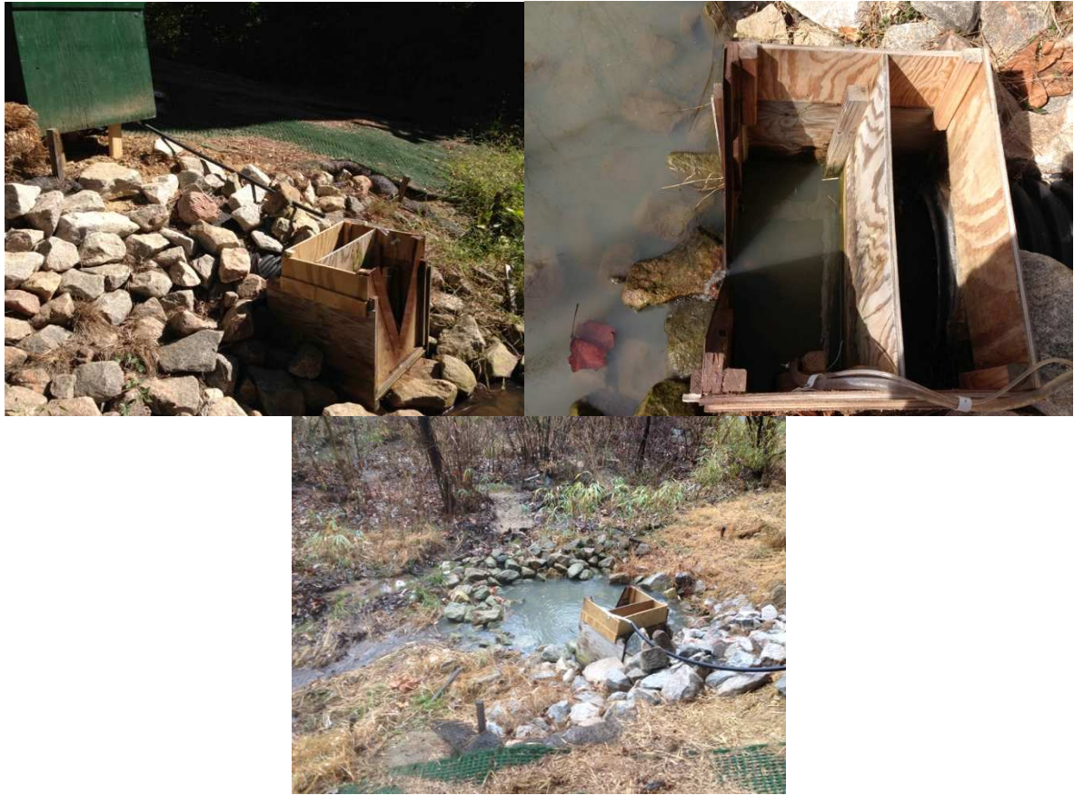
Figure 4-8: Clockwise from top left: Mango Creek outlet monitoring point showing ISCO sampler housing and weir box, weir box from above with baffle placed inside, and the outlet weir during a storm event.
