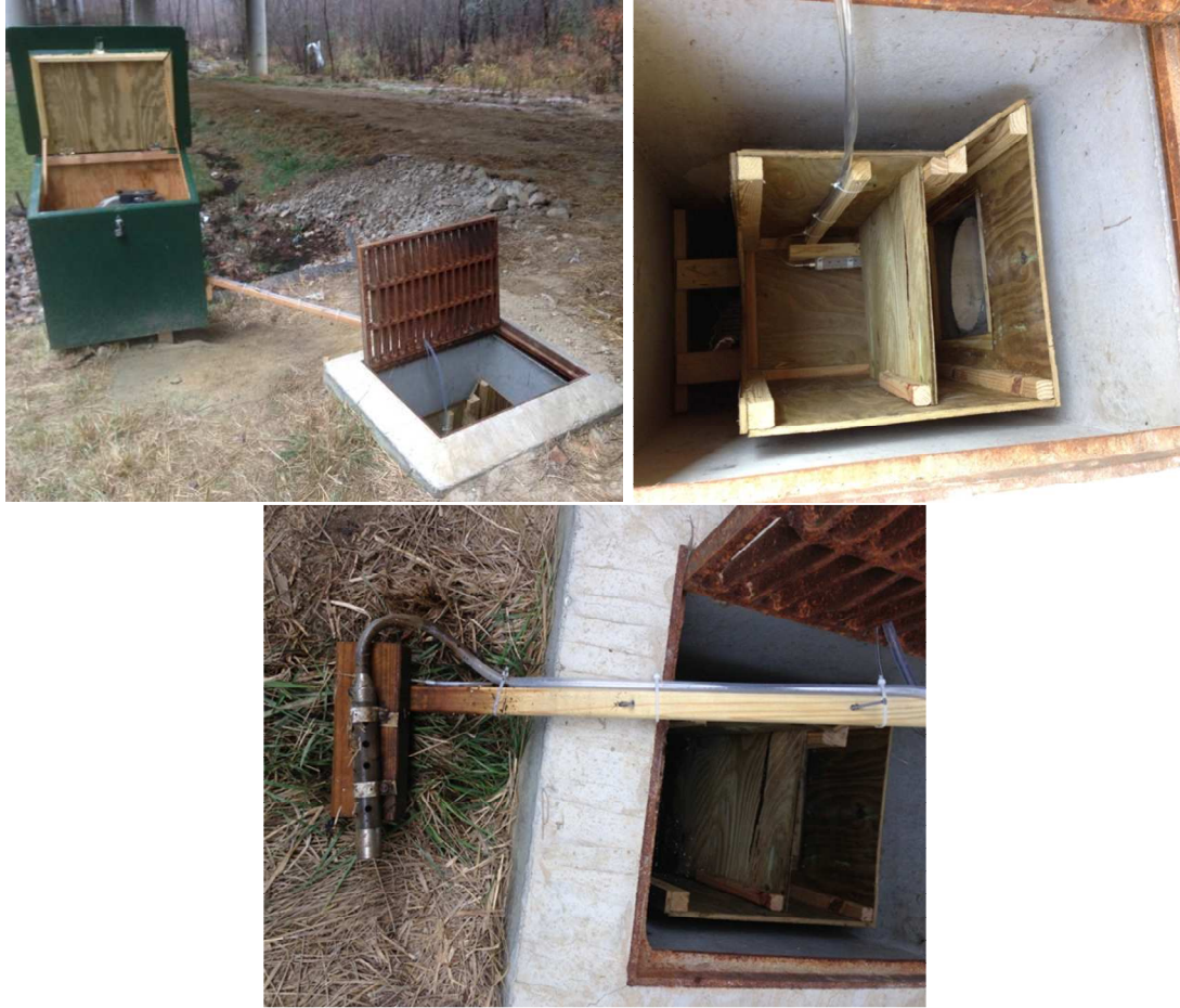
Figure 4-11: Mango Creek inlet monitoring point showing ISCO sampler housing and catch basin (top left), weir box with baffle placed within the catch basin (top right), and the mounted sampler intake with a bubbler attachment for detecting flow rates.
