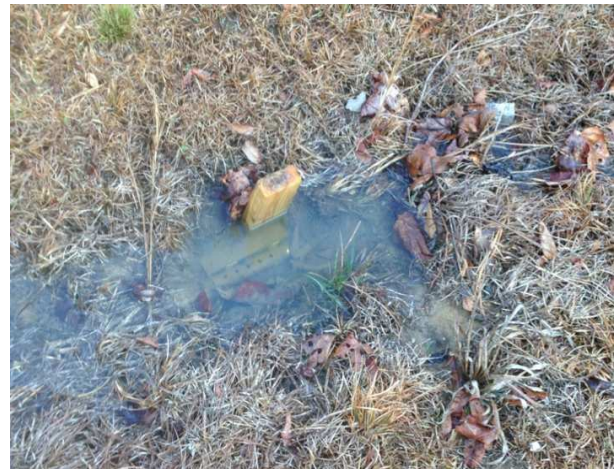
Figure 4-13: A sampler intake strainer set up for monitoring at the I-40 swale inlet (left) and a view of the sampler intake during a storm event (right).
