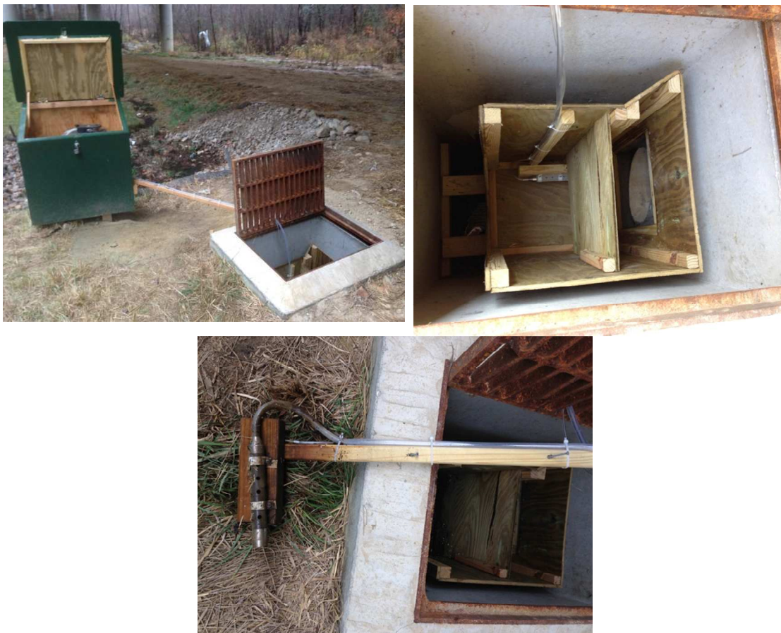
Figure 4-7: Clockwise from top left: Mango Creek inlet monitoring point showing ISCO sampler housing and catch basin, weir box with baffle placed within the catch basin, and the mounted sampler head with a bubbler attachment for measuring flow rates.
