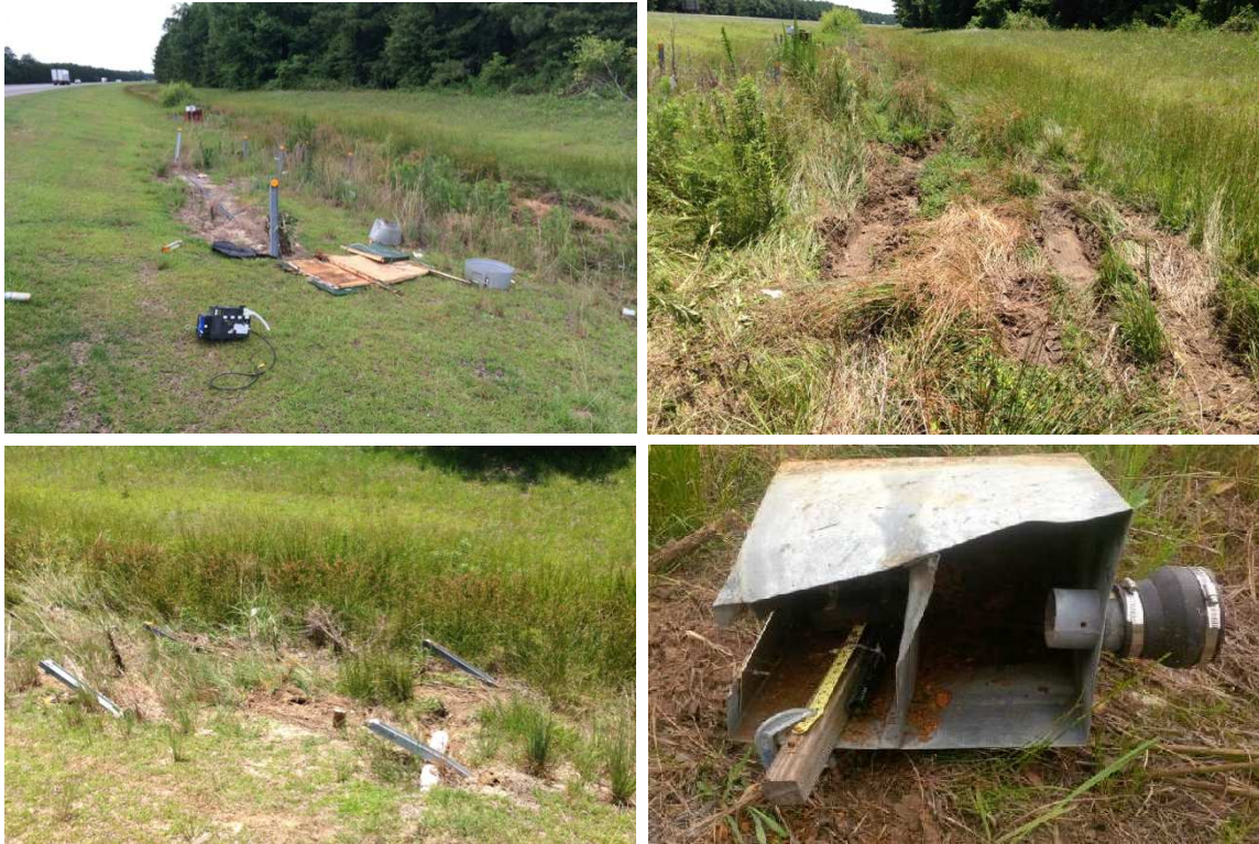
Figure 4-25: Clockwise from top left: Job box housing and ISCO 6712 sampler remains from vehicle incident on June 28, 2014, rut damage in the swale, the damaged weir box from the Road Runoff sampling point, and bent steel reflector beams.
