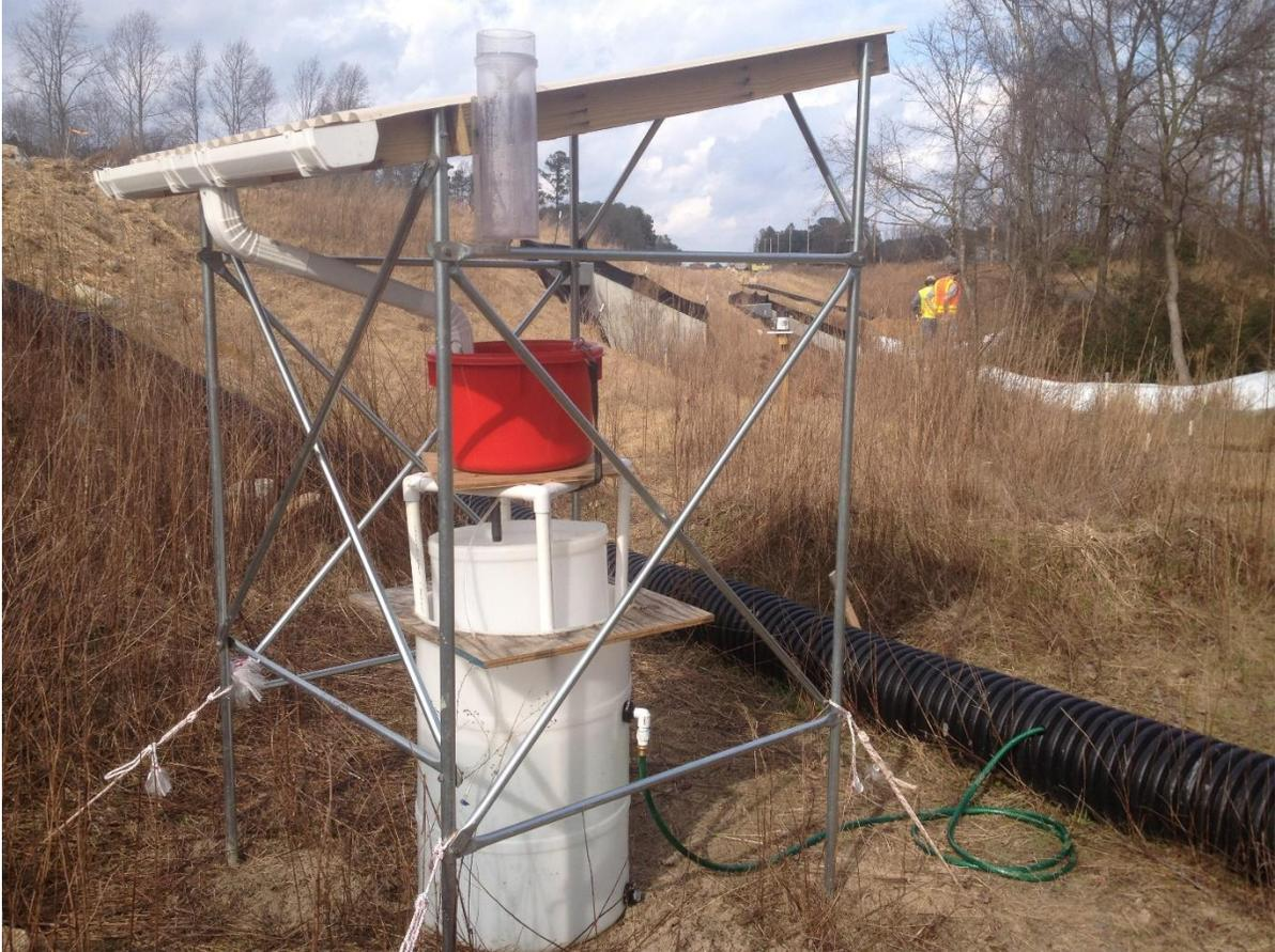
Figure 12. Modified New Zealand dosing system deployed in the field. The system is dosing a slope drain prior to a small sediment basin.
