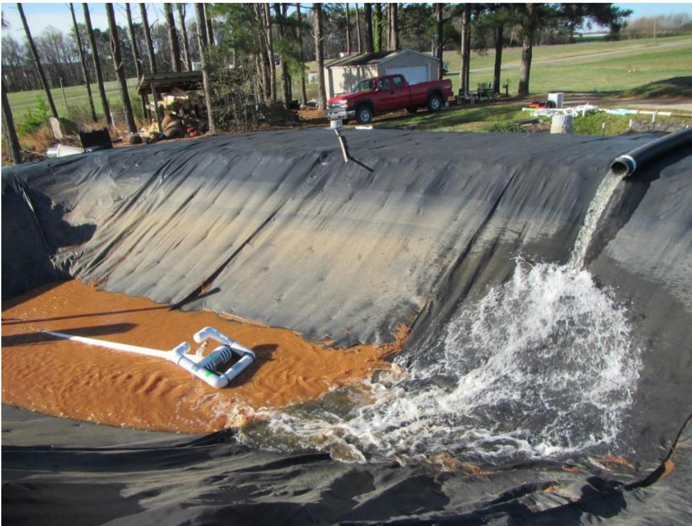
Figure 2. Faircloth skimmer at the beginning of a test.
