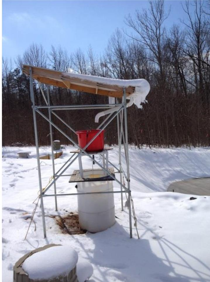
Figure 31. Rainfall driven liquid PAM dosing device (NZ Doser) installation in the foreground with skimmer basin (background right) and float valve doser (background left) at the Greensboro test site.
