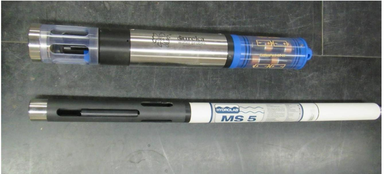
Figure 1. The two sondes tested during this project: Eureka Manta 2 (top) and Hach Hydrolab MS 5 (bottom).
