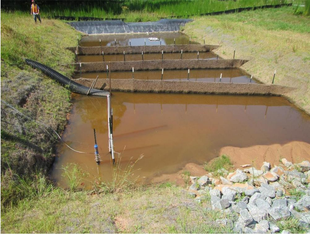
Figure 16. Turbidity measurement testing site in Durham showing the two sondes, stage samplers, and automatic sampler intake tubing.
