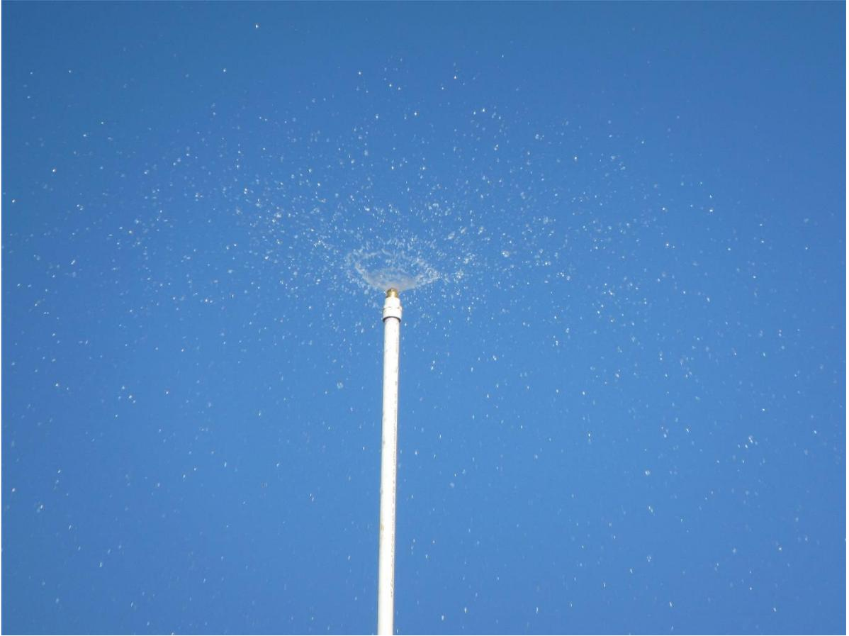
Figure 7. Closeup view of droplet distribution from one nozzle.
