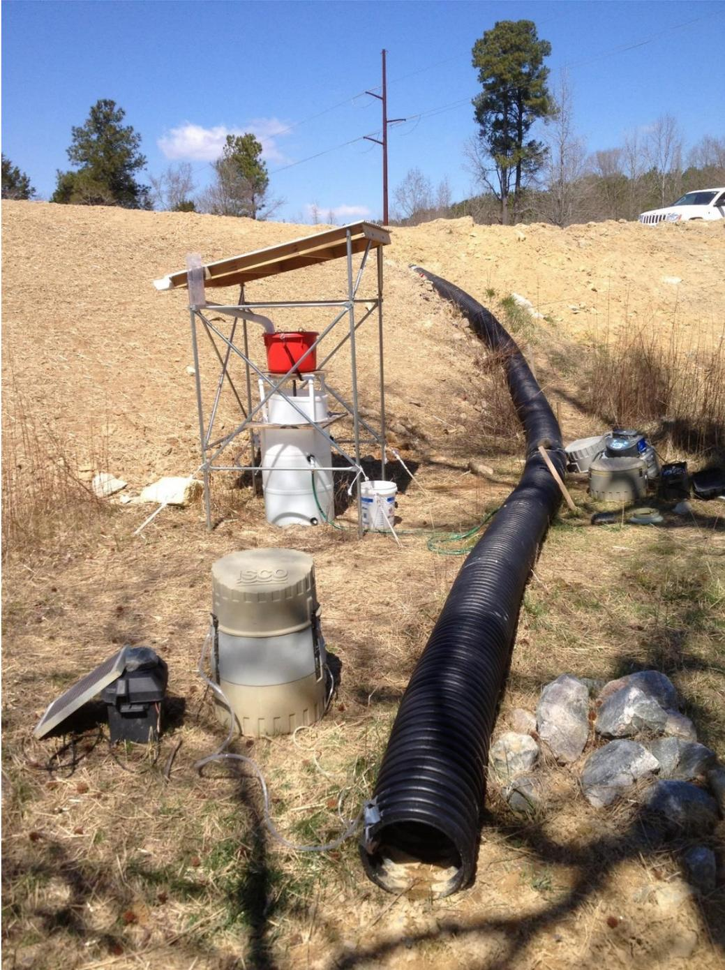
Figure 26. NZ Doser installed at the Rolesville 401 Bypass site. Slope drain brings water from the road bed to a small skimmer basin.
