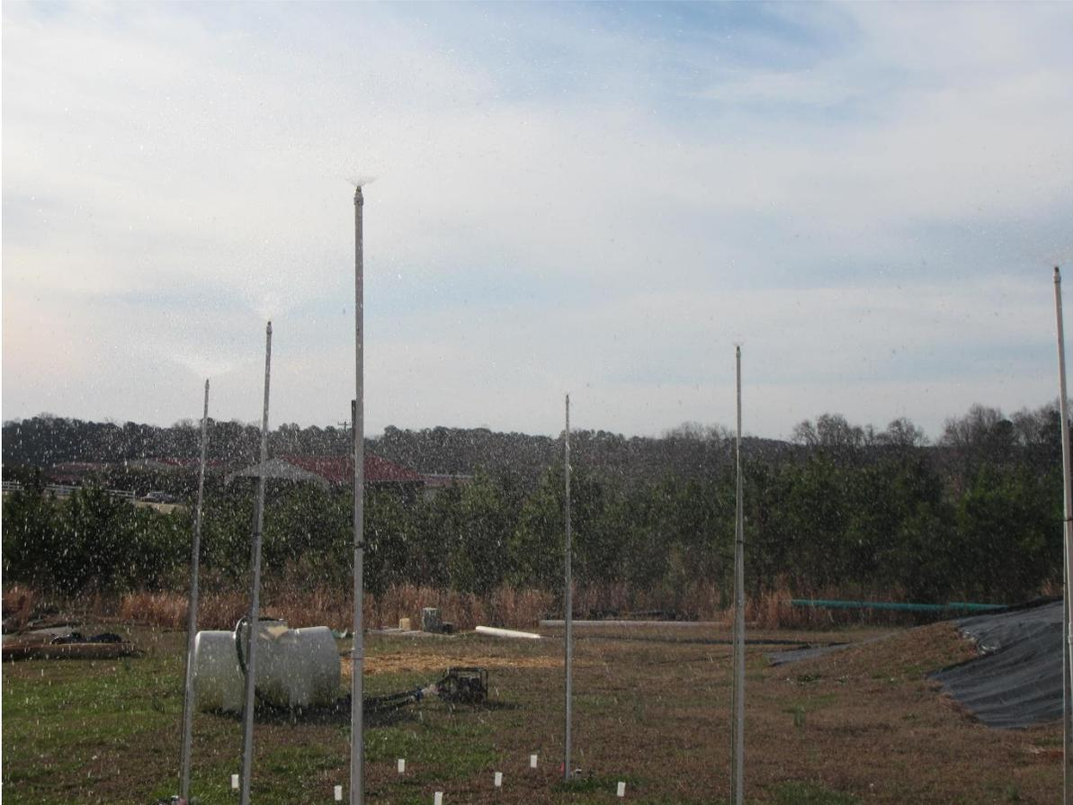
Figure 10. View of the rainfall distribution for the simulator. Pump and reservoir tank are shown beyond the simulator.
