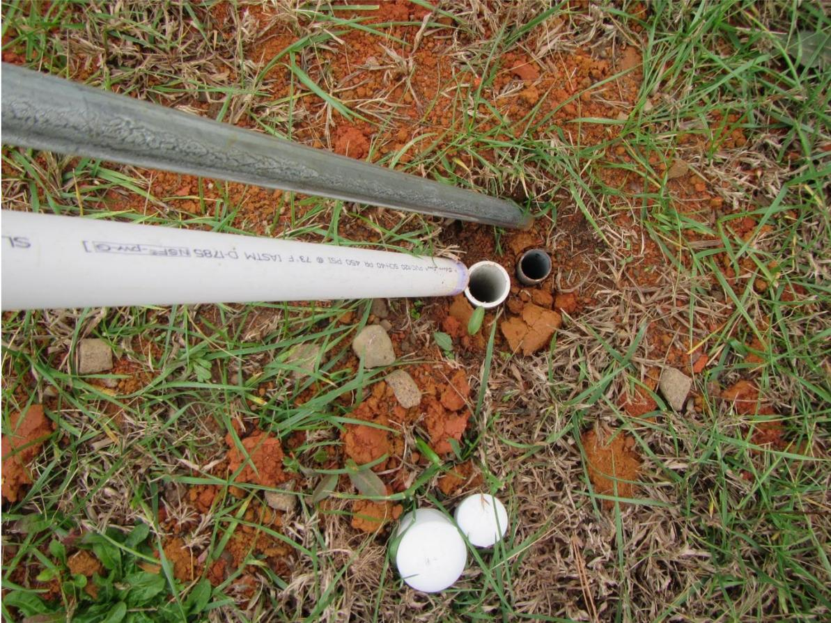
Figure 9. Support pipes inserted flush with the ground so when the simulator nozzle system is removed the grass can be mowed. Metal pipe serves as addition support for the PVC pipe.
