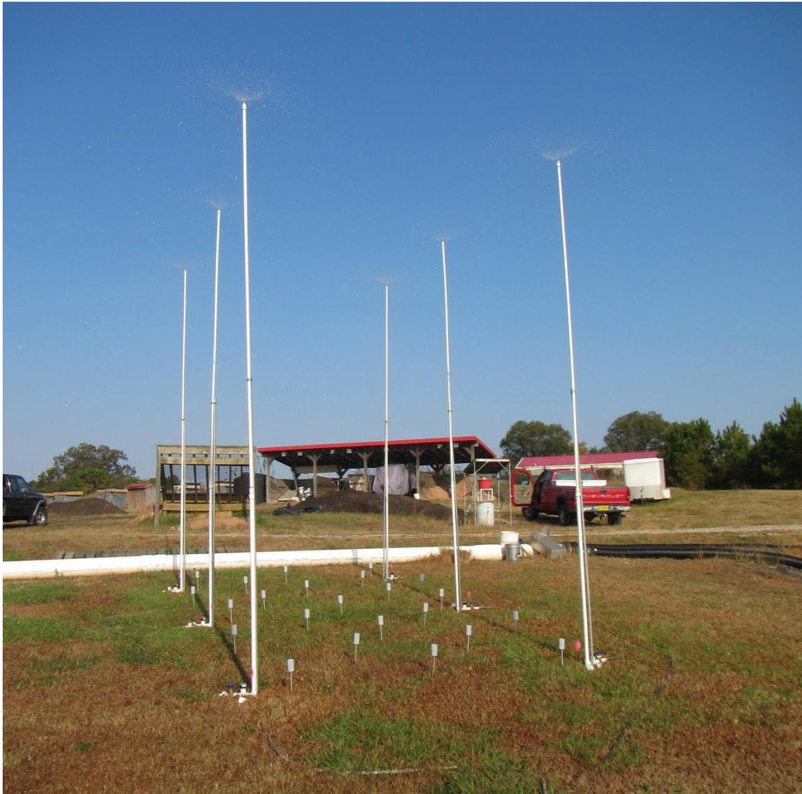
Figure 6. Constructed rainfall simulator in operation at SECREF.
