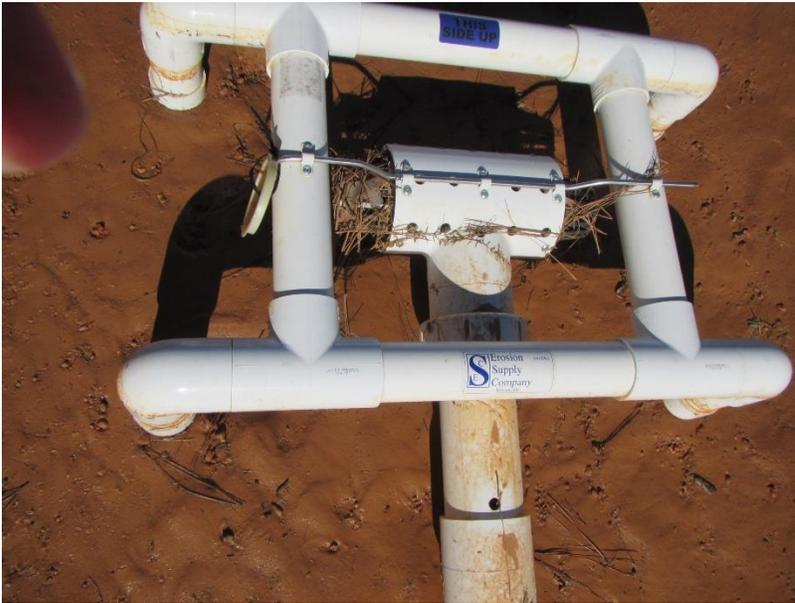
Figure 3. Erosion Supply skimmer.
