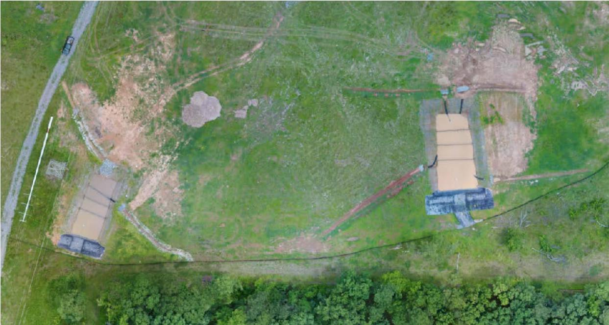
Figure 17. Posi-Shell-lined basin on left and unlined inlet basin on right illustrating potential effects on turbidity.
