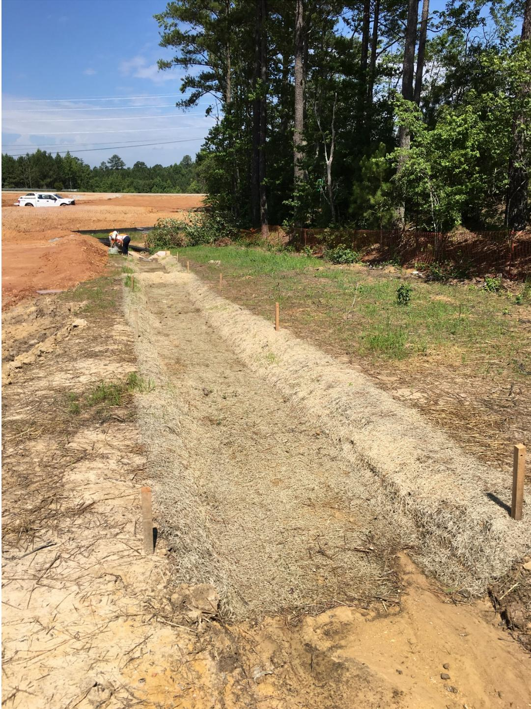
Figure 34. Excelsior-lined ditch in Apex showing the pin stations (stakes) and the V-notch weir at the outlet. Picture was taken July 6, 2016.
