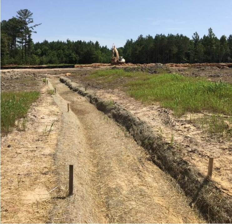
Figure 10. Excelsior-lined ditch at the Apex site after flow was cut off to it during grading. Stakes along each side are level across the ditch so the pin tool could be laid on them to measure changes in the cross-section.
