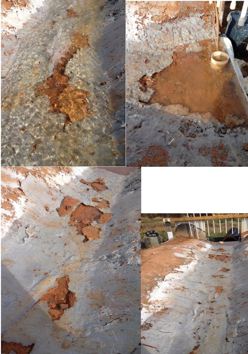
Figure 27. Failures, and resulting erosion, in the hydraulically applied concrete product after poor application to a test ditch.
