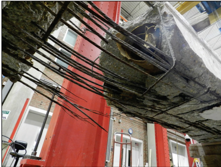
Figure 3.28 – Post-test demolition in laboratory (Oyster Creek – Span 8 – Slab 12)
