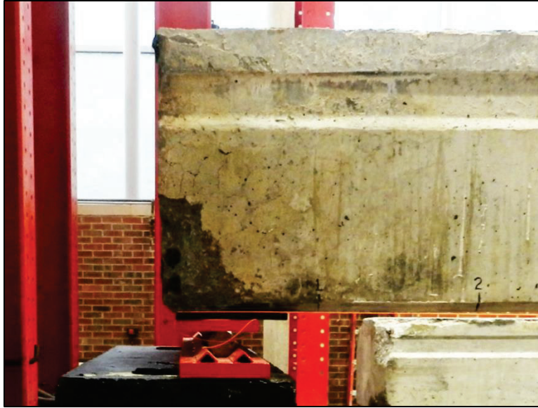
Figure 5.46 - Map-pattern cracking and minor spall at slab end, Oyster Creek - Span 1 - Slab 14
