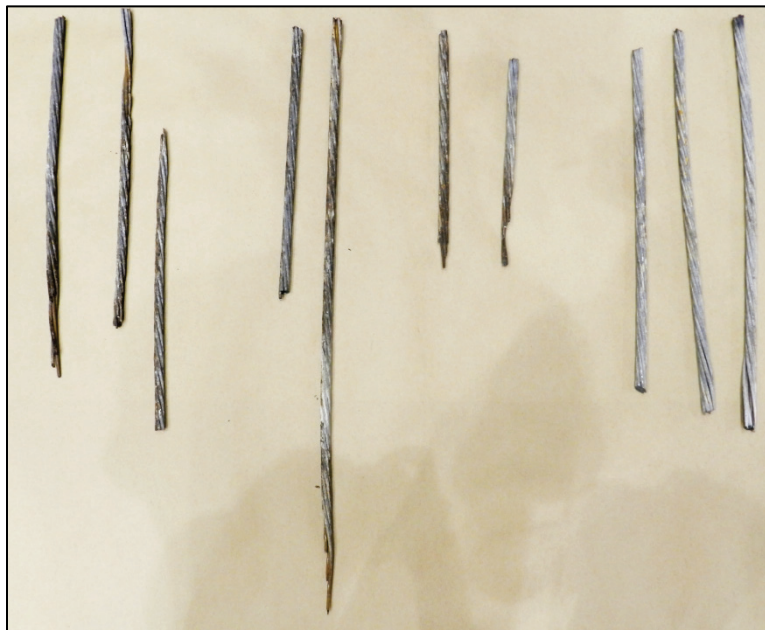
Figure 4.36 - Oyster Creek - Span 1 - Slab 14, bottom layer strands from failed region
