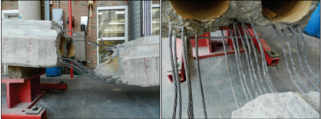
Figure 4.19 - Ward Creek - Span 4 - Slab 5, overview of failed region
