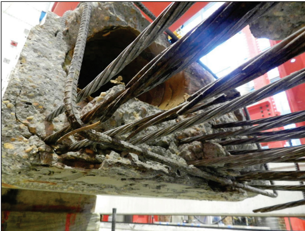
Figure 4.47 - Oyster Creek - Span 8 - Slab 13, moderate rust and pitting of ruptured corner strand
