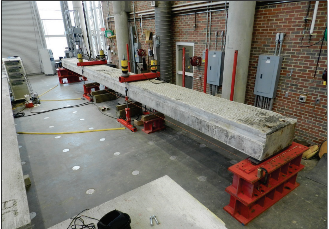
Figure 3.16 – 40 ft slab flexural test setup
