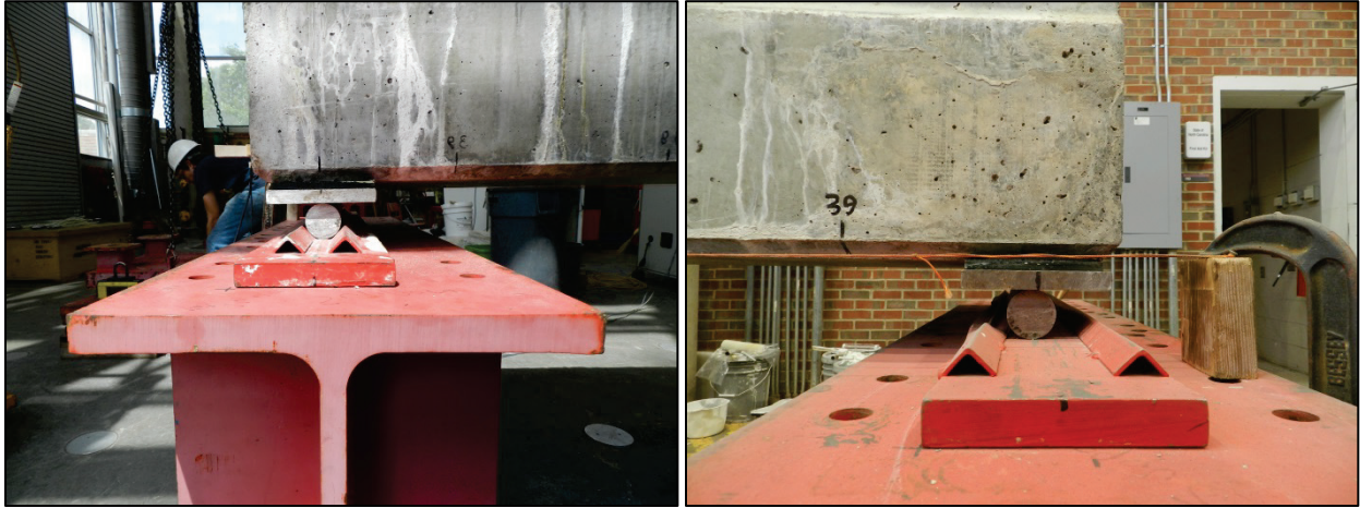
Figure 3.18 – Supports: pin (left), roller (right)
