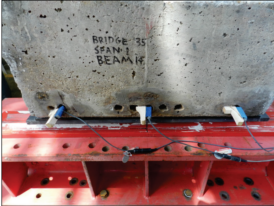
Figure 3.26 - Linear potentiometers at slab end
