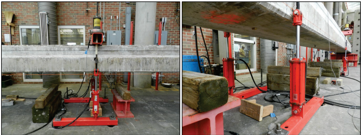
Figure 3.19 – Loading at third points via four 25-kip hydraulic jacks with 10" stroke
