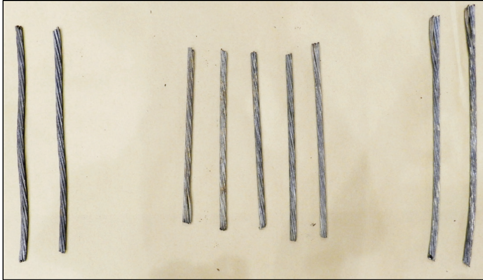
Figure 4.37 - Oyster Creek - Span 1 - Slab 14, second layer strands from failed region
