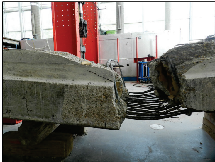
Figure 4.17 - Ward Creek - Span 1 - Slab 14, overview of failed region
