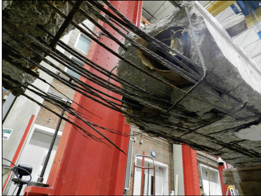
Figure 4.44 - Oyster Creek - Span 8 - Slab 12, soffit after testing, formerly covered by icolastic patch
