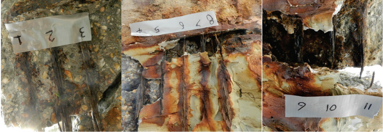
Figure 4.28 - Ward Creek - Span 9 - Slab 7, bottom layer of strands at failure plane after testing
