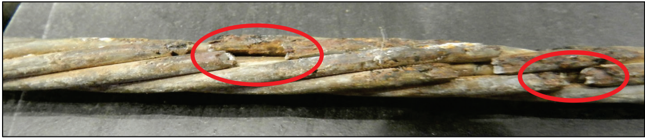
Figure 5.30 – Ruptured wires in strand, Oyster Creek - Span 8 - Slab 13
