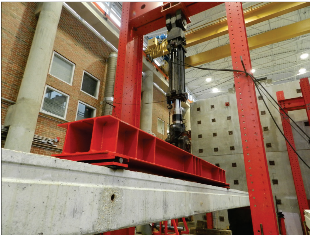
Figure 3.23 - Loading via 220-kip 40 in. stroke actuator with spreader beam
