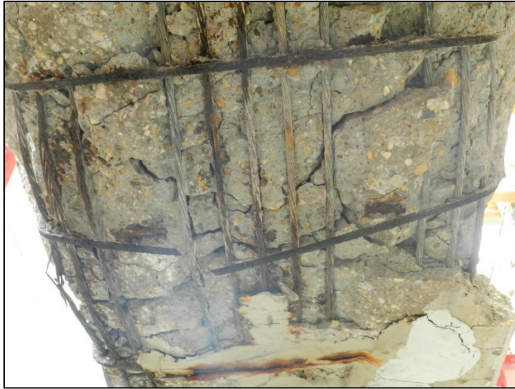
Figure 4.34 - Oyster Creek - Span 1 - Slab 14, slab soffit after failure, showing broken stirrup
