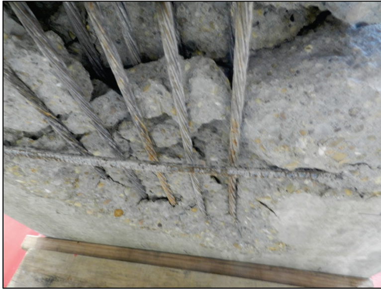
Figure 4.40 - Oyster Creek - Span 2 - Slab 4, central strands at failed region
