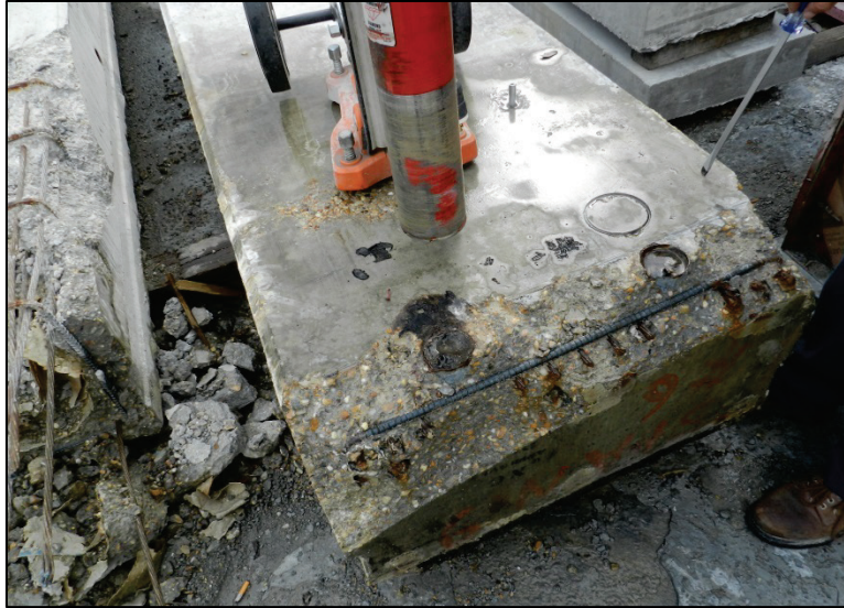
Figure 3.30 - Coring slab end (Ward Creek – Span 9 – Slab 6)
