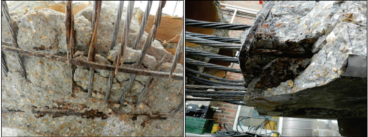
Figure 4.16 - Ward Creek - Span 1 - Slab 14, strands at failed region
