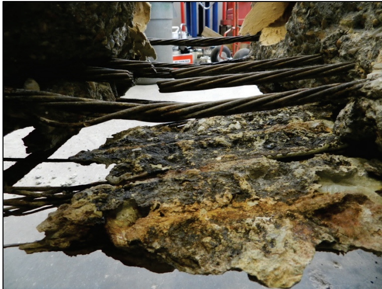
Figure 4.29 - Ward Creek - Span 9 - Slab 7, patching material bonded with strands
