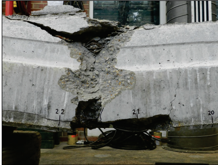
Figure 4.27 - Ward Creek - Span 9 - Slab 7, delamination visible at failed region
