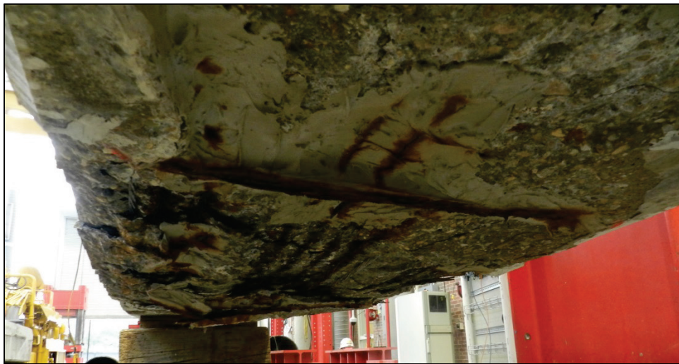
Figure 4.32 - Oyster Creek - Span 1 - Slab 13, slab soffit after failure
