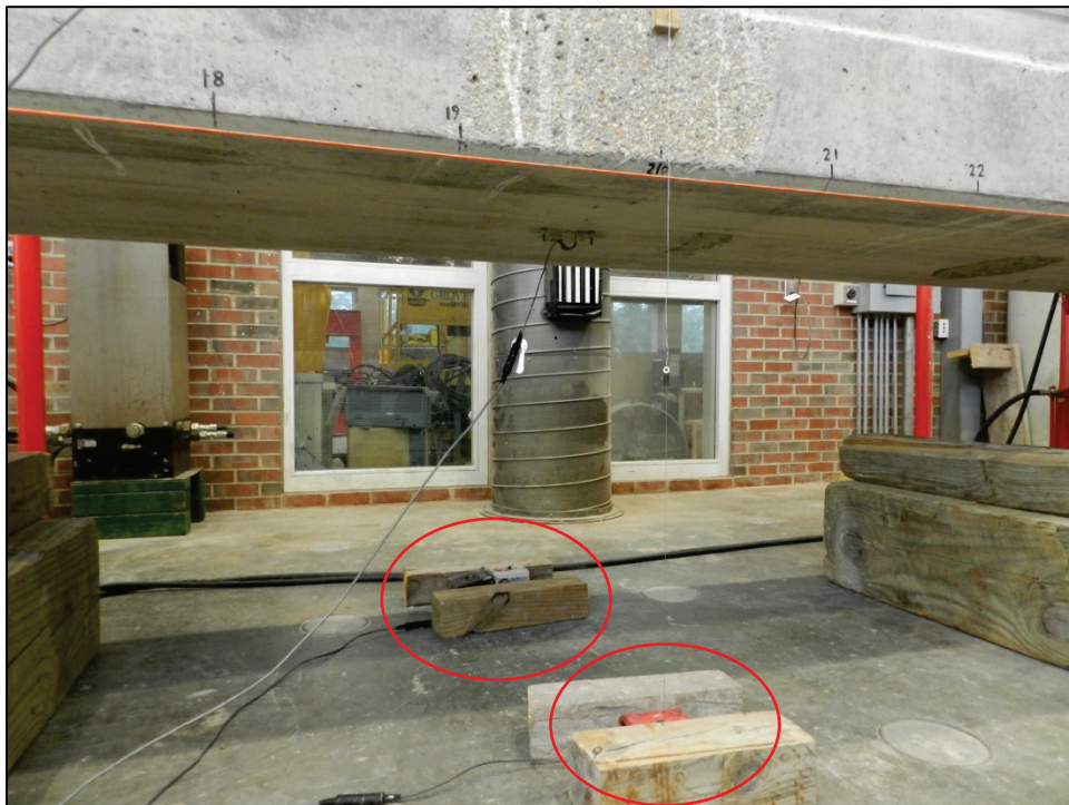
Figure 3.25 – 50 in. string potentiometers at midspan
