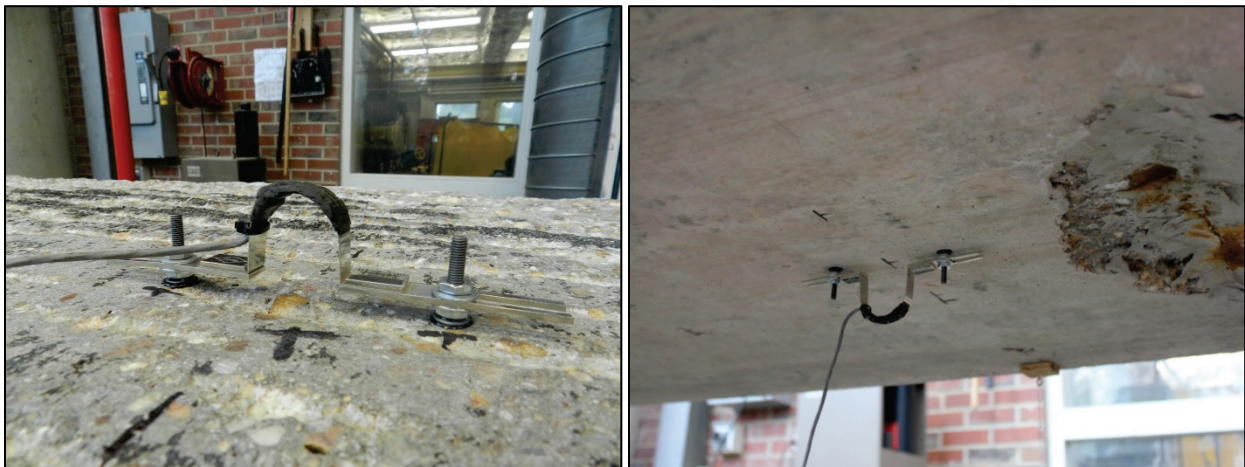
Figure 3.27 - Pi gauges at midspan (top and bottom)
