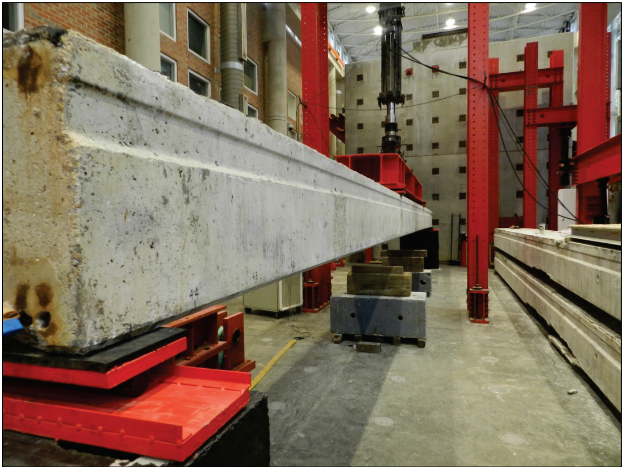
Figure 3.20 - 45-ft slab flexural test setup
