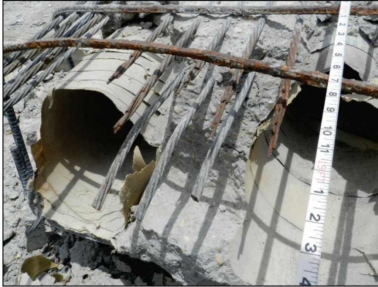
Figure 3.29 - Strands uncovered with jackhammer outside laboratory (Ward Creek – Span 1 – Slab 14)
