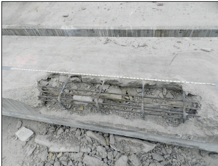
Figure 3.32 – Strands exposed near slab end via jackhammer
