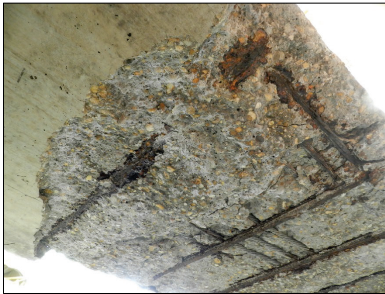
Figure 5.36 - Delaminated region after testing, Ward Creek - Span 1 - Slab 13
