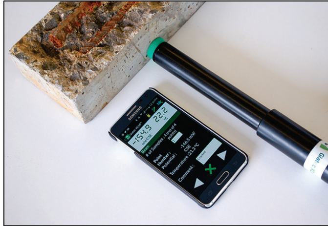
Figure 3.15 - Half-cell potential testing – electrode and software (Giatec Scientific)
