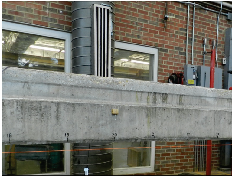
Figure 3.12 – 1 ft intervals marked on side of slab
