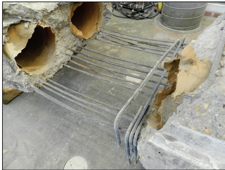
Figure 4.13 - Ward Creek - Span 1 - Slab 13, crushed concrete removed
