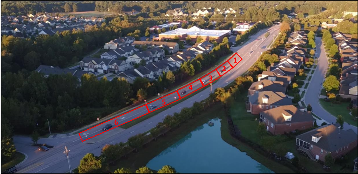
Figure 14 Diagram of merging zones for Ten-Ten Road site
