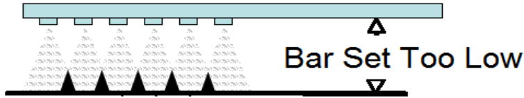
Figure A-6. Streaking resulting from setting the spray bar height too low (Wood et al. 2006).
