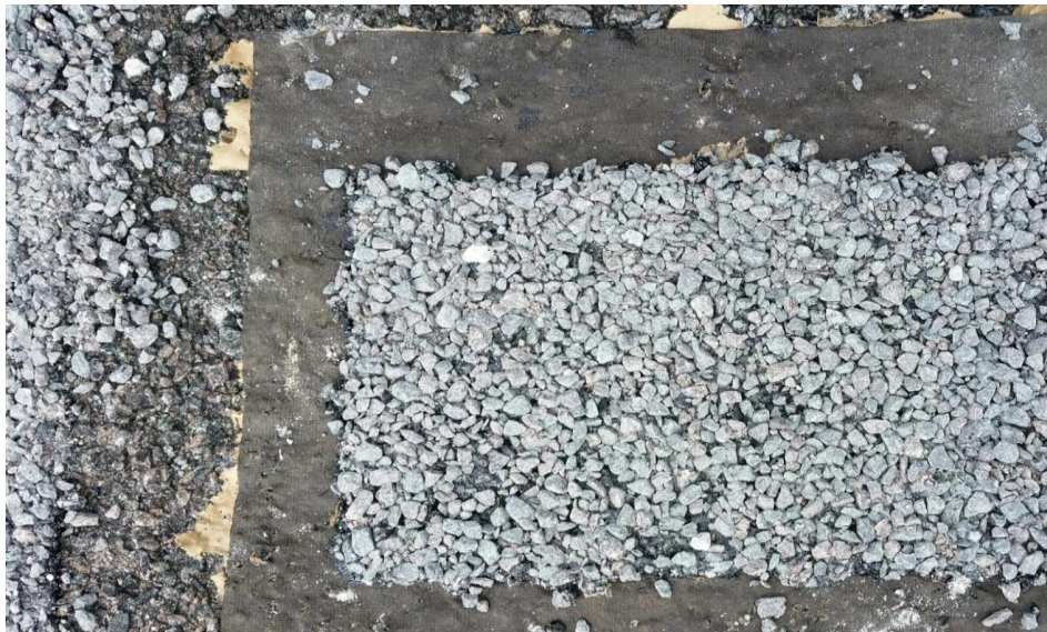
Figure 6. MMLS3 double-seal sample extracted from a chip seal section.
