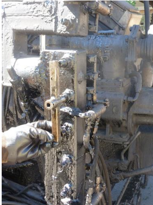
Figure A-4. Adjusting nozzle with nozzle wrench.
