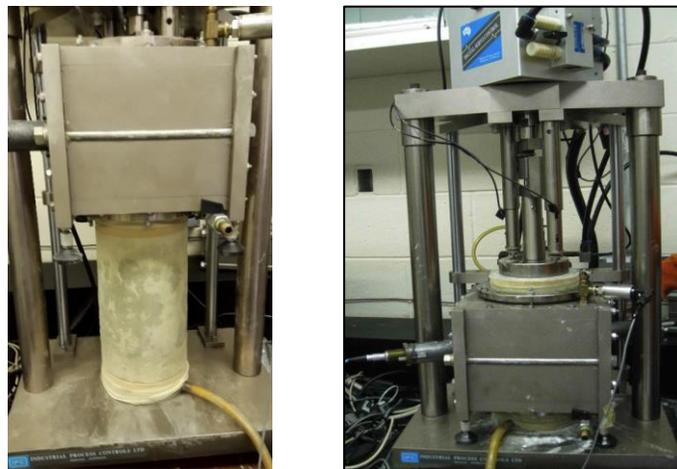
**Figure 3.5** University of Illinois FastCell showing a sample inserted inside the cell (left) and the cell lowered around the sample prior to starting the test (right)
