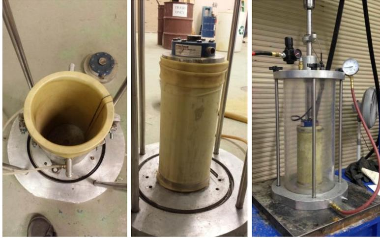
**Figure 3.3** Sample preparation for shear strength test and the TX-12 shear strength setup
