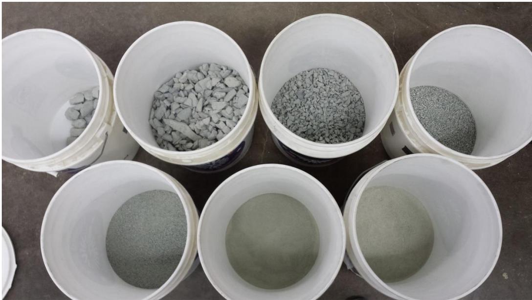
**Figure 3.1** Size separation of each aggregate material batched at the source gradation determined from sieve analysis. From left to right and top to bottom: materials retained on sieve sizes 1.0 in., 0.5 in., No.4, No. 10, No. 40, No. 200 and pan.
