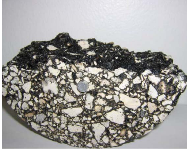
Figure A-12 - The Interstitial Surface on a Broken Sample (Kim 2006)
