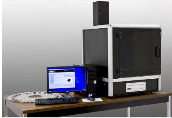
Figure 6 - AIMS2 equipment and set-up (Gates et al. 2011)
