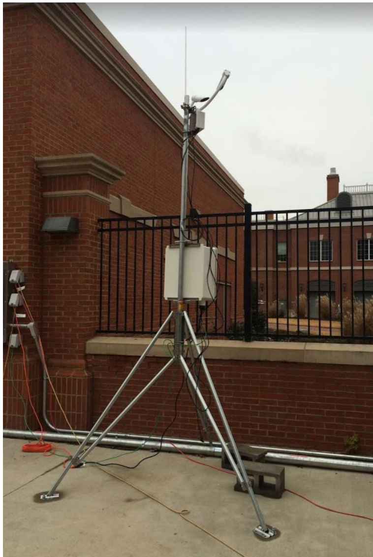
Figure 30 Visibility Sensor (Installed at UNC Charlotte)
