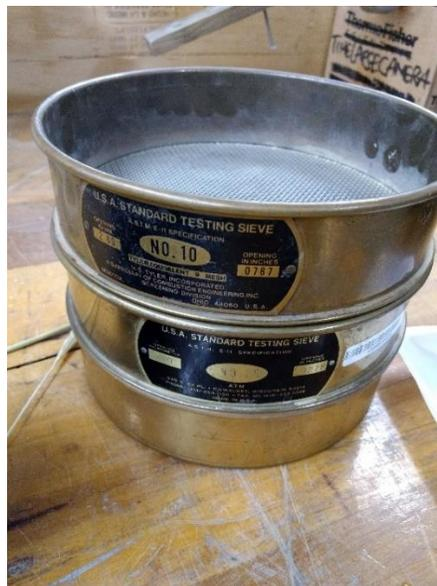
**Figure 7.** Sieve setup to reduce particle size of sediment for runoff simulation
