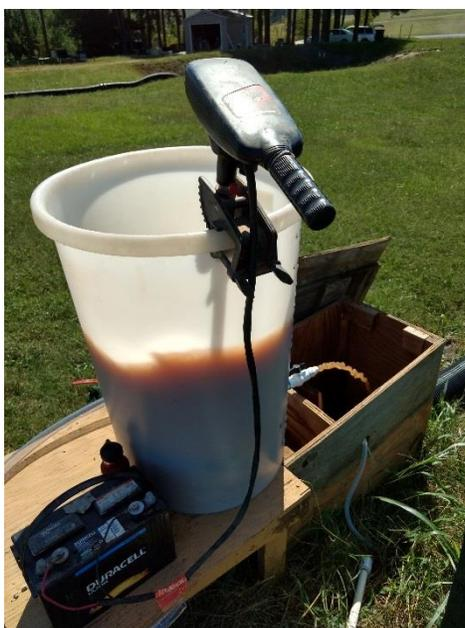
**Figure 8.** Synthetic runoff simulation and monitoring setup at the inlet box
