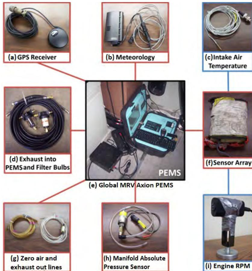
FIGURE 3-1. The GlobalMRV Axion PEMS and components: (a) GPS receiver; (b) Meteorology sensor; (c) Intake Air Temperature Sensor; (d) Exhaust sample lines; (e) Axion PEMS; (f) Engine sensor array; (g) Zero air and exhaust-out lines; (h) Manifold Absolute Pressure sensor; and (i) Engine RPM sensor
