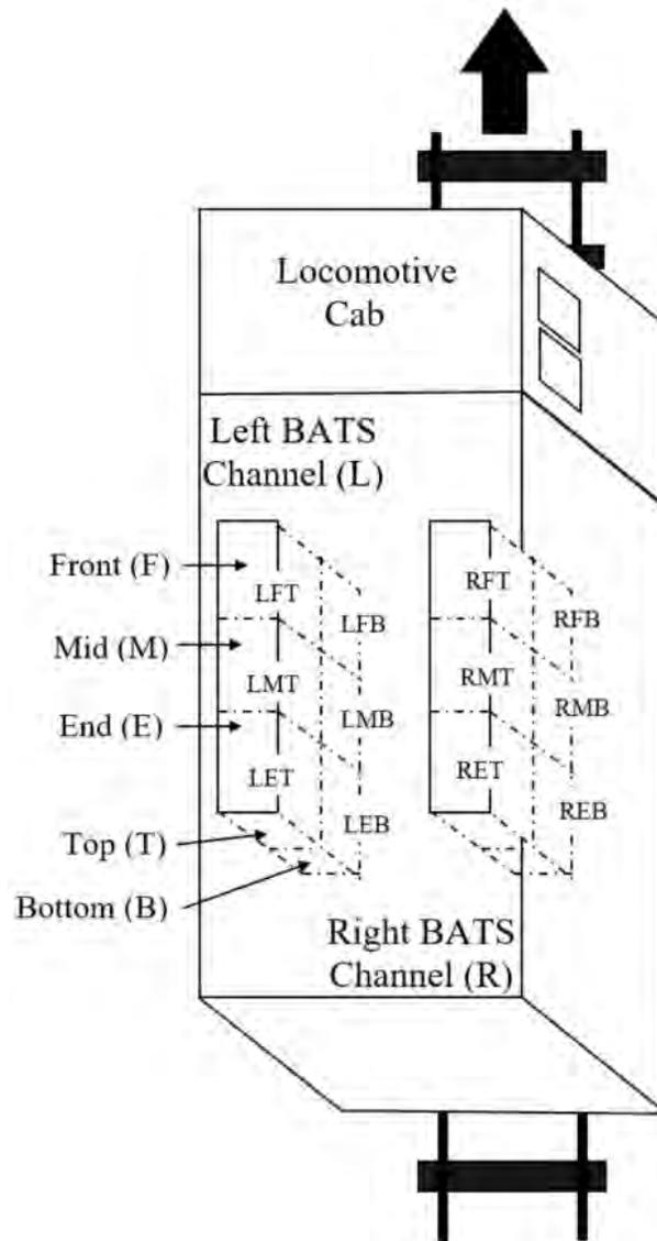
FIGURE D- 4. Sampling Locations for BATS Mapping
