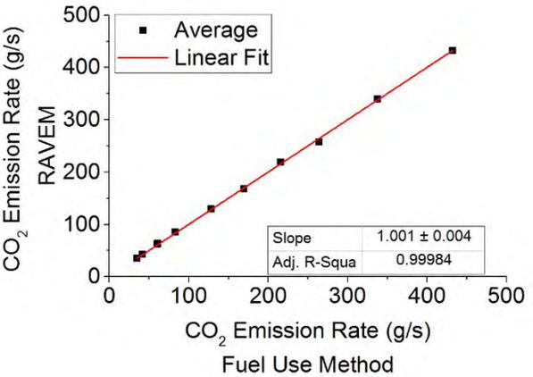
FIGURE C- 2. Comparison of CO<sub>2</sub> emission rates estimated from fuel use method with LEMS estimates at BATS outlet of locomotive NC 1859 running on ULSD
