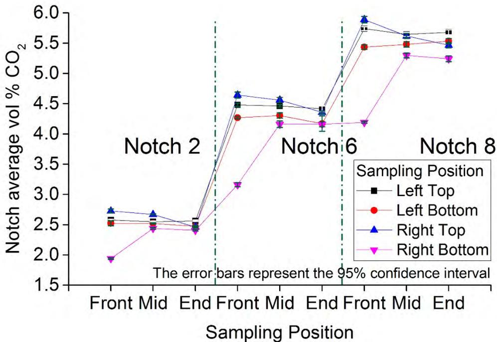
FIGURE D- 5. Variation of CO<sub>2</sub> Concentration with Sampling Location
