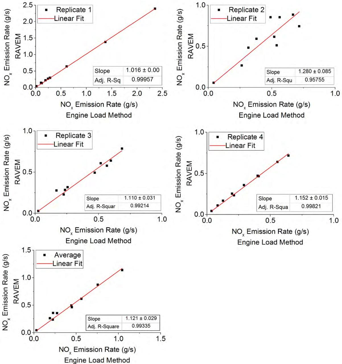
FIGURE C- 3. Comparison of NO<sub>x</sub> emission rates estimated from engine Activity method with LEMS estimates at BATS outlet of locomotive NC 1859 running on ULSD
