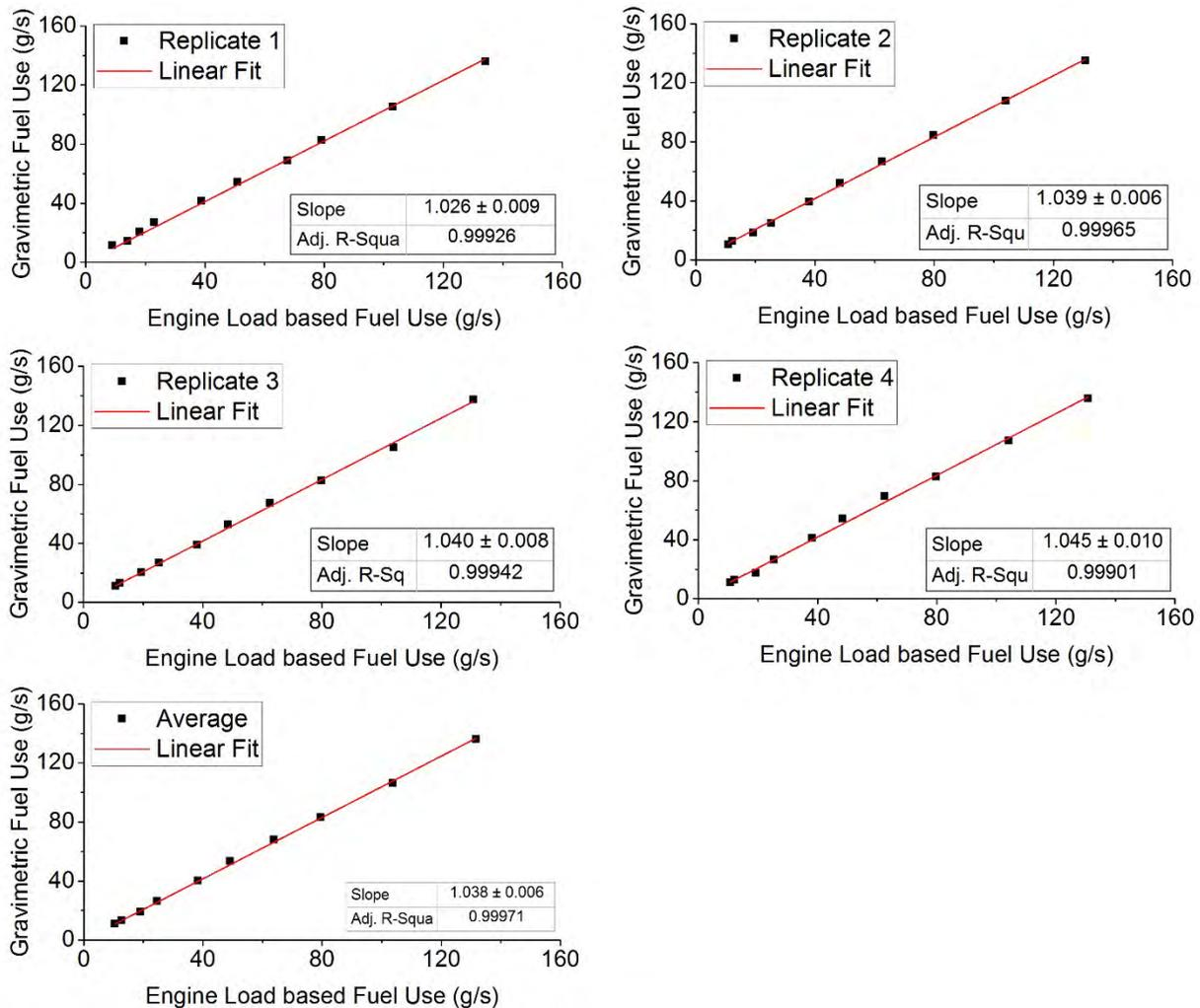
FIGURE 6-4. Comparison between Fuel Use Rate Estimated by BATS Engine Activity Method and Fuel Use Rate Measured Gravimetrically for the Measurements Conducted at BATS Outlet of Locomotive NC1859
