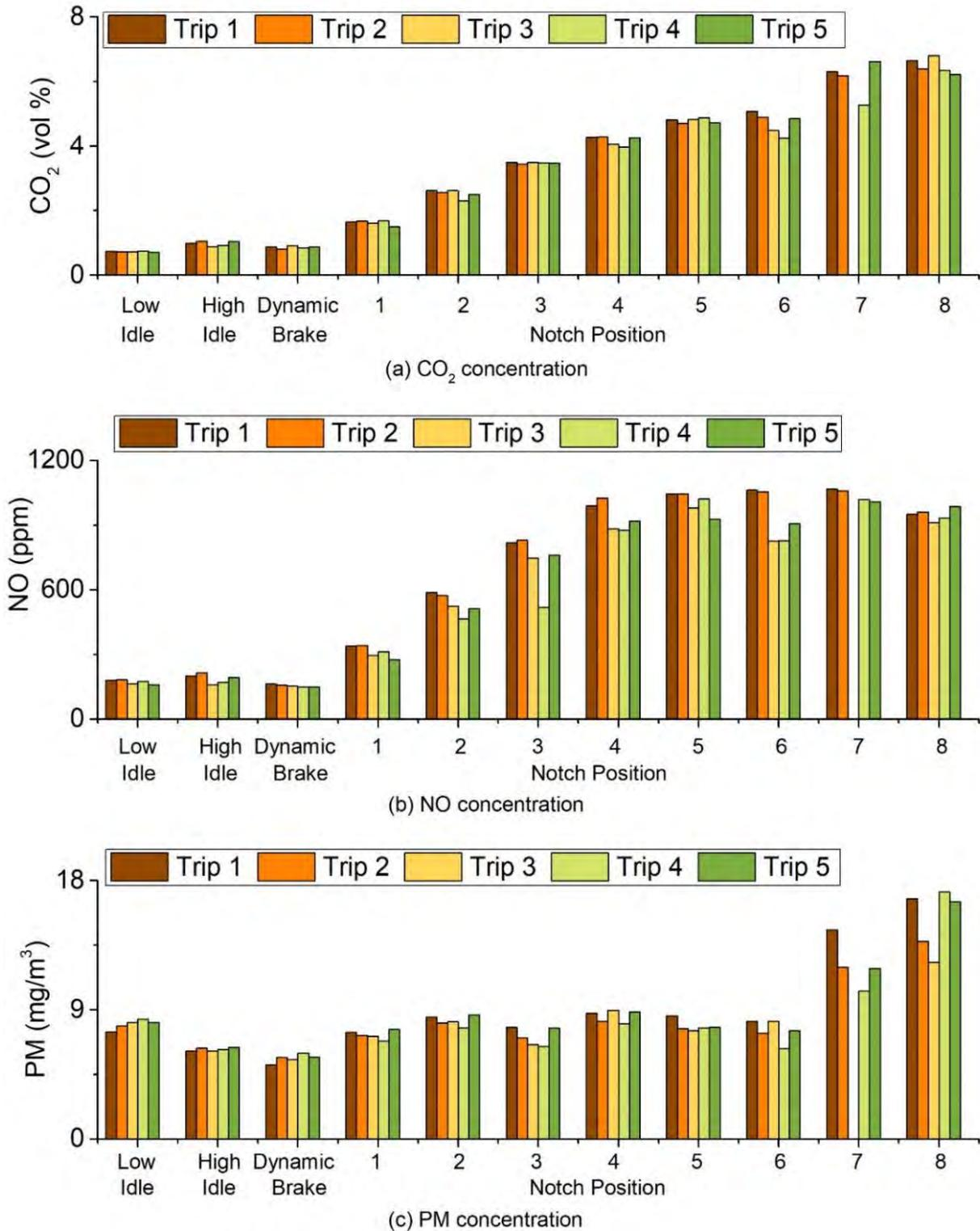
FIGURE 5-1. Measured Notch average Concentrations during Over-the-Rail Measurements on the Prime Mover Engine of NC 1859 Operated on ULSD and connected in Tandem with another locomotive: (a) CO<sub>2</sub> Concentration; (b) NO concentration; and (c) PM Concentration.
