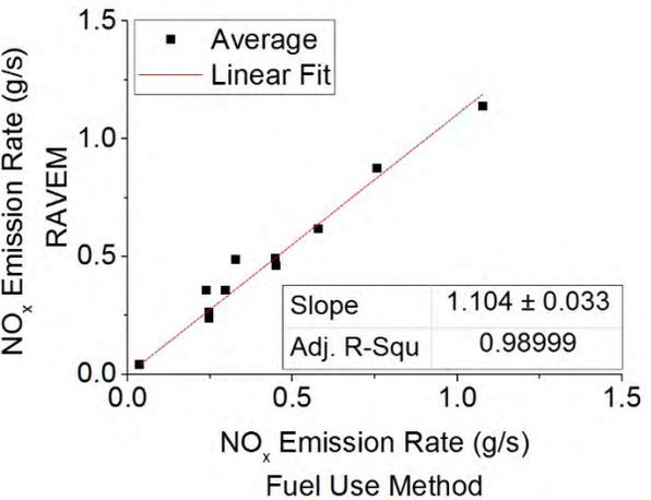
FIGURE C- 4. Comparison of NO<sub>x</sub> emission rates estimated from fuel use method with LEMS estimates at BATS outlet of locomotive NC 1859 running on ULSD
