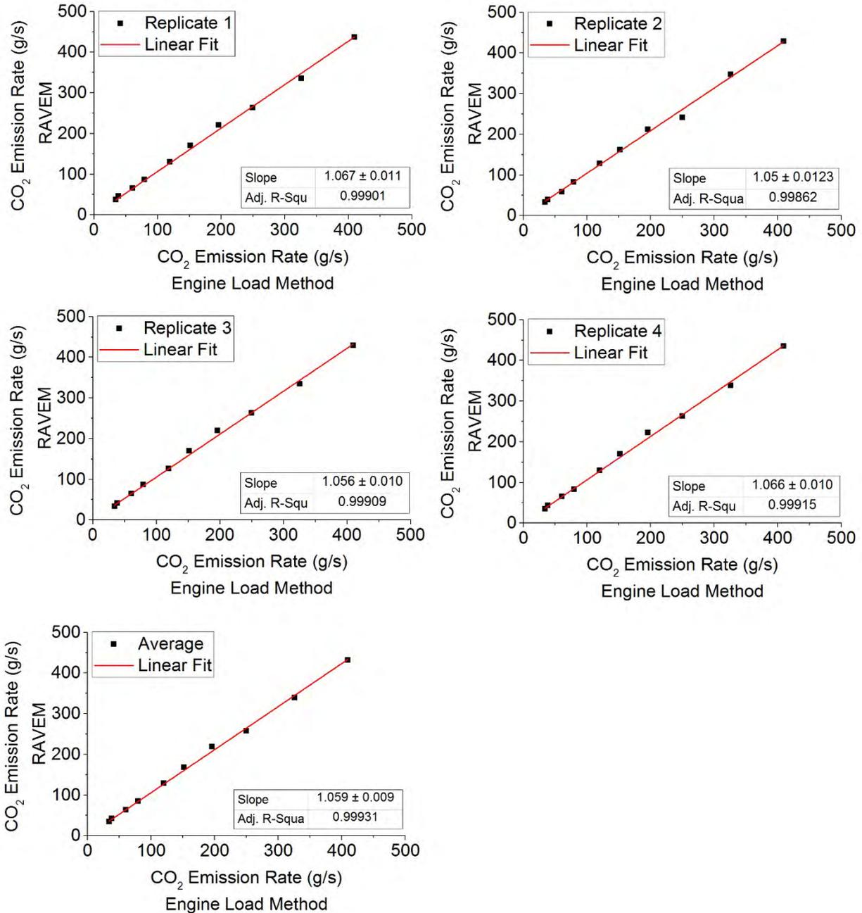
FIGURE C- 1. Comparison of CO<sub>2</sub> emission rates estimated from engine Activity method with LEMS estimates at BATS outlet of locomotive NC 1859 running on ULSD
