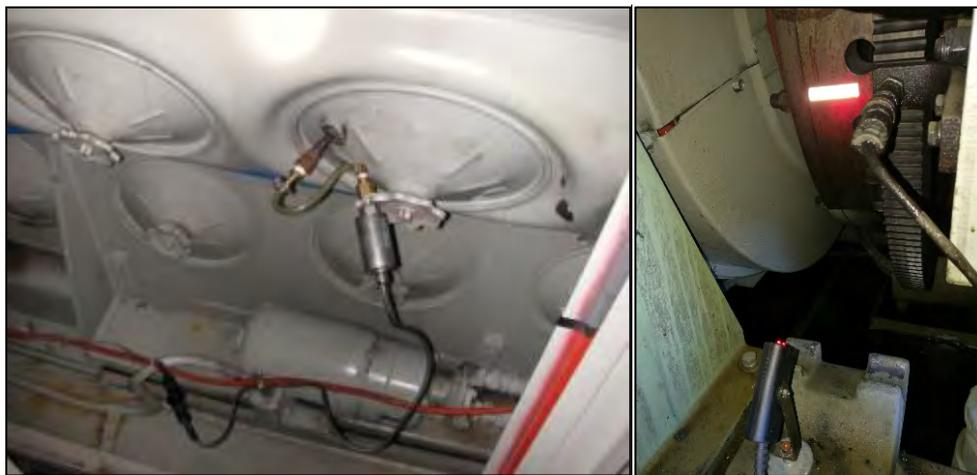
(c) Manifold absolute pressure and temperature sensor (d) Engine RPM sensor
